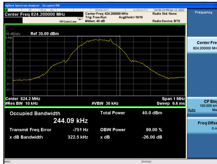
26dB&99% Occupied Bandwidth Plot on Channel 190
