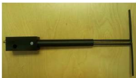
Figure 1 – MVG COMOSAR Validation Dipole
