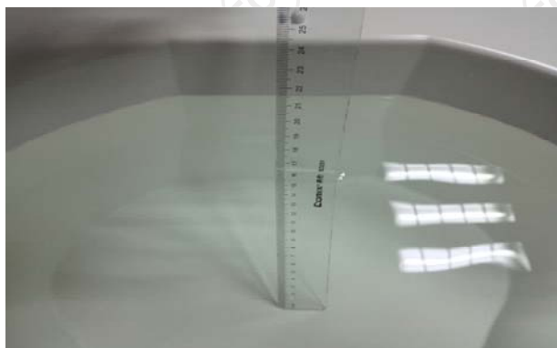
The Body Liquid 2450MHz (16.4cm)
