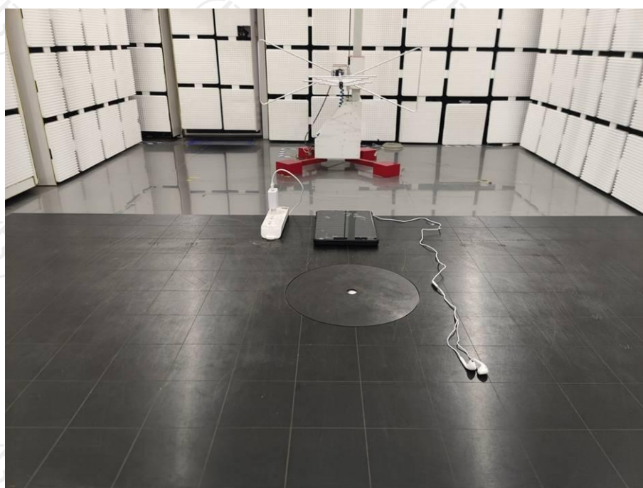
Radiated emission (30 MHz-1 GHz) test view
