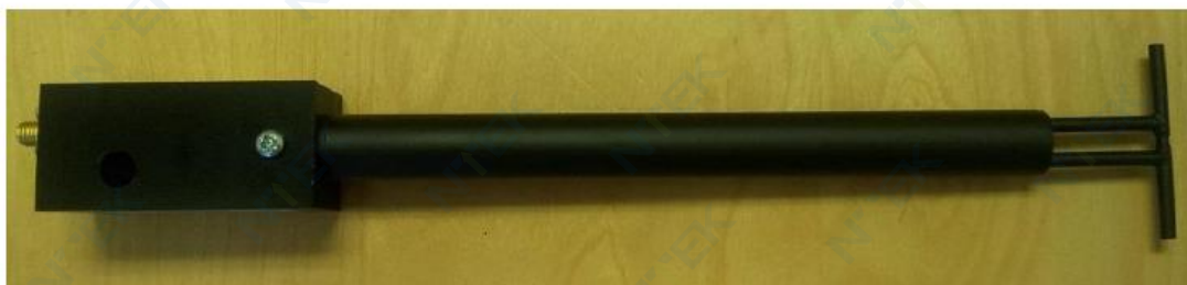
Figure 1 – MVG COMOSAR Validation Dipole
