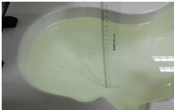
The Head Liquid of 900MHz (15.2cm)
