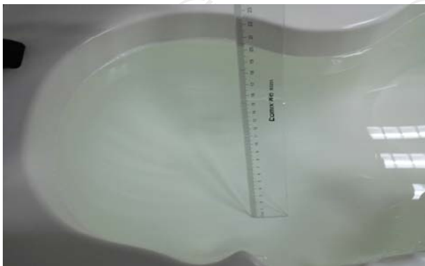
The Head Liquid of 2450MHz (15.7cm)
