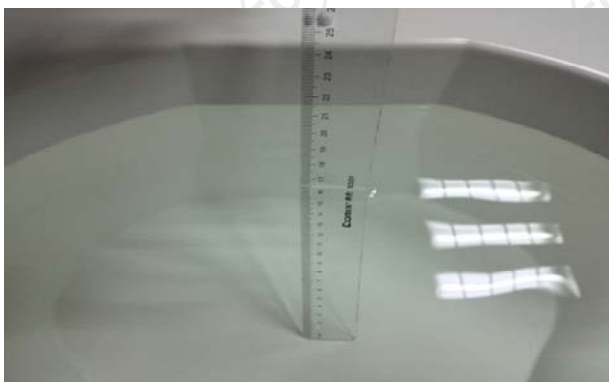
The Body Liquid 2450MHz (16.4cm)
