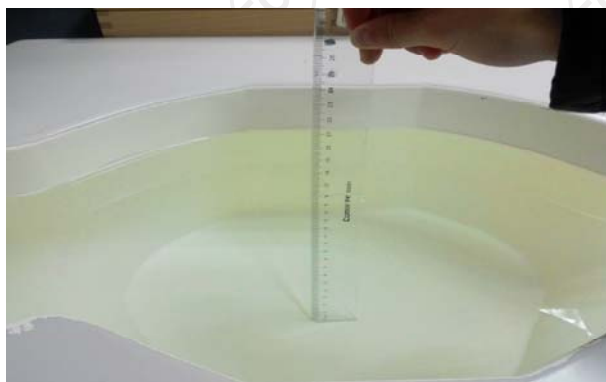
The Body Liquid of 900MHz (15.9 cm)
