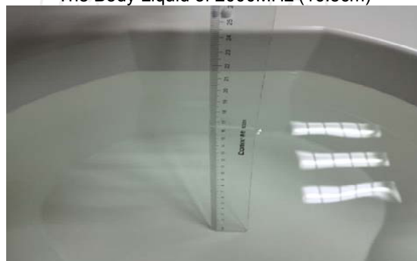
The Body Liquid of 2600MHz (16.6cm)
