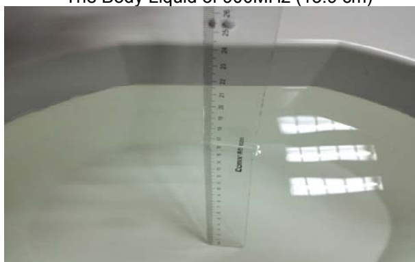
The Body Liquid of 2000MHz (16.5cm)
