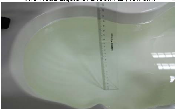
The Head Liquid of 1800MHz (15.6cm)
