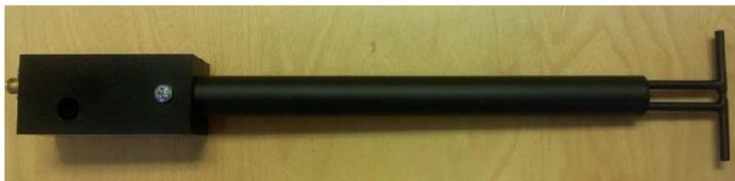
Figure 1 – MVG COMOSAR Validation Dipole
