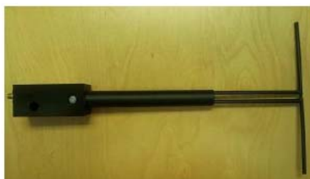
Figure 1 – MVG COMOSAR Validation Dipole
