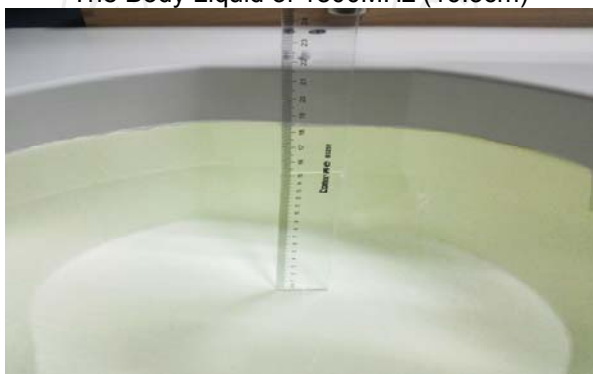
The Body Liquid of 5000-6000MHz (15.2 cm)
