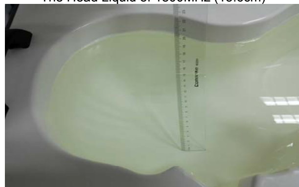
The Head Liquid of 5000-6000MHz (15.3cm)
