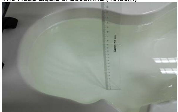
The Head Liquid of 2600MHz (15.1cm)
