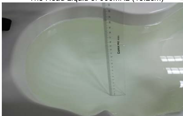
The Head Liquid of 2000MHz (15.5cm)
