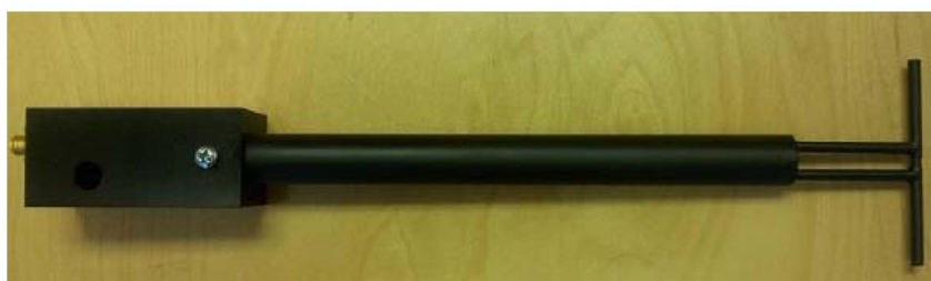
Figure 1 – MVG COMOSAR Validation Dipole
