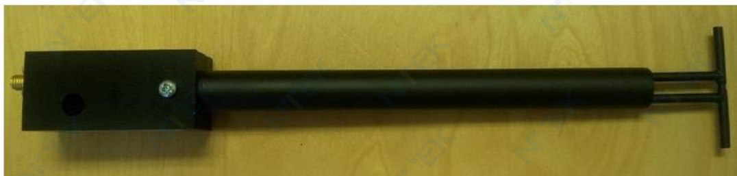
Figure 1 – MVG COMOSAR Validation Dipole
