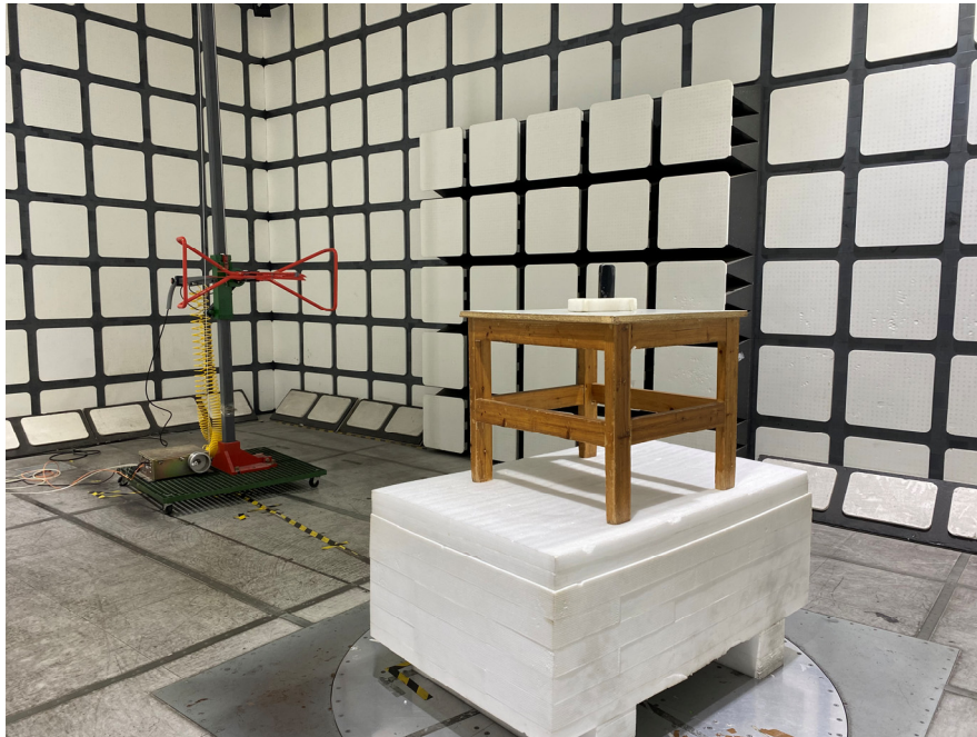
Radiated Spurious Emissions Test View (Below 1GHz)
