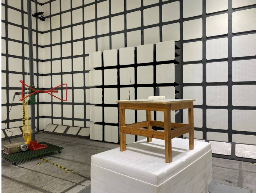
Radiated Spurious Emissions Test View (Above 1GHz)
