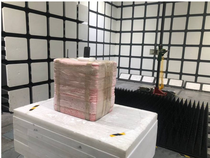
Radiated Spurious Emissions Test View (Above 1GHz)
