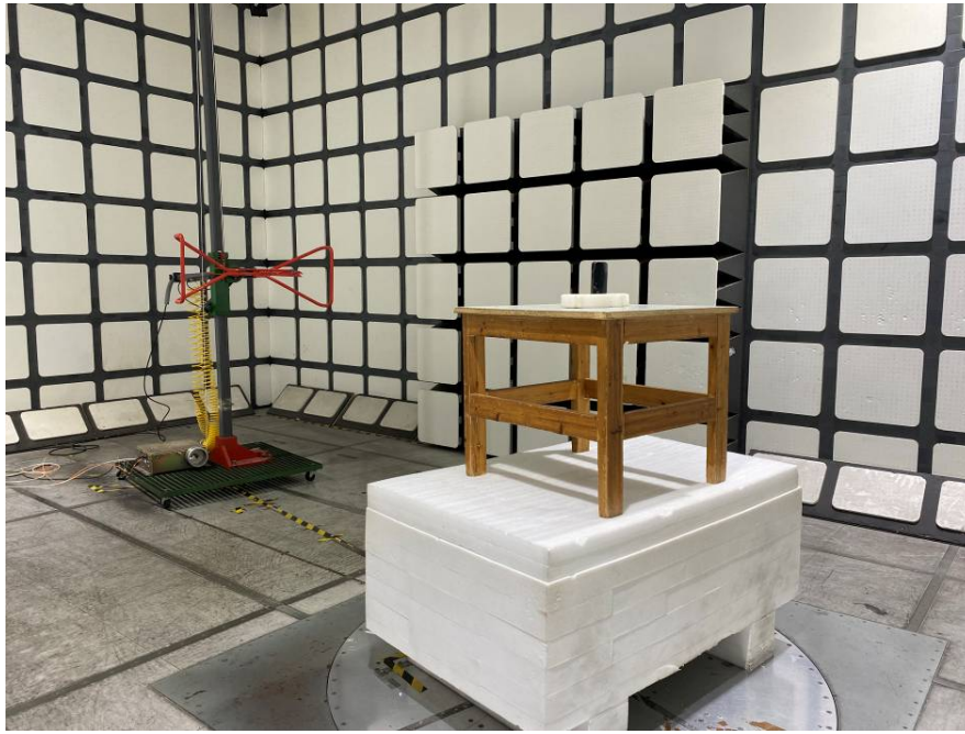
Radiated Spurious Emissions Test View (Above 1GHz)
