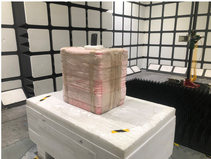
Radiated Spurious Emissions Test View (Above 1GHz)
