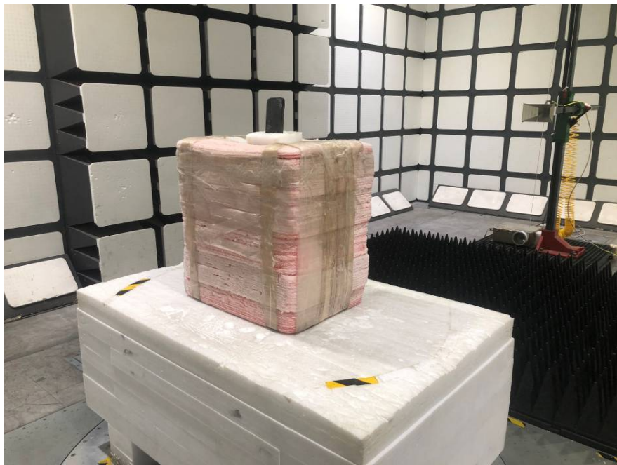
Radiated Spurious Emissions Test View (Above 1GHz)
