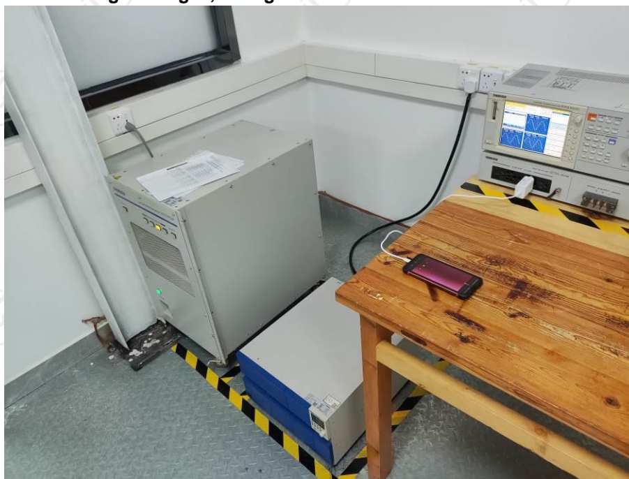
Voltage changes, voltage fluctuations and flicker test view
