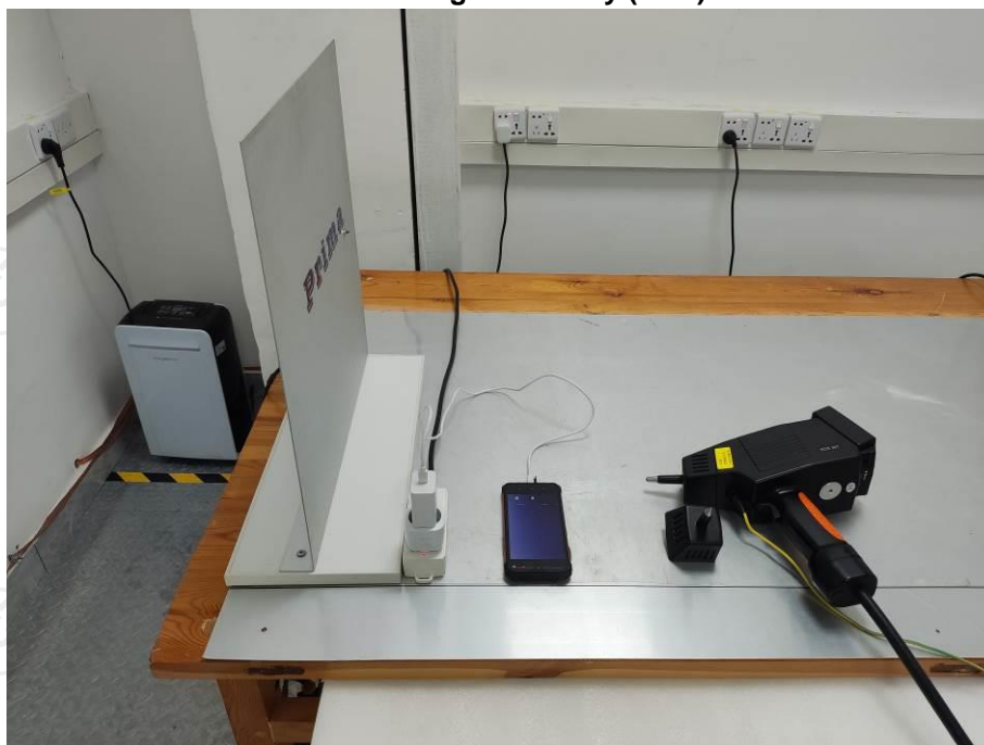
Electrostatic discharge immunity (ESD) test view
