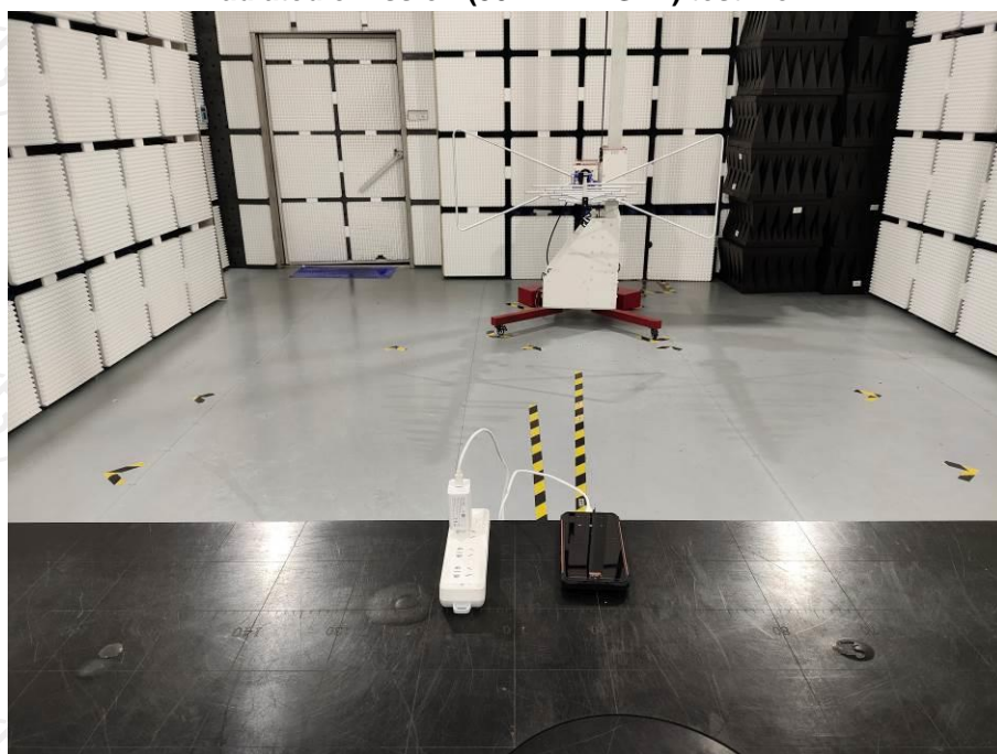
Radiated emission (30 MHz-1 GHz) test view
