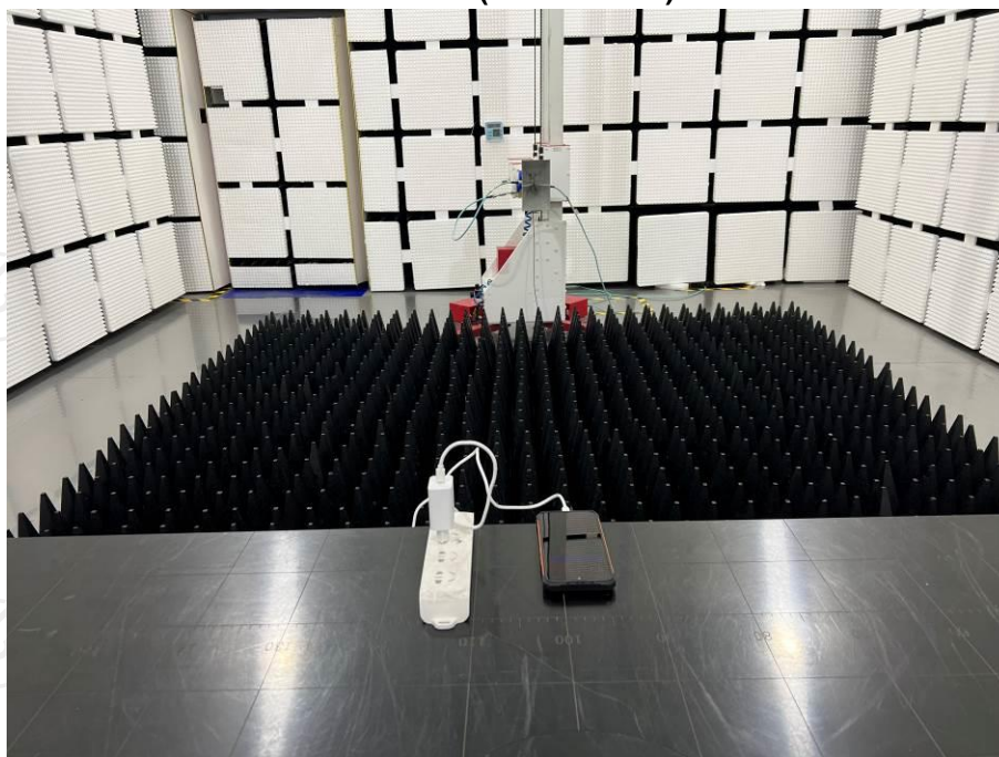
Radiated emission (1 GHz-6 GHz) test view
