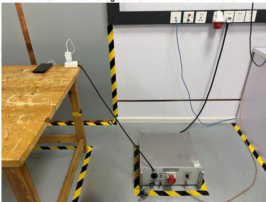
Disturbance voltage at mains terminals test view
