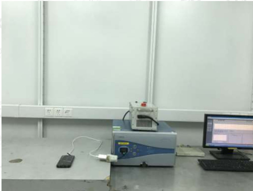
EFT SURGE and DIPS IMMUNITY TEST SETUP
