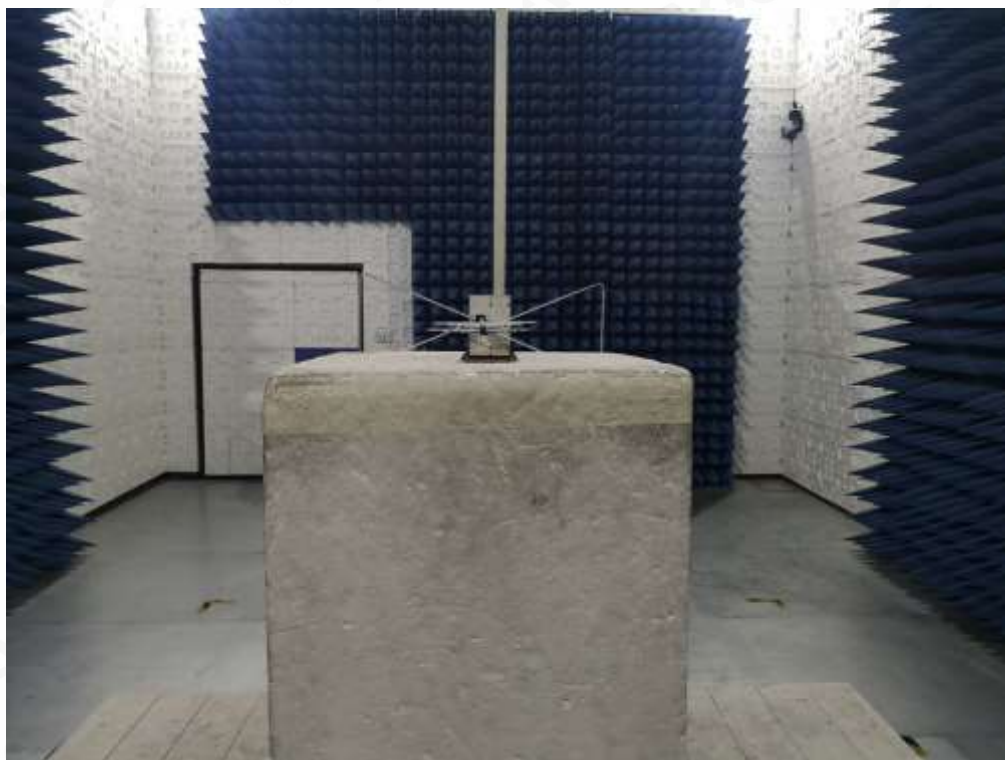
RADIATED SPURIOUS EMISSION ABOVE 1G TEST SETUP
