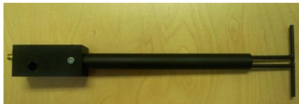
Figure 1 – MVG COMOSAR Validation Dipole
