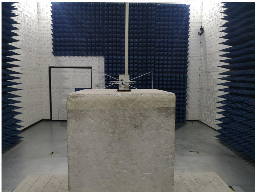
RADIATED SPURIOUS EMISSION-ABOVE 1G TEST SETUP
