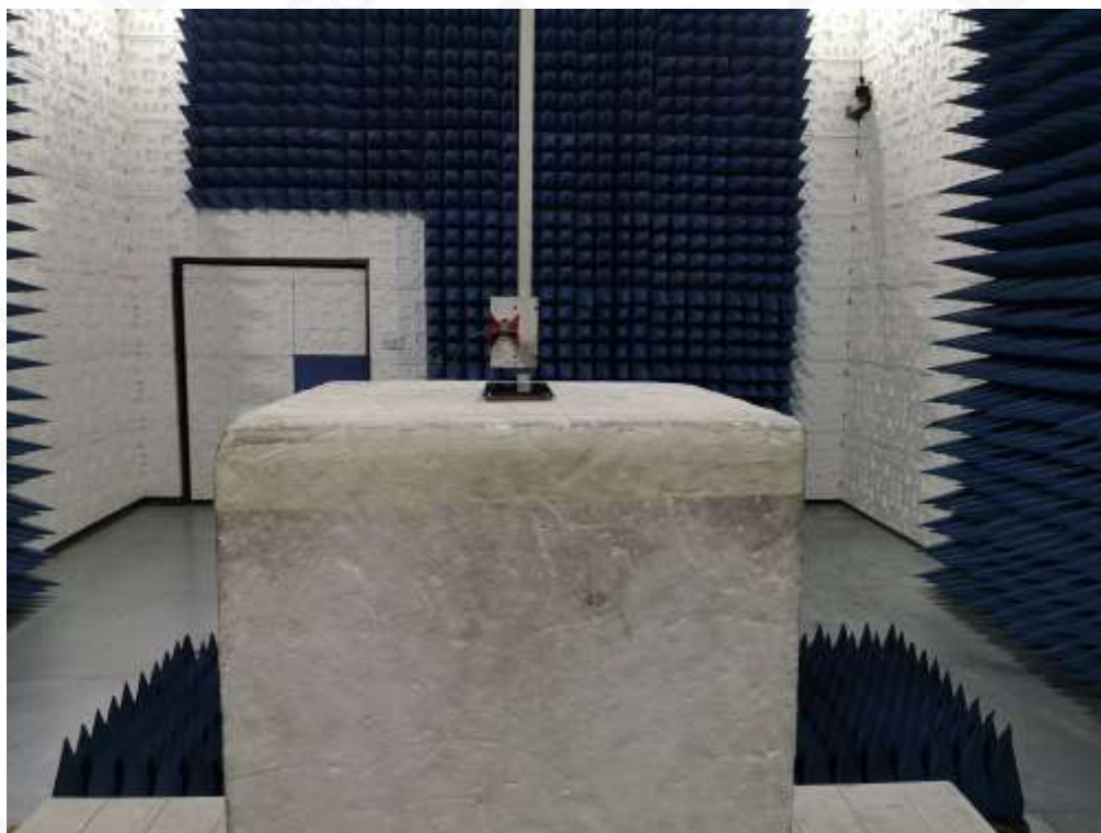
RADIATED SPURIOUS EMISSION ABOVE 1G TEST SETUP
