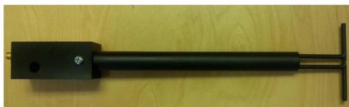
Figure 1 – MVG COMOSAR Validation Dipole
