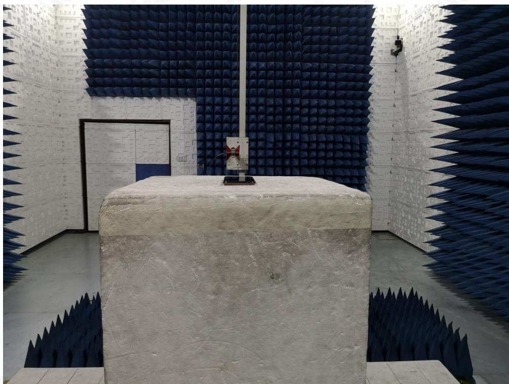
RADIATED SPURIOUS EMISSION-ABOVE 1G TEST SETUP
