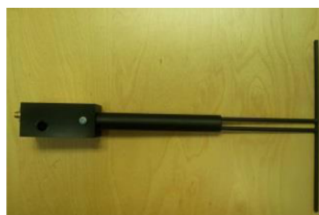
Figure 1 – MVG COMOSAR Validation Dipole
