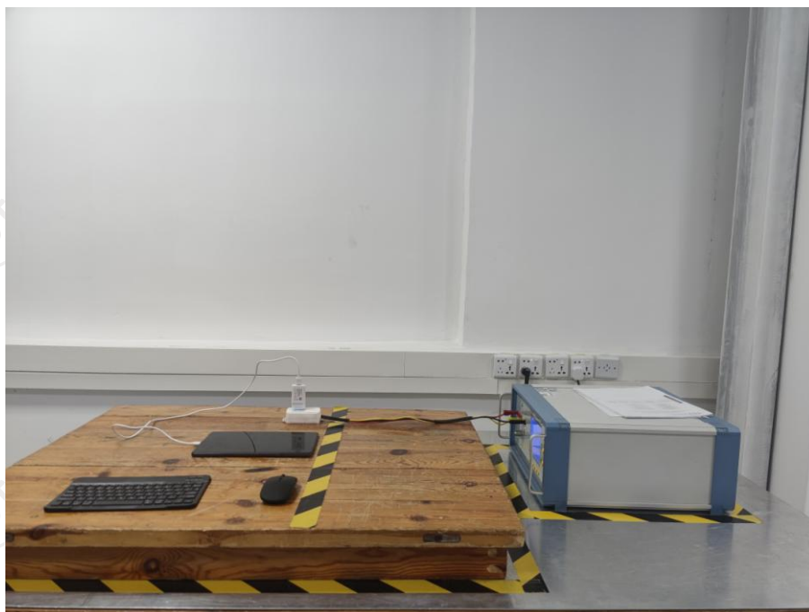
Electrical fast transient/burst immunity (EFT/B) test view
