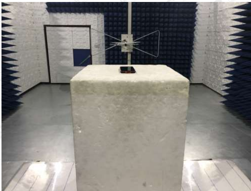
RADIATED SPURIOUS EMISSION_ABOVE 1G TEST SETUP
