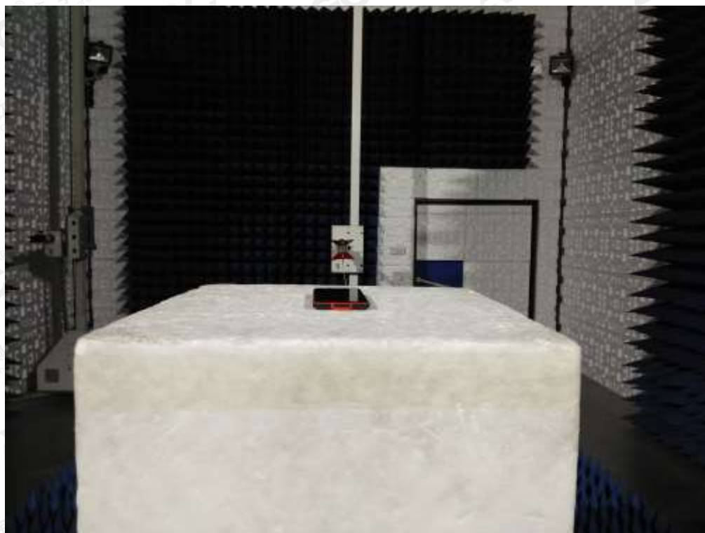
RADIATED SPURIOUS EMISSION_ABOVE 1G TEST SETUP
