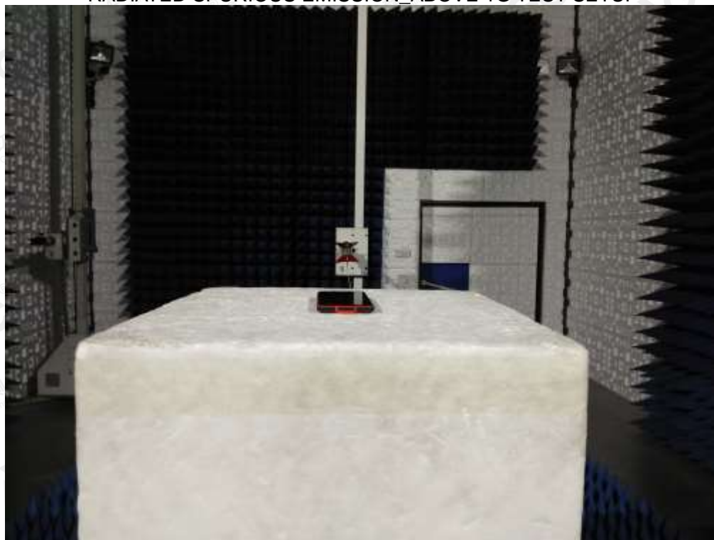
RADIATED SPURIOUS EMISSION_ABOVE 1G TEST SETUP
