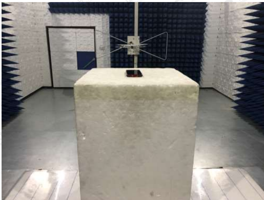
RADIATED SPURIOUS EMISSION_ABOVE 1G TEST SETUP
