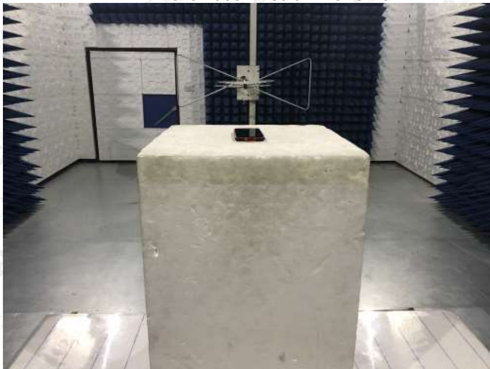
RADIATED SPURIOUS EMISSION_ABOVE 1G TEST SETUP
