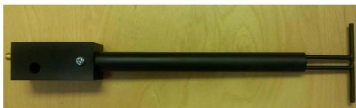
Figure 1 – MVG COMOSAR Validation Dipole
