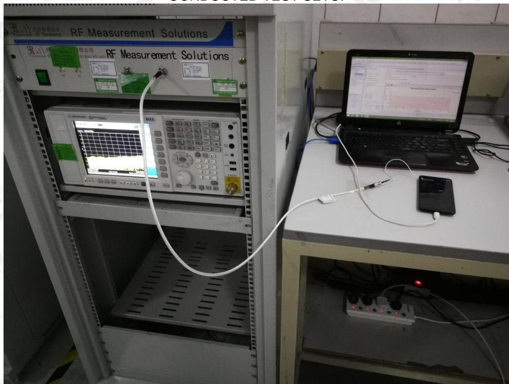
CONDUCTED TEST SETUP
