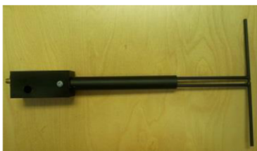
Figure 1 – MVG COMOSAR Validation Dipole
