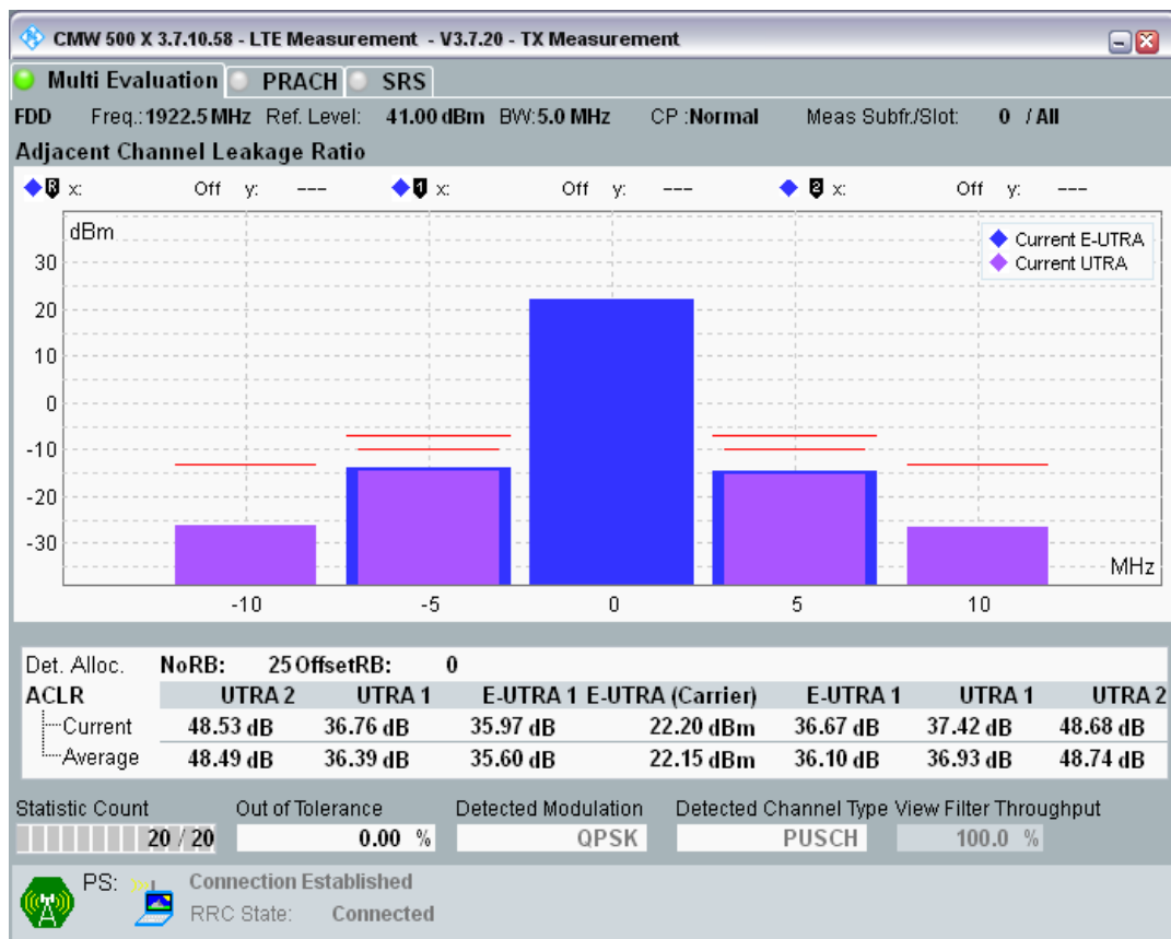
Band1 QPSK BW=5MHz Channel=18025 RB Size=8 Position=#0.png
