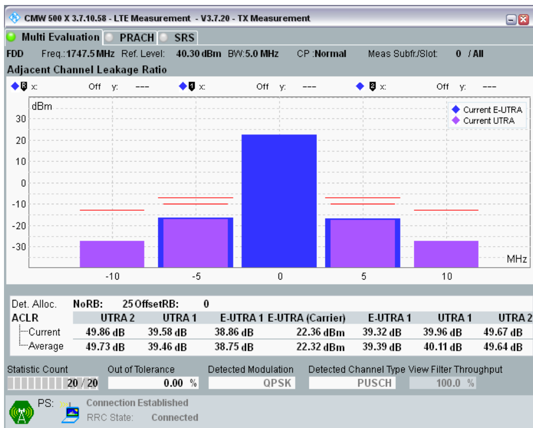
Band3 QPSK BW=5MHz Channel=19575 RB Size=8 Position=#0.png
