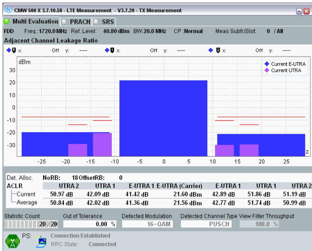
Band3 QAM16 BW=20MHz Channel=19300 RB Size=18 Position=#Max.png
