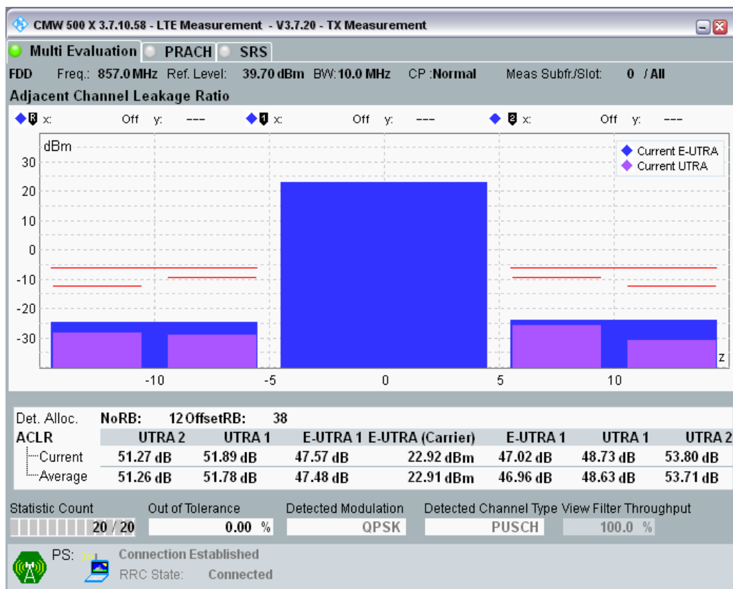
Band20 QPSK BW=10MHz Channel=24400 RB Size=50 Position=#0.png
