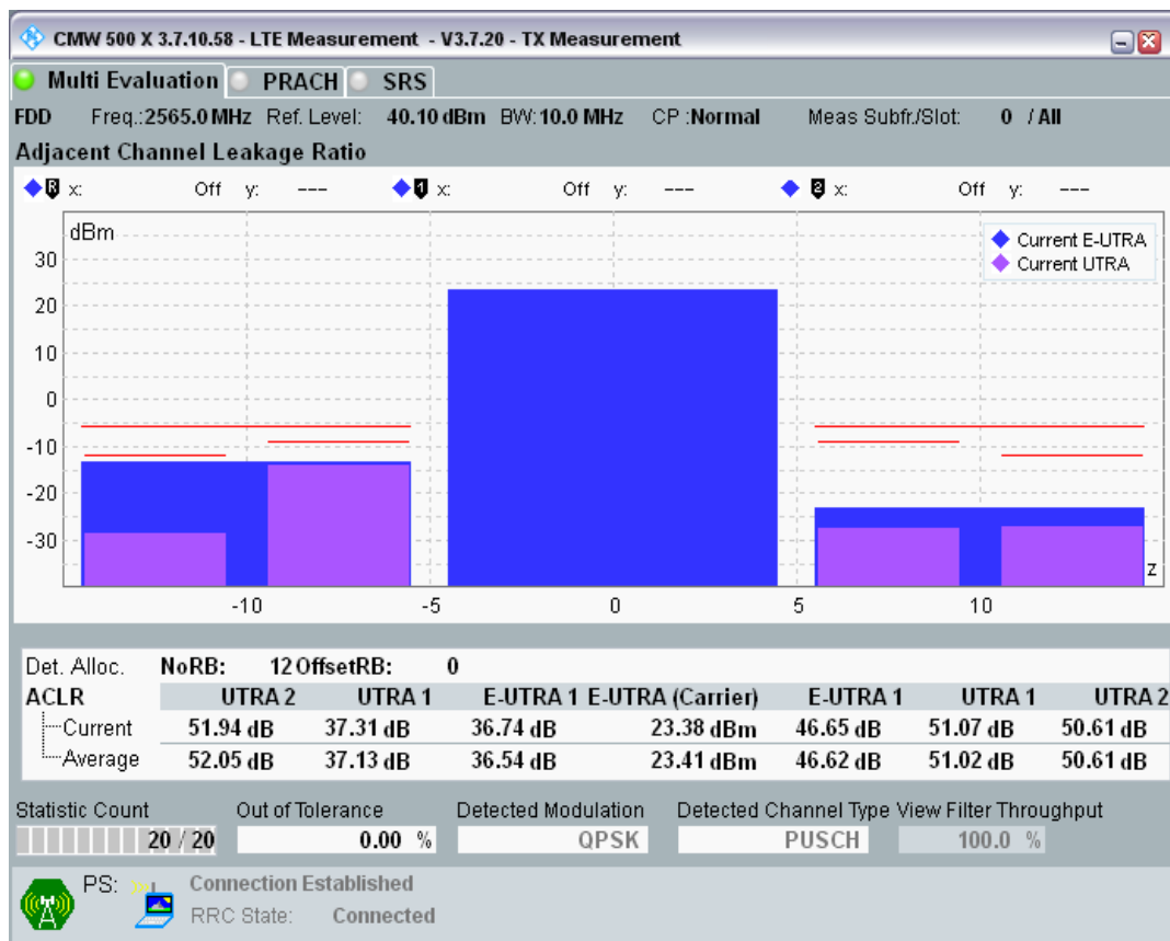
Band7 QPSK BW=10MHz Channel=21400 RB Size=12 Position=#Max.png
