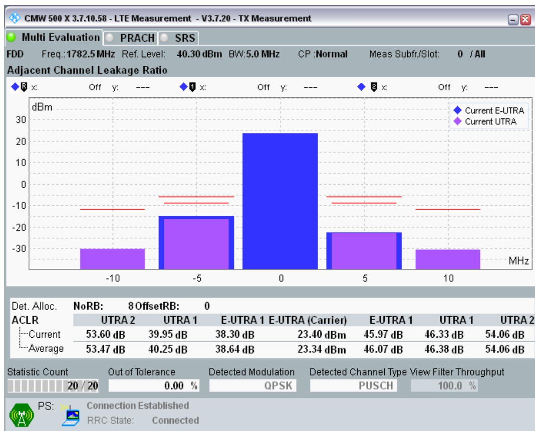
Band3 QPSK BW=5MHz Channel=19925 RB Size=8 Position=#Max.png
