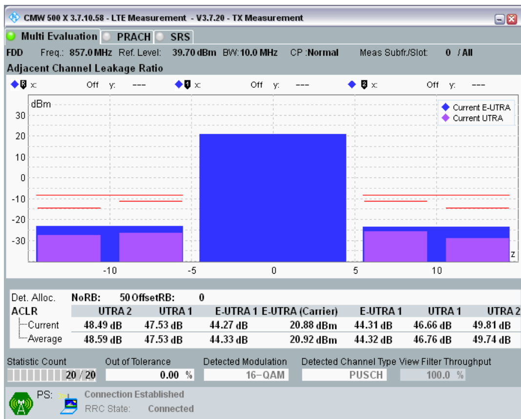
Band20 QAM16 BW=20MHz Channel=24250 RB Size=100 Position=#0.png
