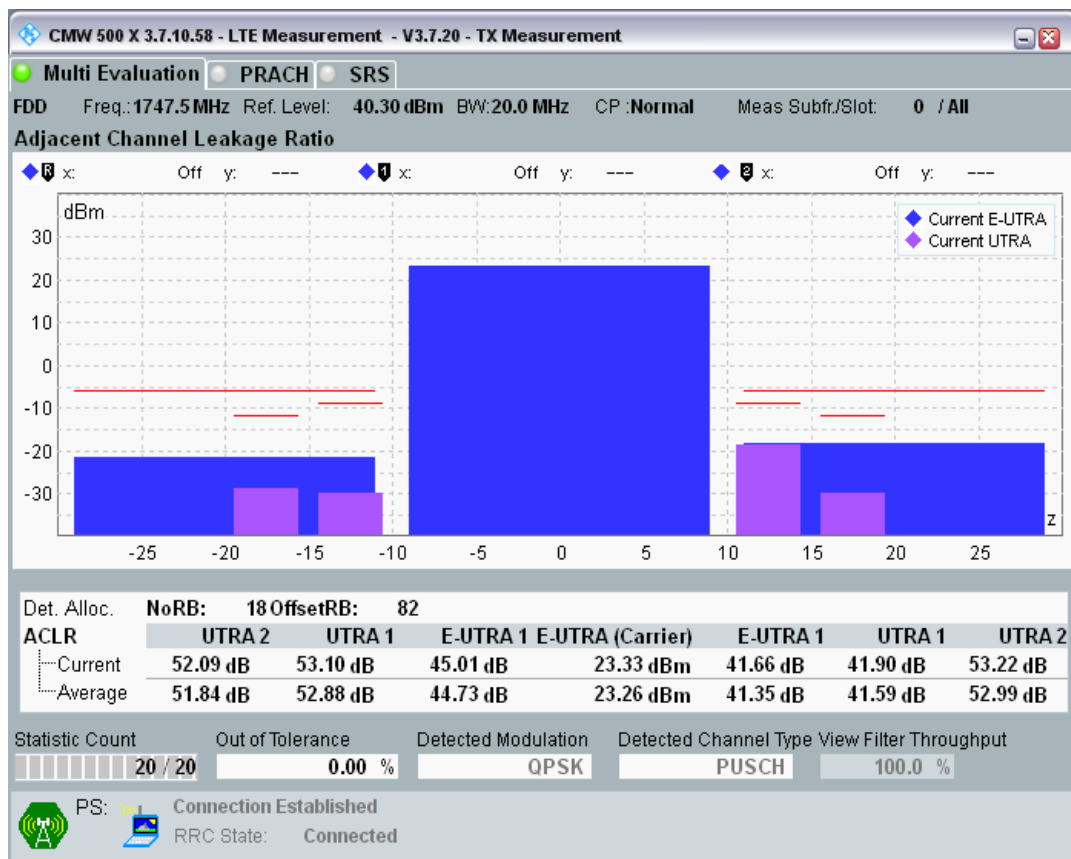
Band3 QPSK BW=20MHz Channel=19850 RB Size=100 Position=#0.png
