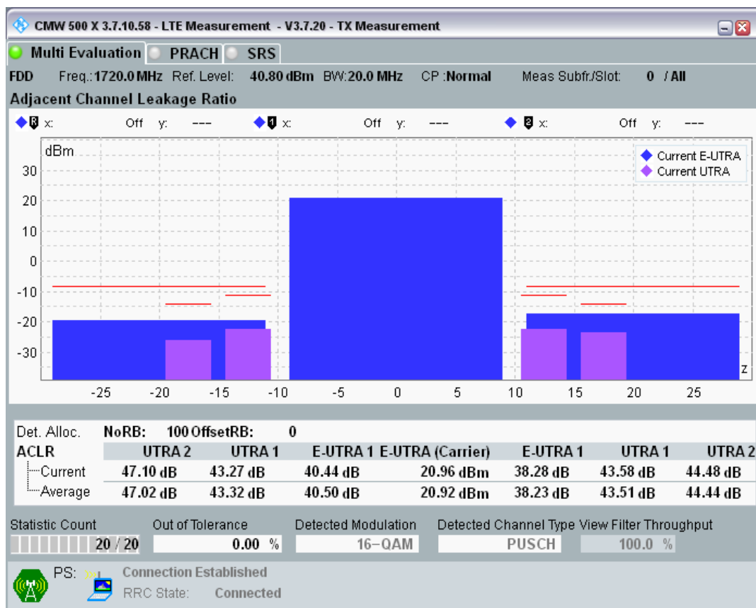
Band3 QAM16 BW=20MHz Channel=19300 RB Size=18 Position=#0.png
