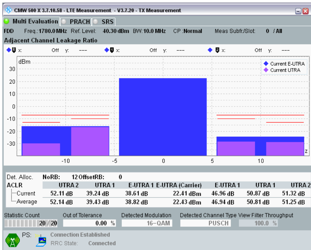
Band3 QAM16 BW=10MHz Channel=19900 RB Size=12 Position=#Max.png
