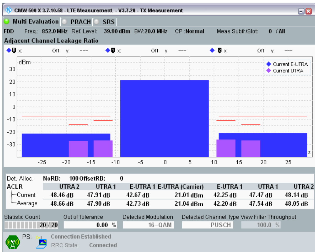
Band20 QAM16 BW=20MHz Channel=24350 RB Size=18 Position=#0.png
