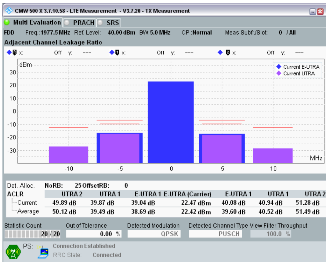
Band1 QPSK BW=5MHz Channel=18575 RB Size=8 Position=#0.png
