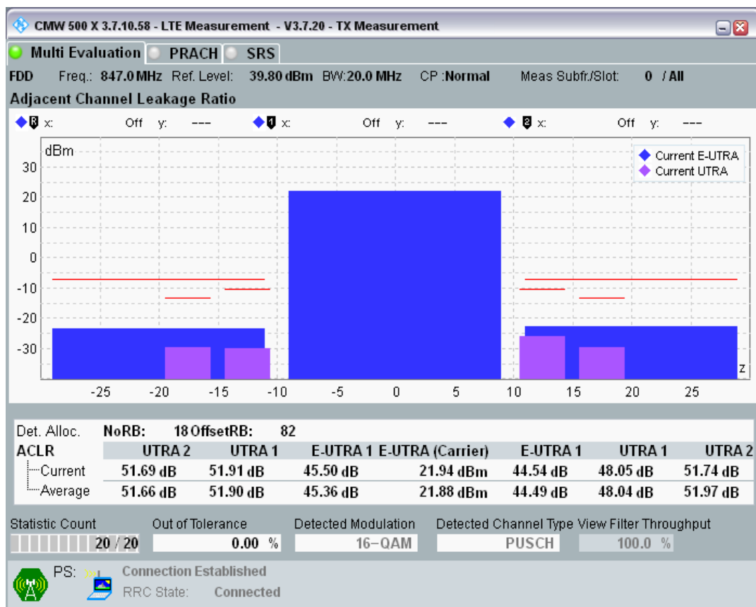
Band20 QAM16 BW=20MHz Channel=24350 RB Size=100 Position=#0.png
