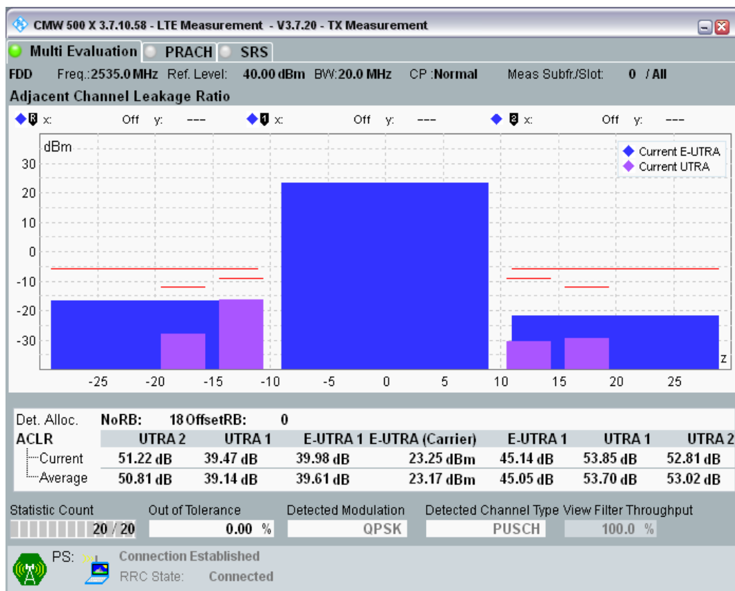
Band7 QPSK BW=20MHz Channel=21100 RB Size=18 Position=#Max.png
