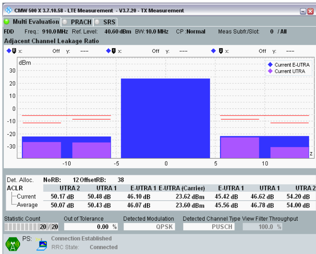
Band8 QPSK BW=10MHz Channel=21750 RB Size=50 Position=#0.png
