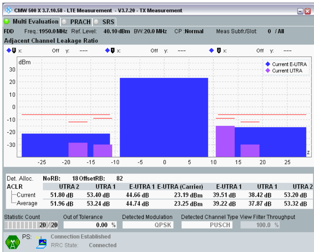
Band1 QPSK BW=20MHz Channel=18500 RB Size=100 Position=#0.png
