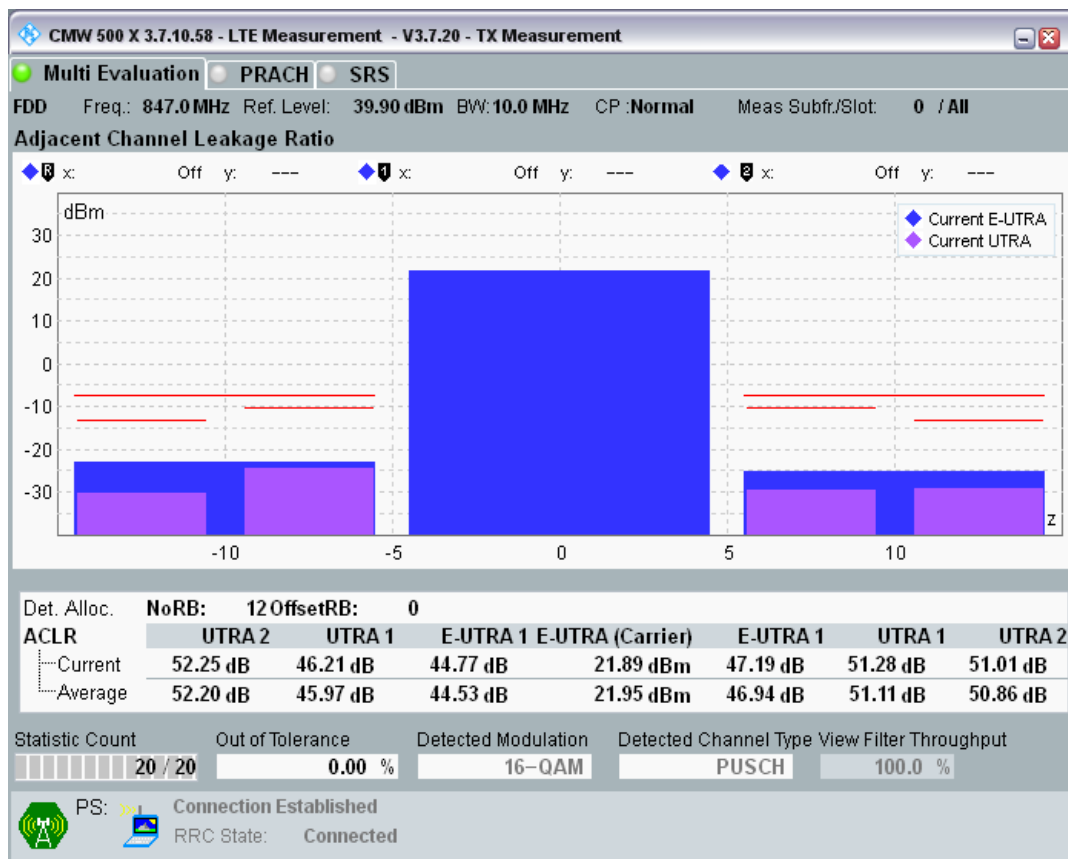
Band20 QAM16 BW=10MHz Channel=24300 RB Size=12 Position=#Max.png
