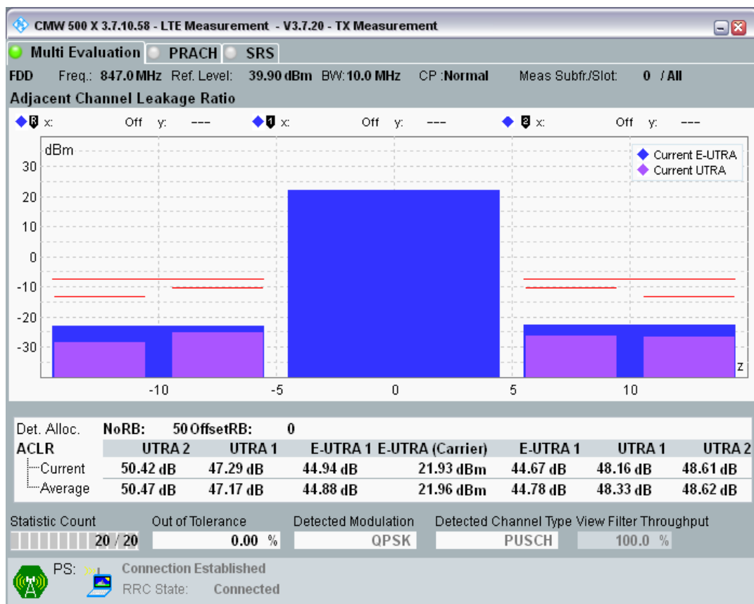
Band20 QPSK BW=10MHz Channel=24400 RB Size=12 Position=#0.png
