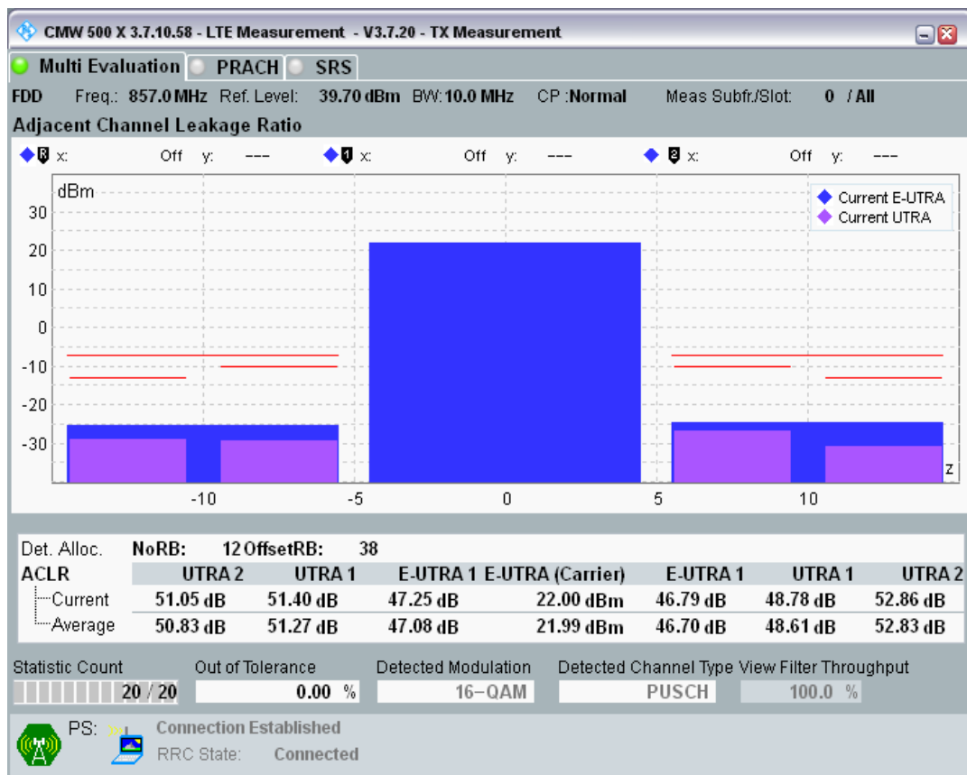
Band20 QAM16 BW=10MHz Channel=24400 RB Size=50 Position=#0.png
