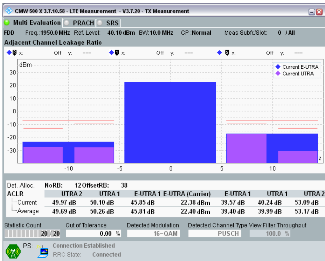
Band1 QAM16 BW=10MHz Channel=18300 RB Size=50 Position=#0.png
