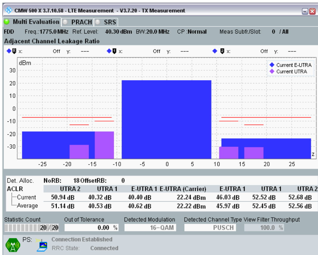
Band3 QAM16 BW=20MHz Channel=19850 RB Size=18 Position=#Max.png
