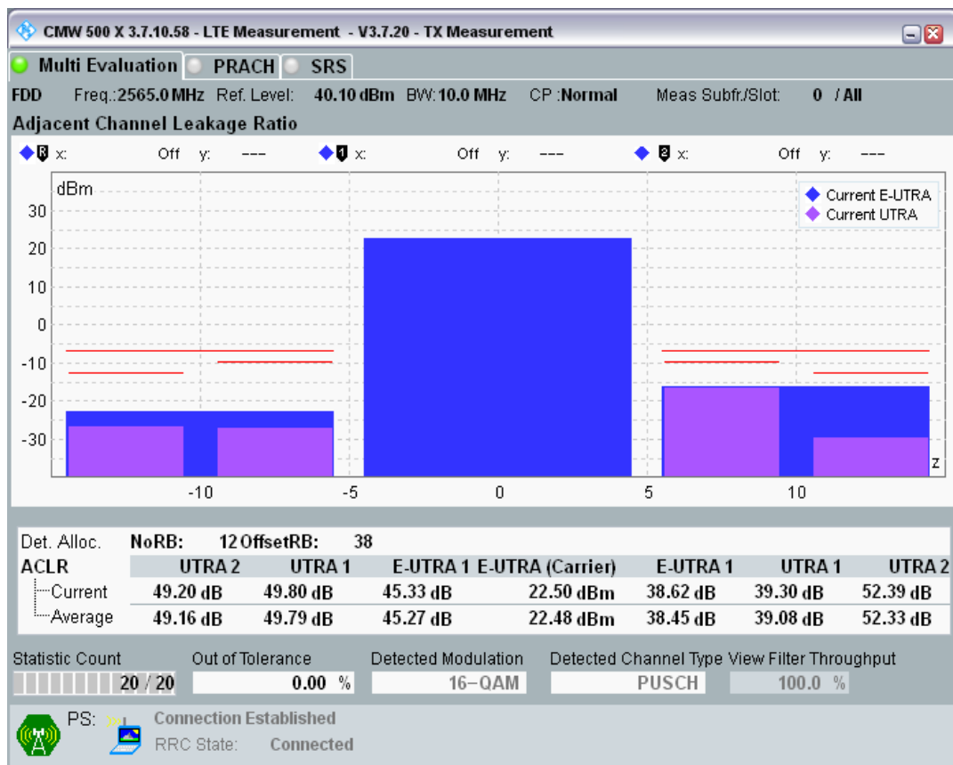
Band7 QAM16 BW=10MHz Channel=21400 RB Size=50 Position=#0.png
