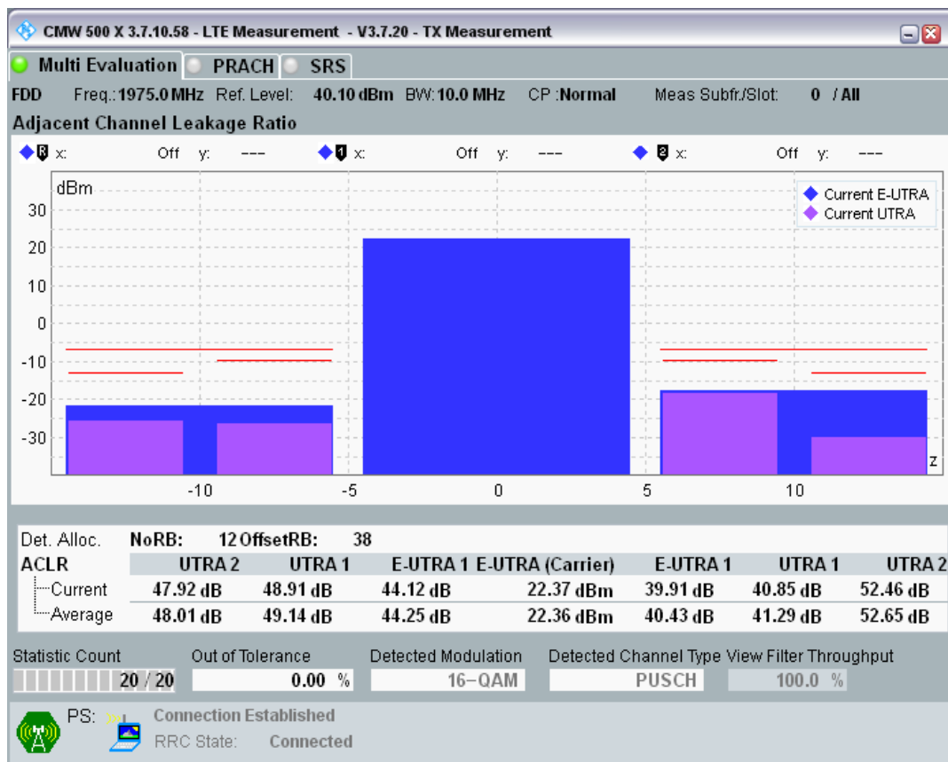
Band1 QAM16 BW=10MHz Channel=18550 RB Size=50 Position=#0.png
