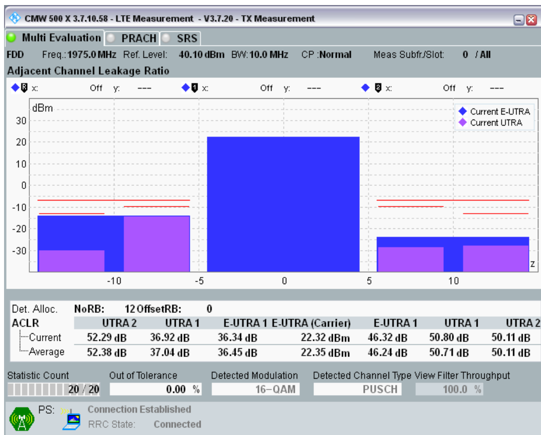
Band1 QAM16 BW=10MHz Channel=18550 RB Size=12 Position=#Max.png
