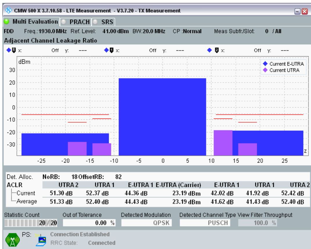
Band1 QPSK BW=20MHz Channel=18300 RB Size=100 Position=#0.png
