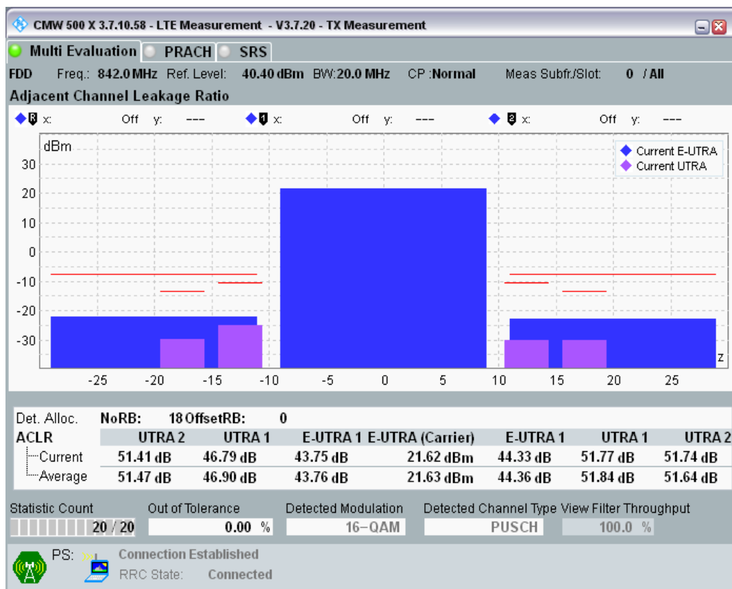
Band20 QAM16 BW=20MHz Channel=24250 RB Size=18 Position=#Max.png
