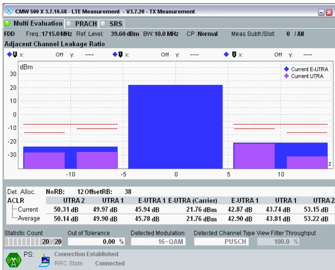
Band3 QAM16 BW=10MHz Channel=19250 RB Size=50 Position=#0.png
