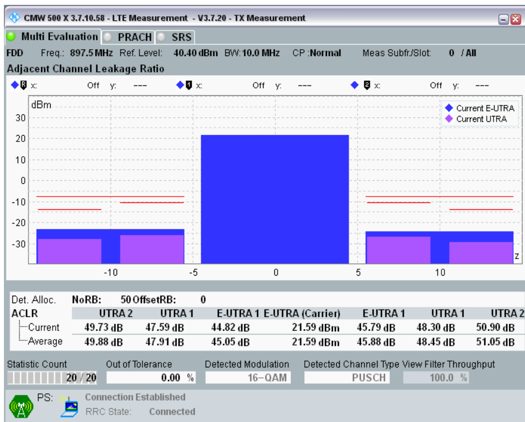
Band8 QAM16 BW=10MHz Channel=21750 RB Size=12 Position=#0.png
