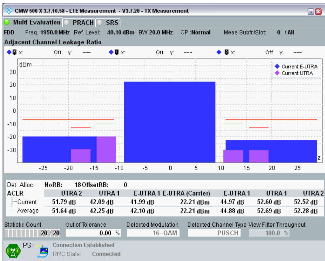
Band1 QAM16 BW=20MHz Channel=18300 RB Size=18 Position=#Max.png
