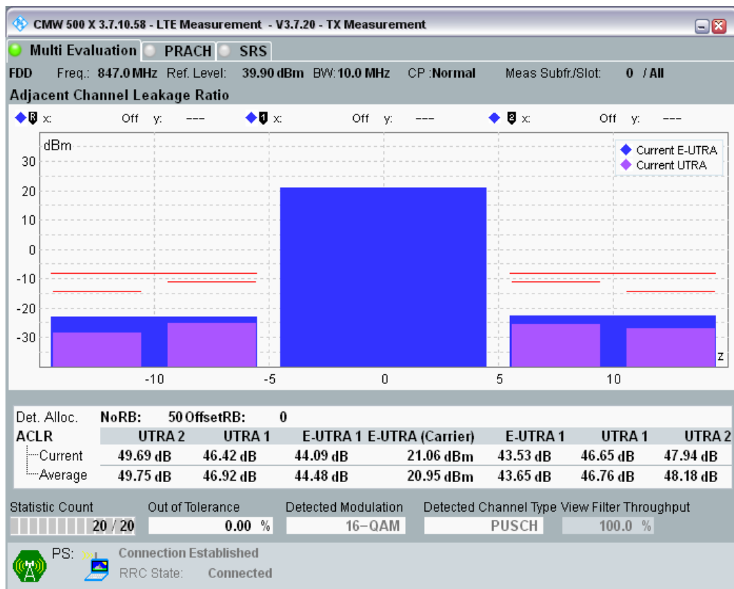
Band20 QAM16 BW=10MHz Channel=24400 RB Size=12 Position=#0.png
