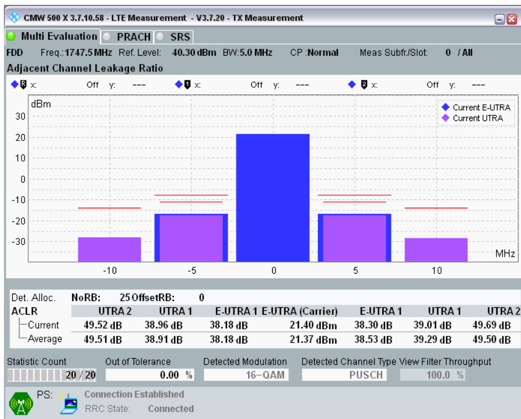
Band3 QAM16 BW=5MHz Channel=19575 RB Size=8 Position=#0.png
