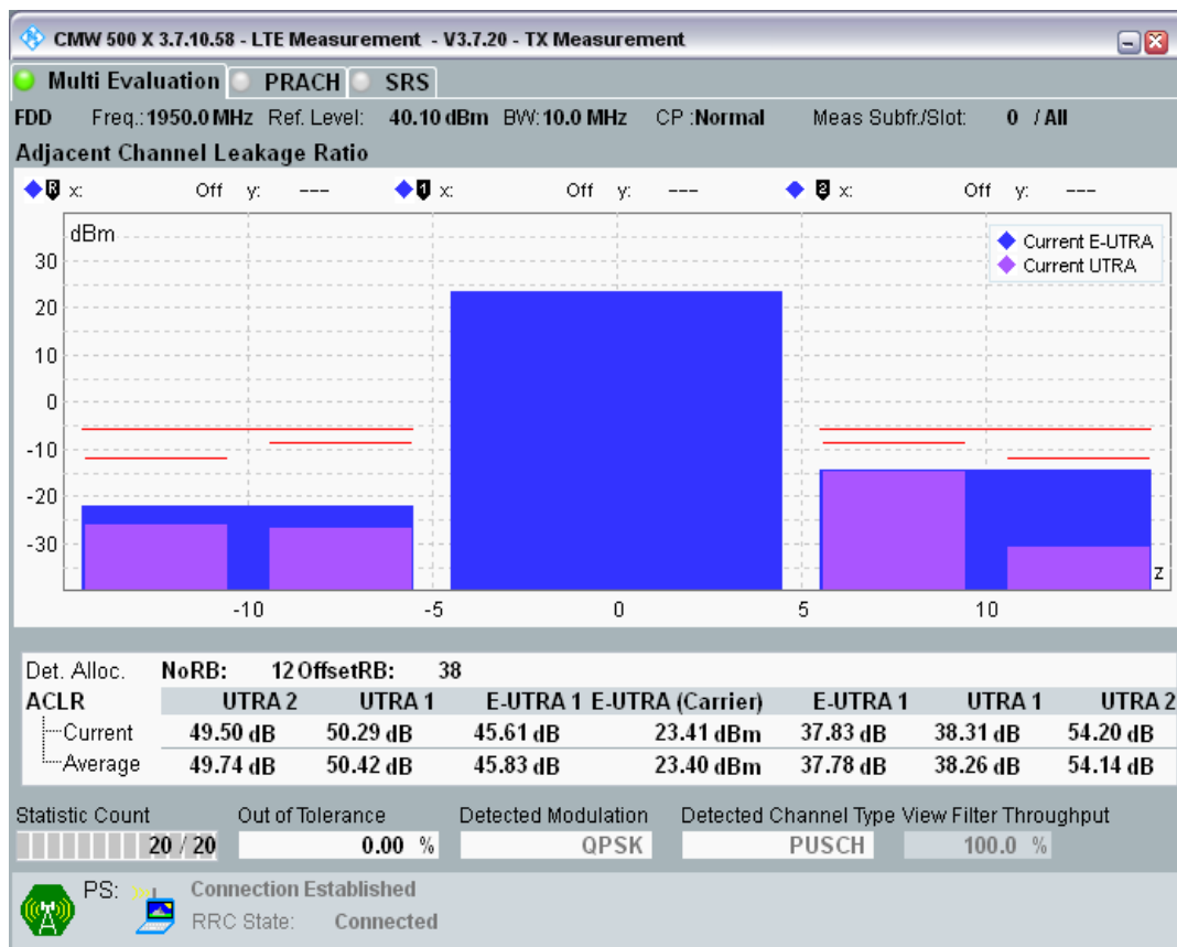
Band1 QPSK BW=10MHz Channel=18300 RB Size=50 Position=#0.png
