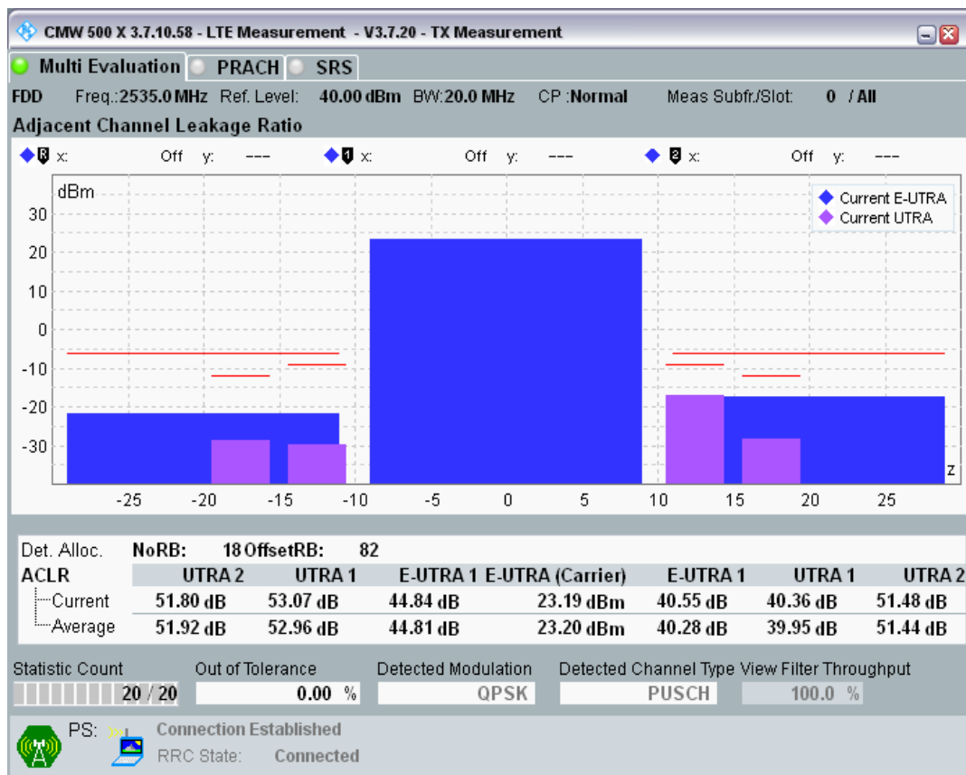
Band7 QPSK BW=20MHz Channel=21350 RB Size=100 Position=#0.png
