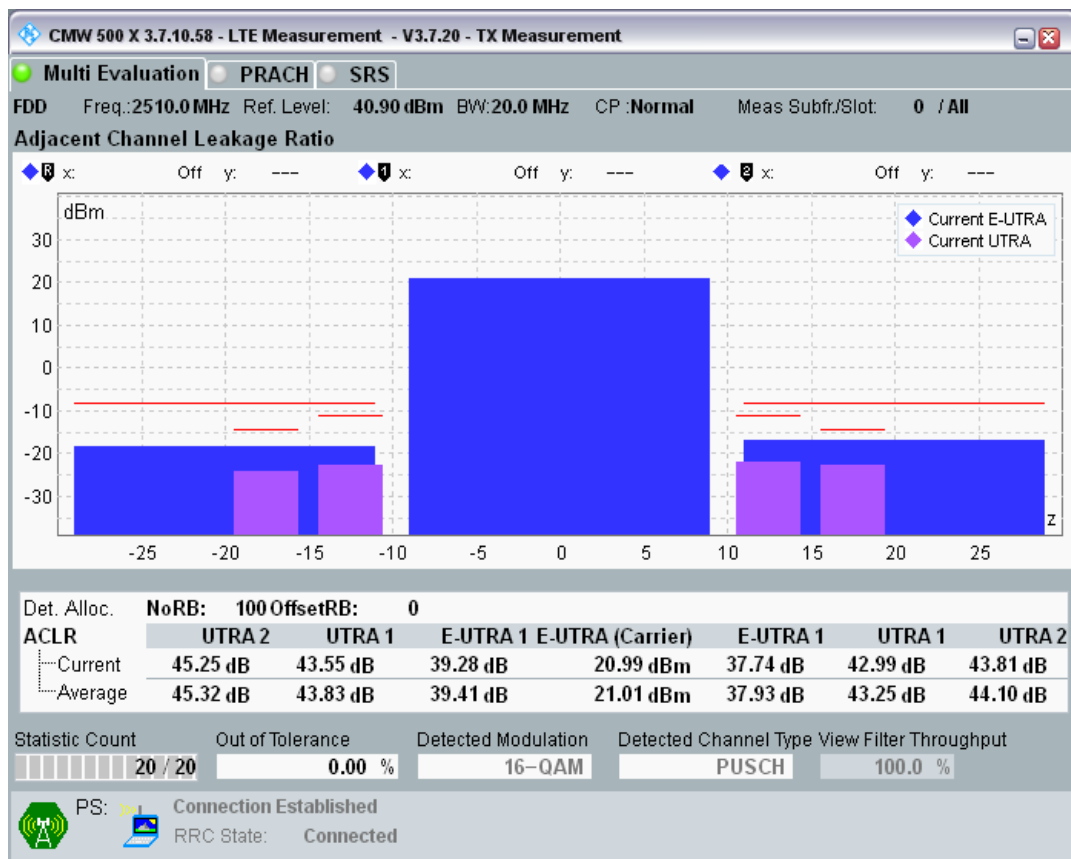
Band7 QAM16 BW=20MHz Channel=20850 RB Size=18 Position=#0.png
