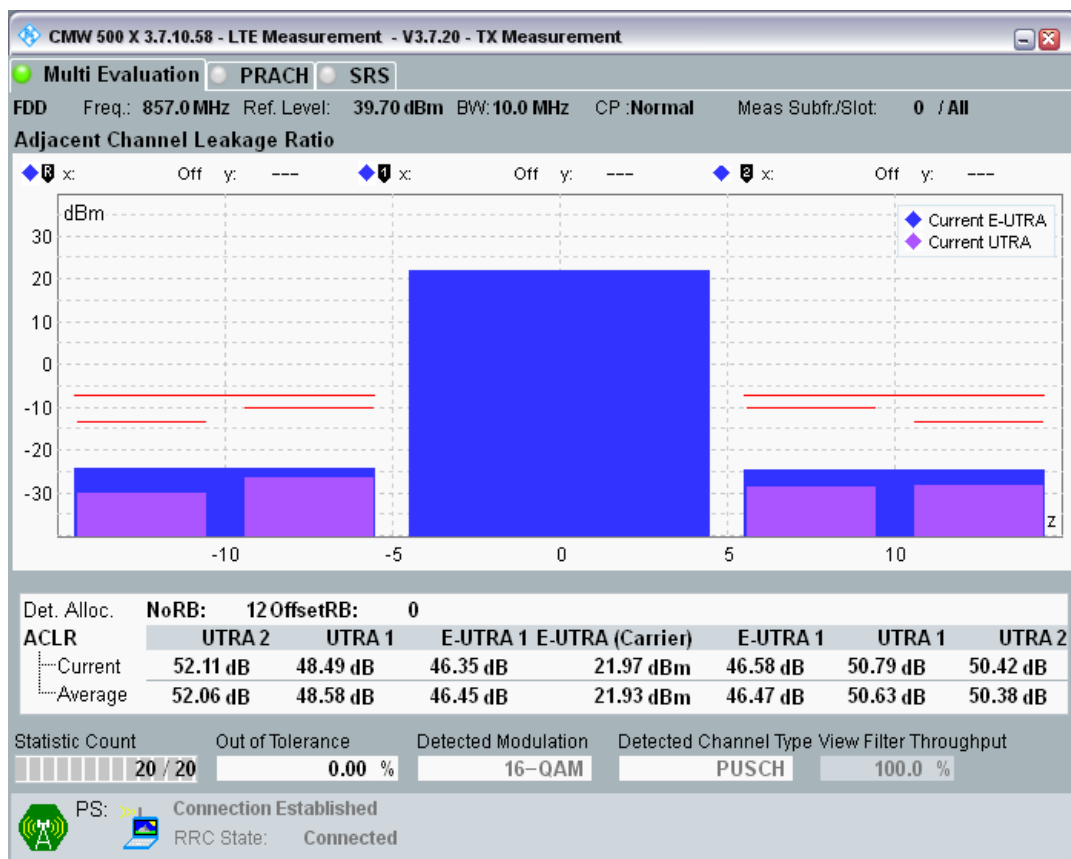
Band20 QAM16 BW=10MHz Channel=24400 RB Size=12 Position=#Max.png
