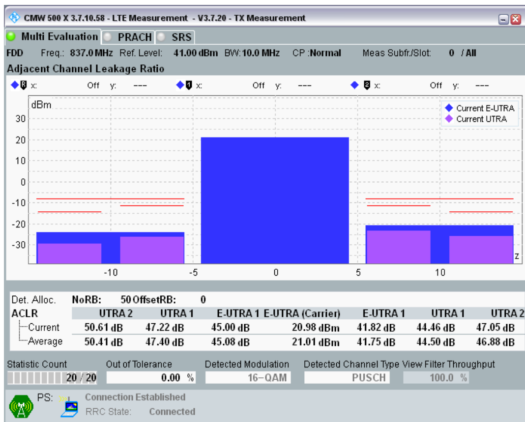
Band20 QAM16 BW=10MHz Channel=24300 RB Size=12 Position=#0.png
