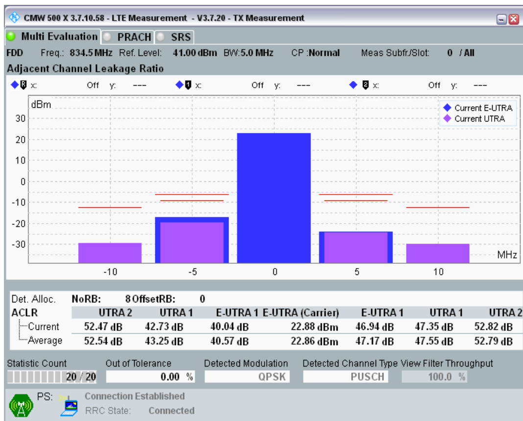
Band20 QPSK BW=5MHz Channel=24175 RB Size=8 Position=#Max.png
