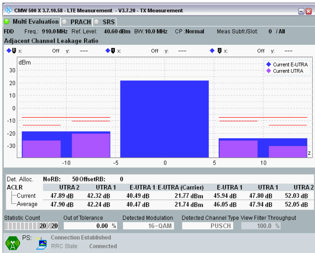
Band8 QAM16 BW=5MHz Channel=21475 RB Size=25 Position=#0.png
