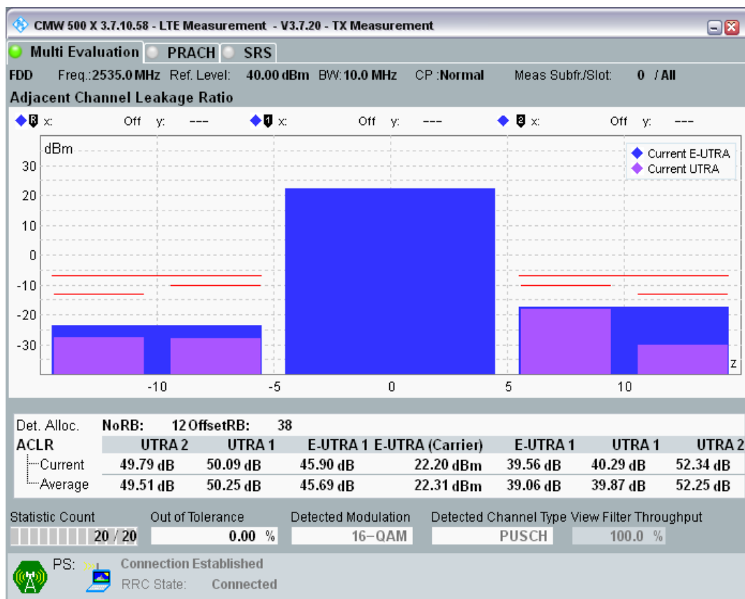
Band7 QAM16 BW=10MHz Channel=21100 RB Size=50 Position=#0.png
