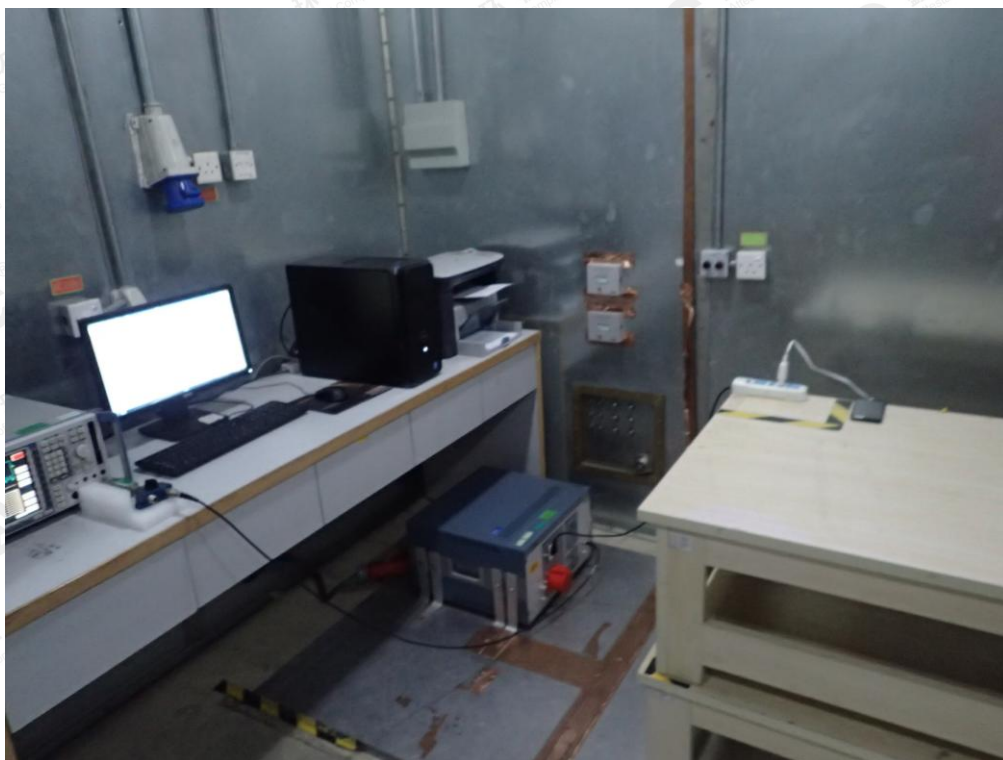
RADIATED EMISSION TEST SETUP
