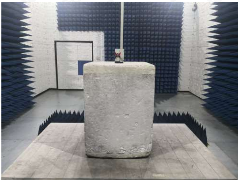
RADIATED SPURIOUS EMISSION ABOVE 1G TEST SETUP
