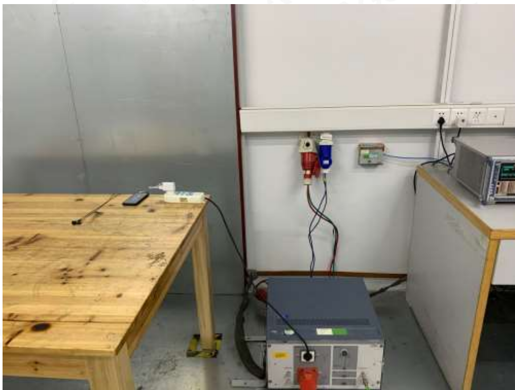
EN 55032 RADIATED EMISSION TEST SETUP
