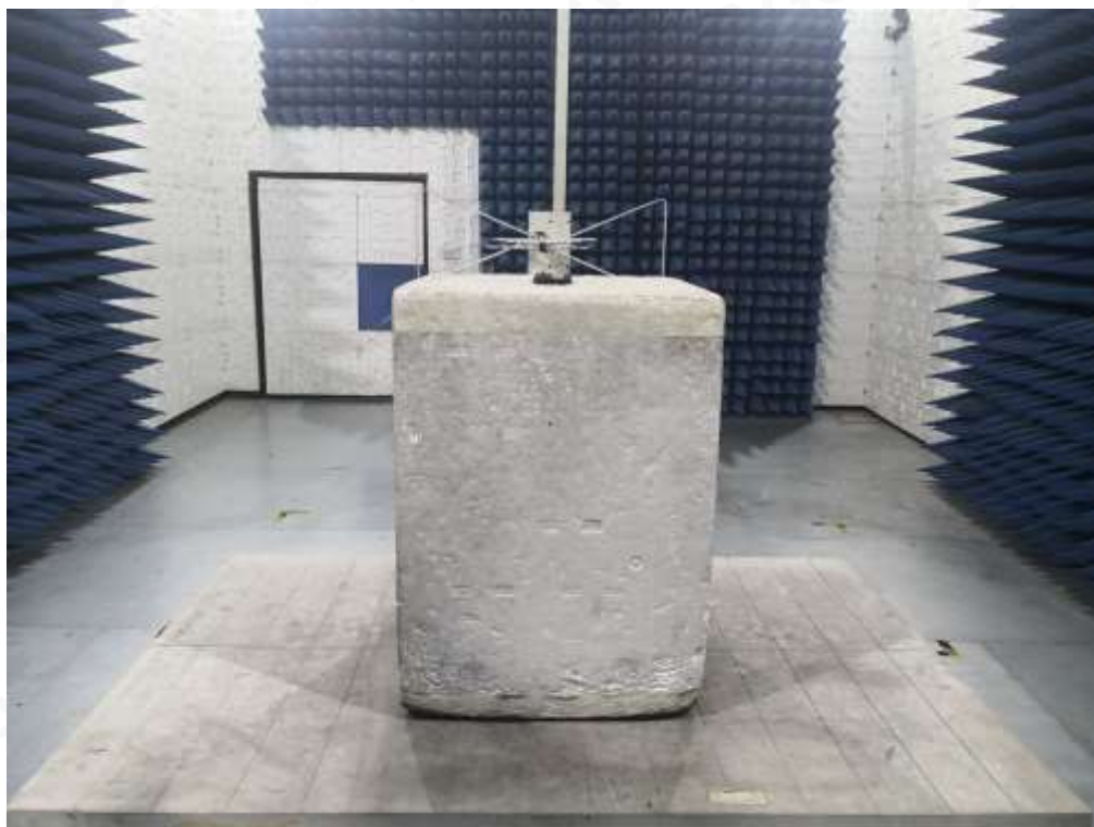
RADIATED SPURIOUS EMISSION ABOVE 1G TEST SETUP
