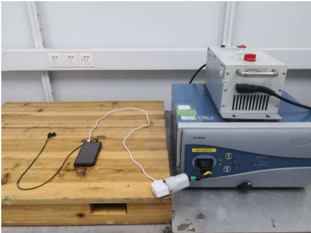
EFT SURGE and DIPS IMMUNITY TEST SETUP
