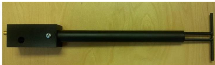
Figure 1 – MVG COMOSAR Validation Dipole
