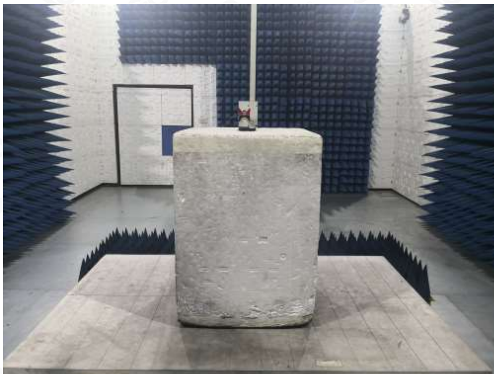
RADIATED SPURIOUS EMISSION ABOVE 1G TEST SETUP
