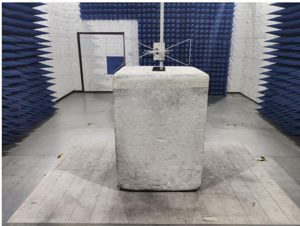
RADIATED SPURIOUS EMISSION ABOVE 1G TEST SETUP
