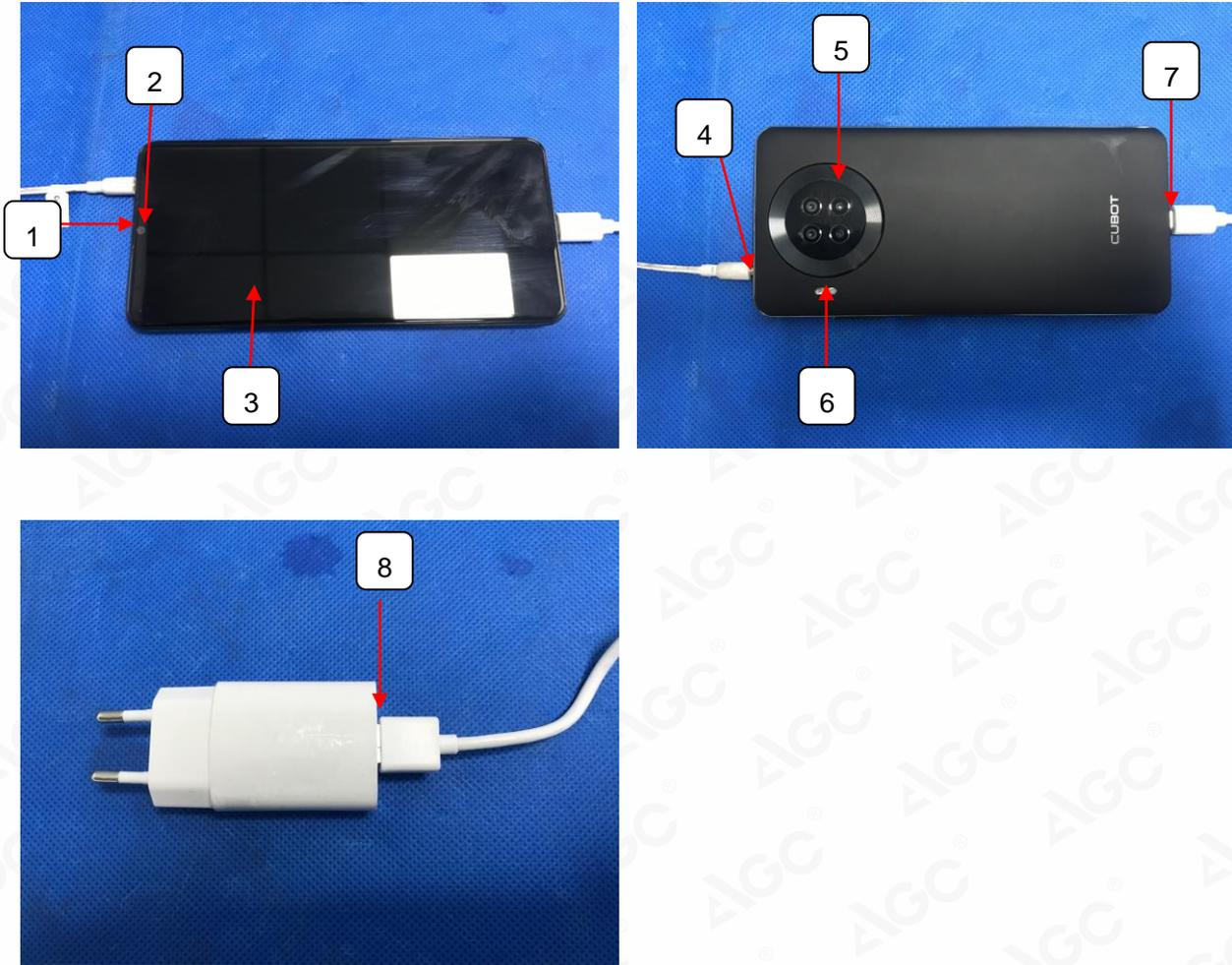
**Note:** The air discharge points are 1~3, 5, 6. The contact discharge points are 4, 7 and 8.
