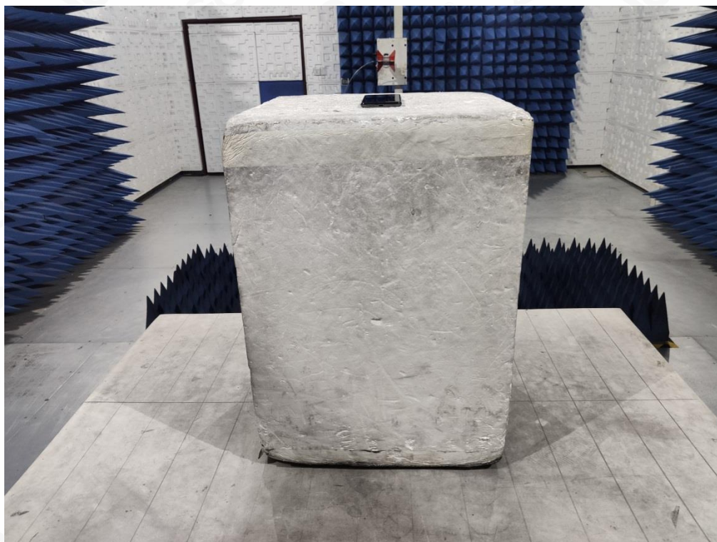
RADIATED SPURIOUS EMISSION ABOVE 1G TEST SETUP
