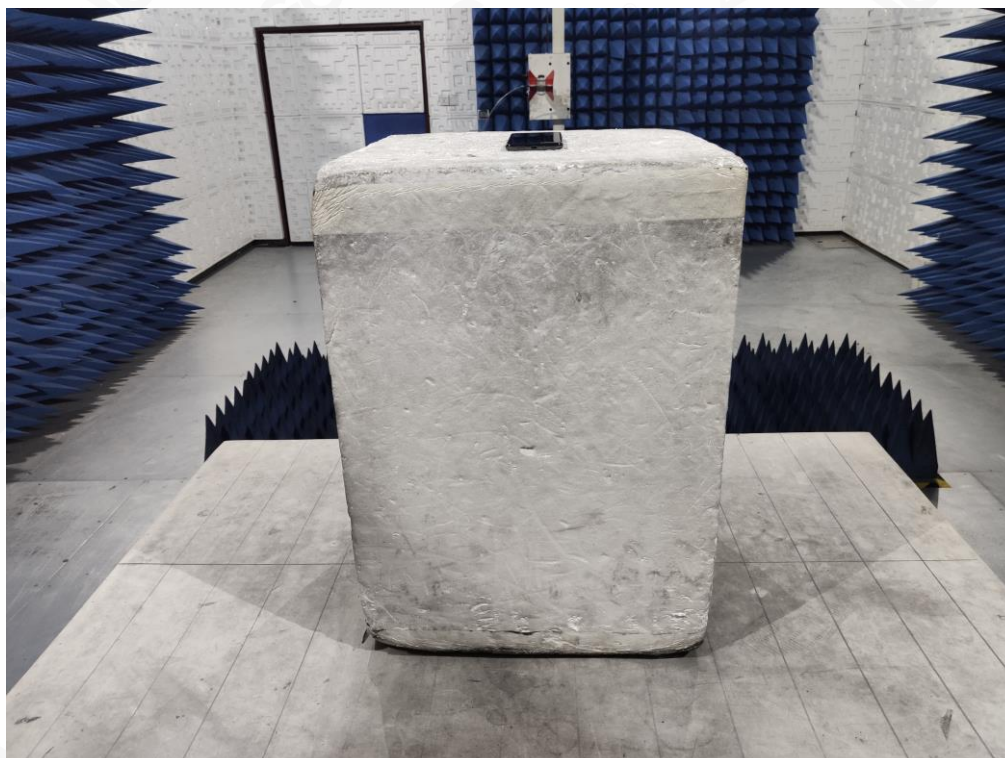
RADIATED SPURIOUS EMISSION ABOVE 1G TEST SETUP
