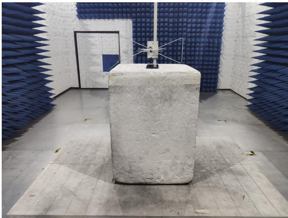
RADIATED SPURIOUS EMISSION ABOVE 1G TEST SETUP
