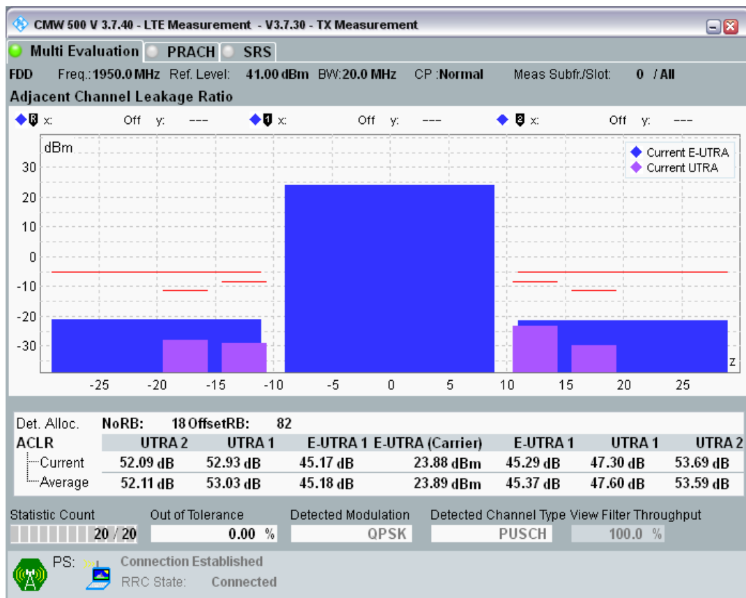
Band1 QPSK BW=20MHz Channel=18500 RB Size=100 Position=#0.png
