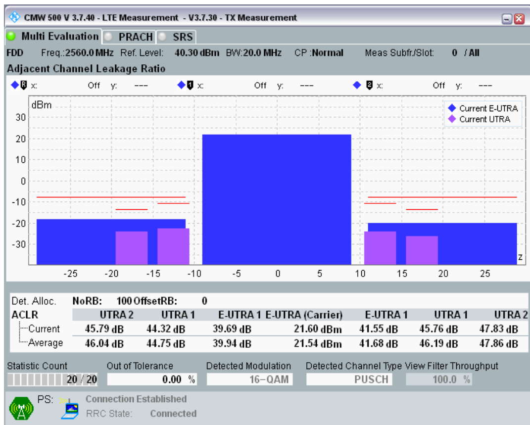
Band7 QAM16 BW=20MHz Channel=21350 RB Size=18 Position=#0.png
