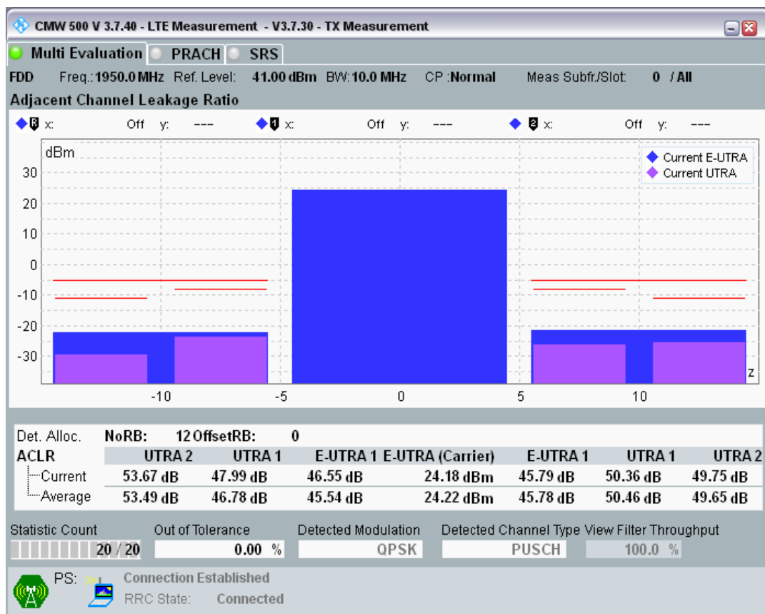
Band1 QPSK BW=10MHz Channel=18300 RB Size=12 Position=#Max.png
