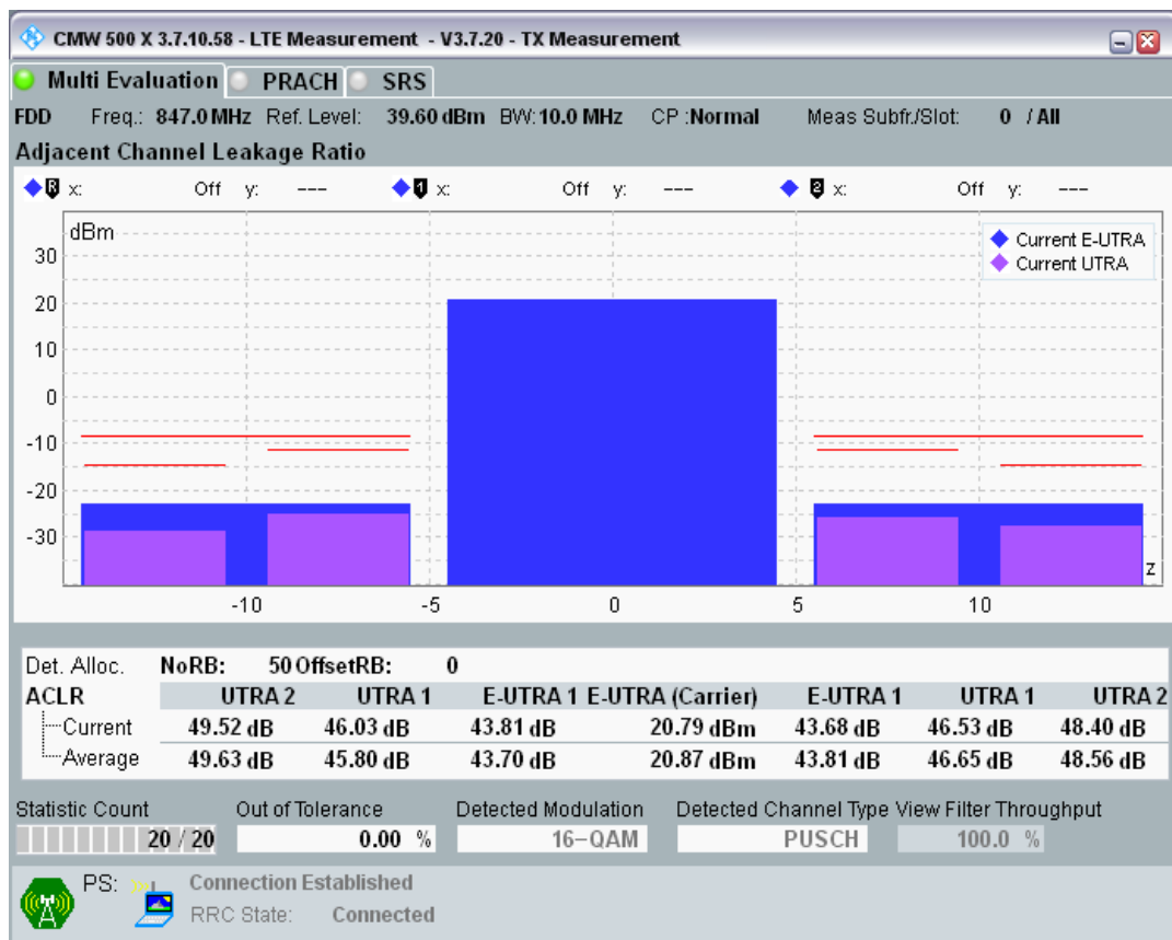
Band20 QAM16 BW=10MHz Channel=24400 RB Size=12 Position=#0.png
