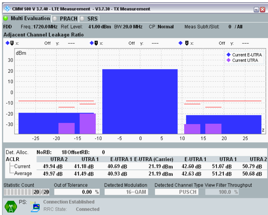
Band3 QAM16 BW=20MHz Channel=19300 RB Size=18 Position=#Max.png
