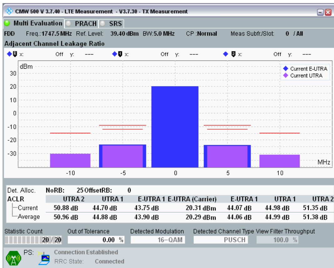
Band3 QAM16 BW=5MHz Channel=19575 RB Size=8 Position=#0.png
