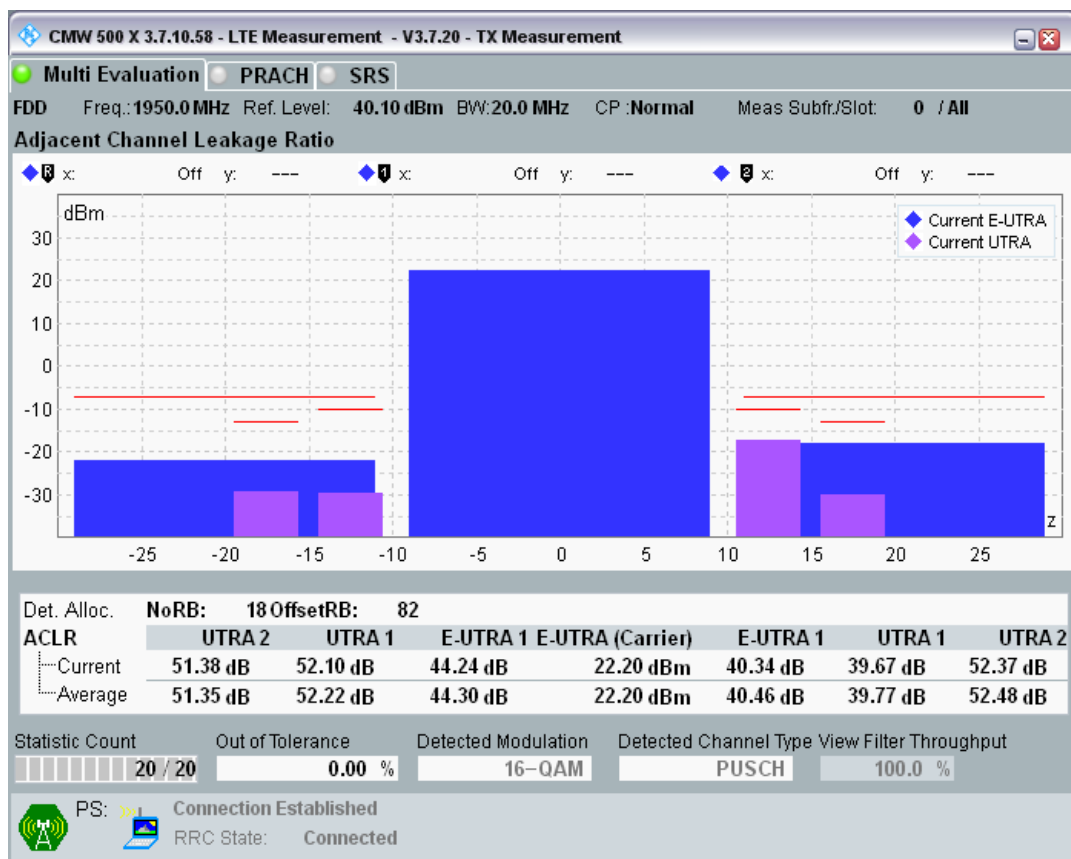
Band1 QAM16 BW=20MHz Channel=18500 RB Size=100 Position=#0.png
