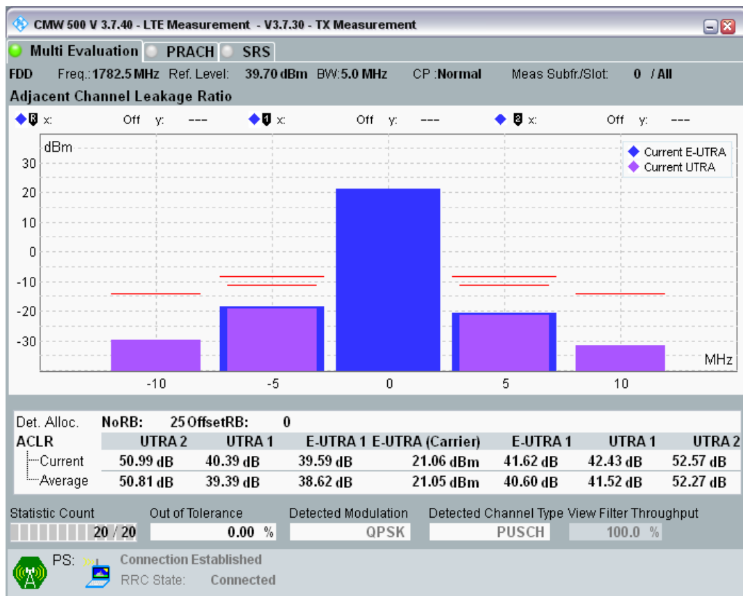
Band3 QPSK BW=5MHz Channel=19925 RB Size=8 Position=#0.png
