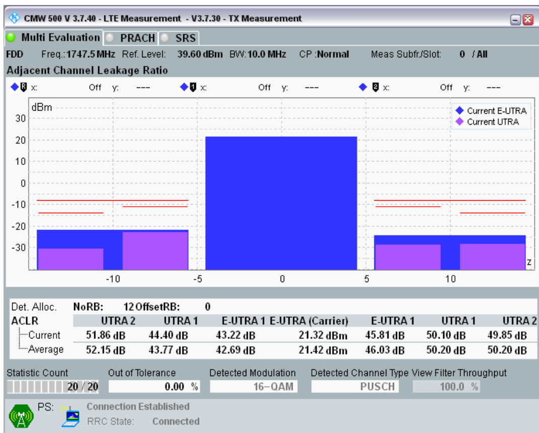
Band3 QAM16 BW=10MHz Channel=19575 RB Size=12 Position=#Max.png
