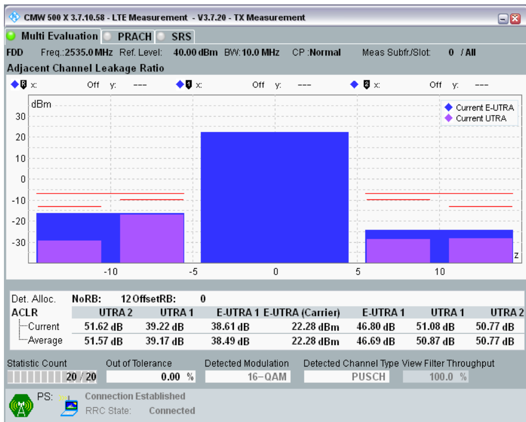
Band7 QAM16 BW=10MHz Channel=21100 RB Size=12 Position=#Max.png
