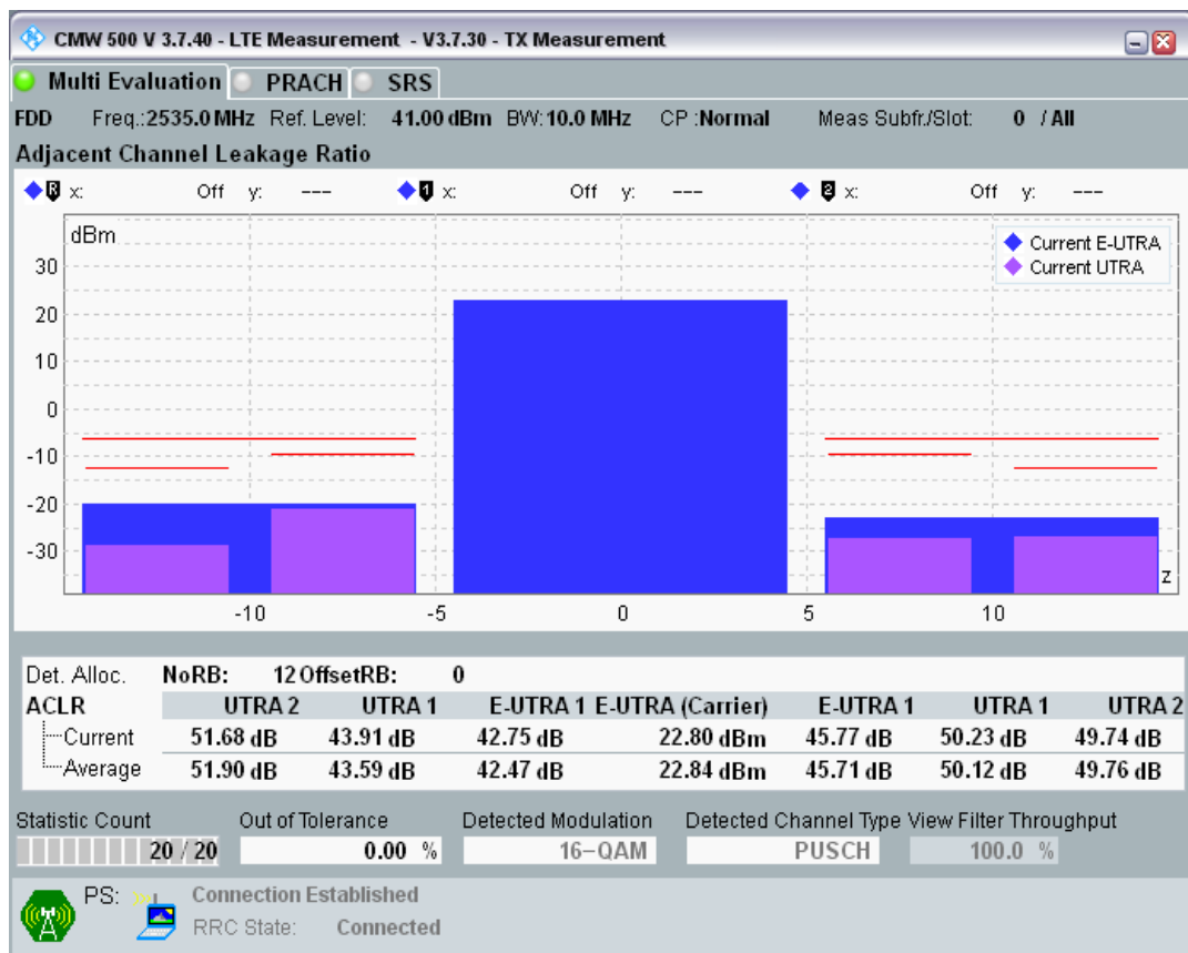
Band7 QAM16 BW=10MHz Channel=21100 RB Size=12 Position=#Max.png
