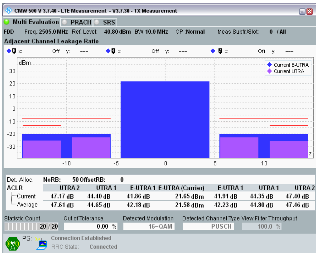
Band7 QAM16 BW=10MHz Channel=21100 RB Size=12 Position=#0.png
