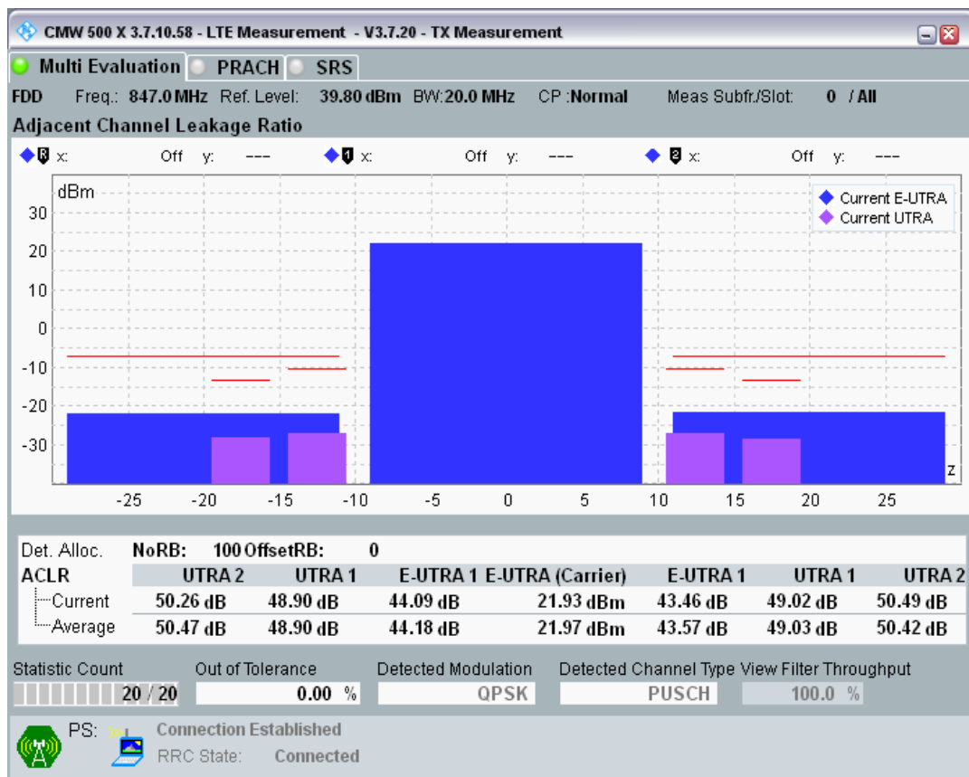
Band20 QPSK BW=20MHz Channel=24300 RB Size=18 Position=#0.png
