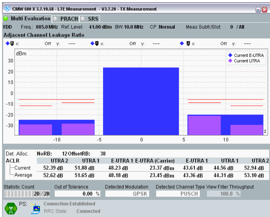
Band8 QPSK BW=10MHz Channel=21500 RB Size=50 Position=#0.png
