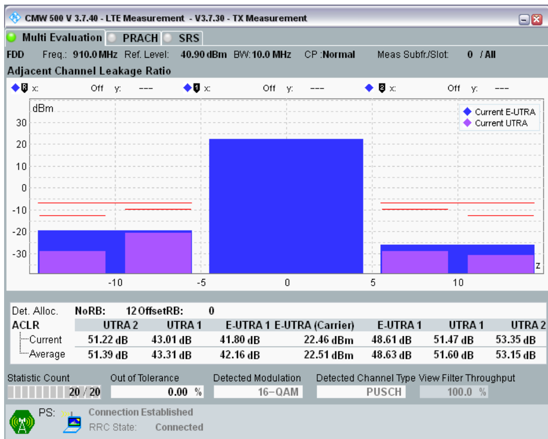
Band8 QAM16 BW=10MHz Channel=21750 RB Size=12 Position=#Max.png
