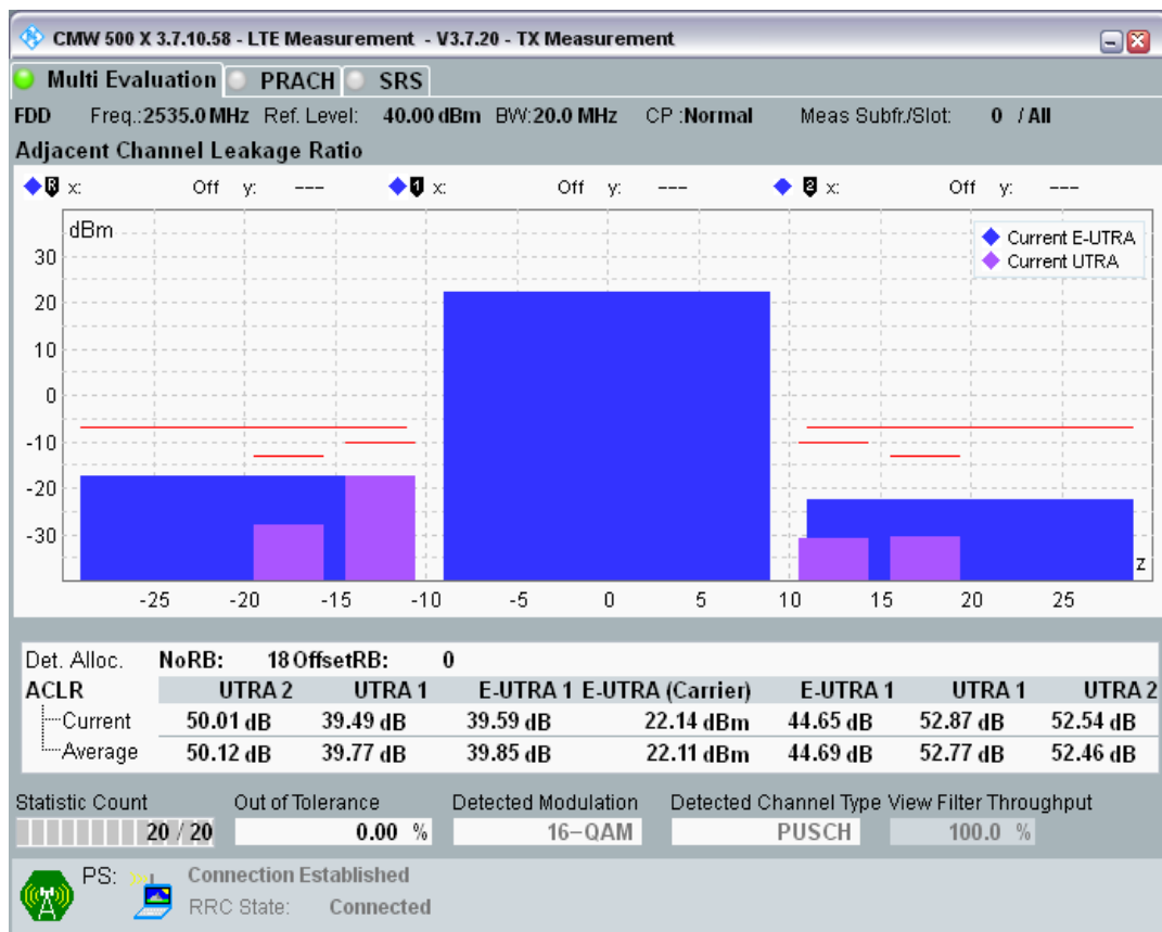
Band7 QAM16 BW=20MHz Channel=21100 RB Size=18 Position=#Max.png
