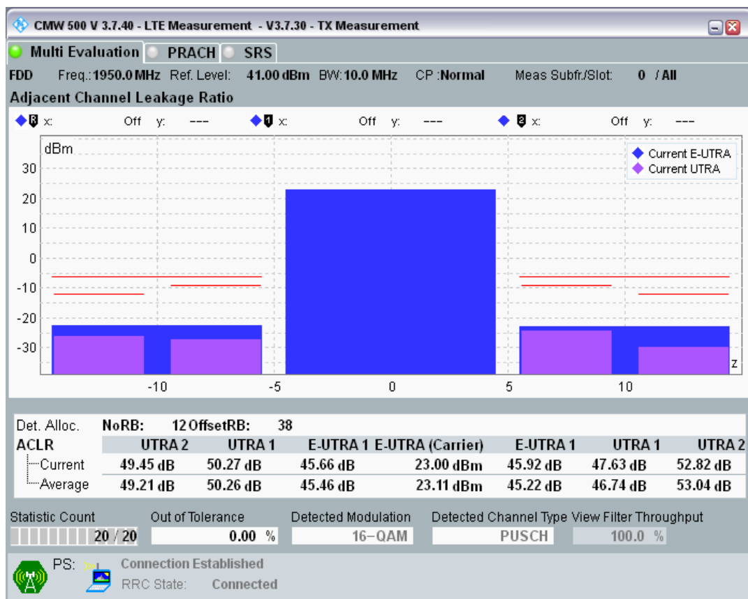
Band1 QAM16 BW=10MHz Channel=18300 RB Size=50 Position=#0.png
