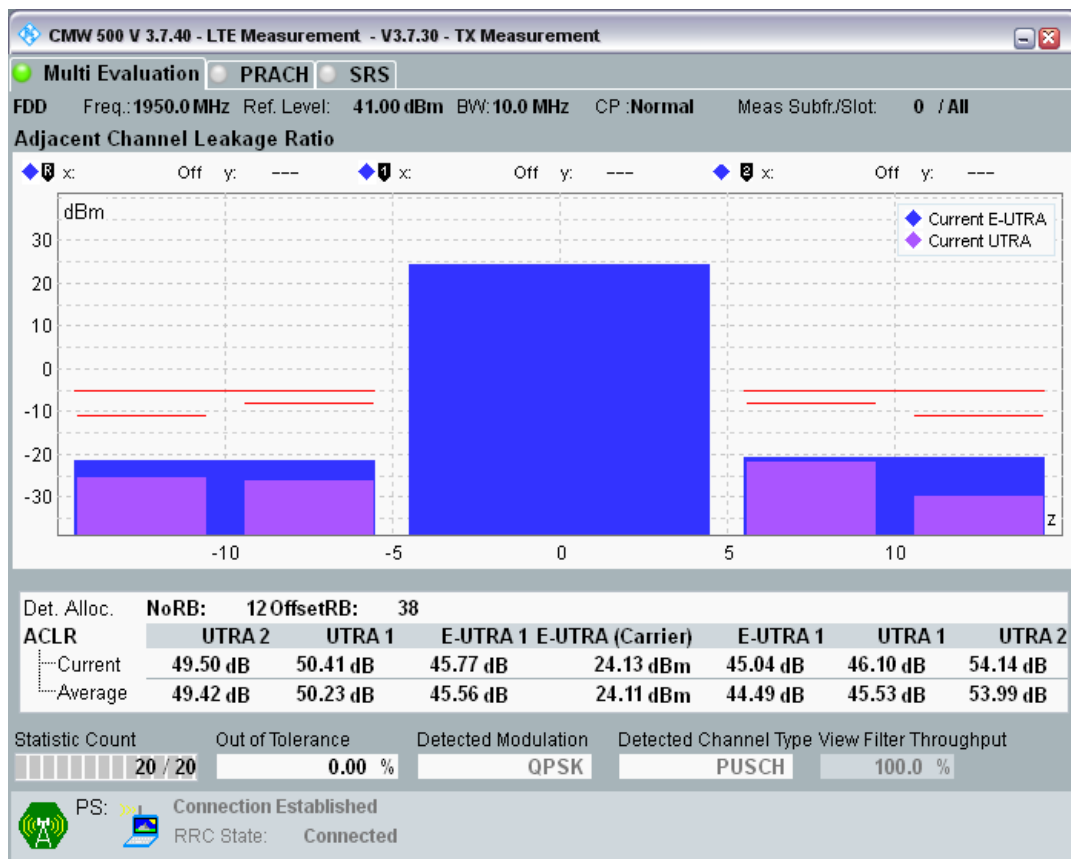
Band1 QPSK BW=10MHz Channel=18300 RB Size=50 Position=#0.png
