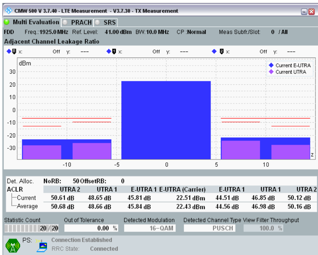
Band1 QAM16 BW=10MHz Channel=18300 RB Size=12 Position=#0.png
