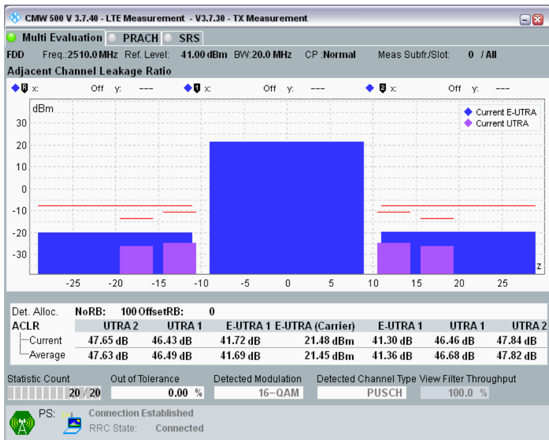
Band7 QAM16 BW=20MHz Channel=20850 RB Size=18 Position=#0.png
