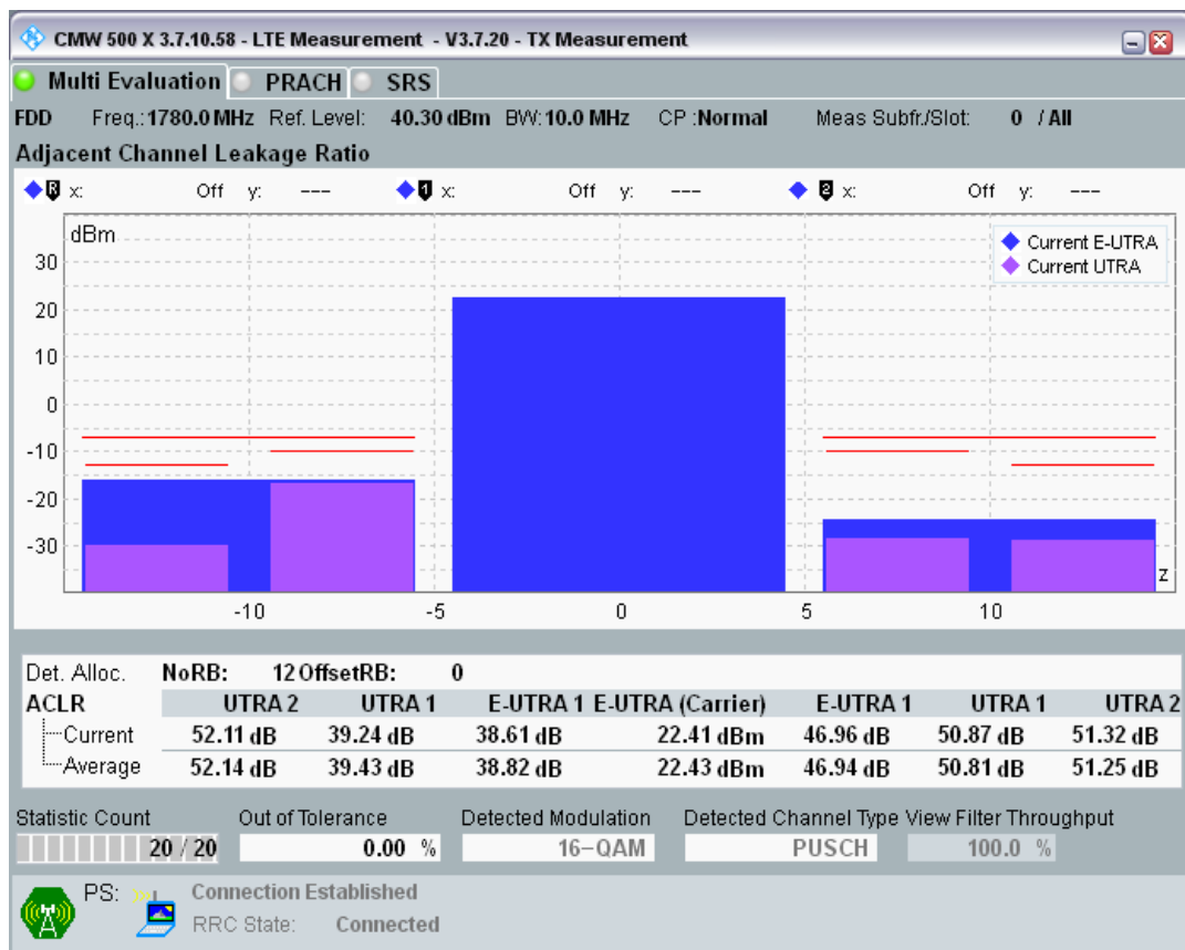
Band3 QAM16 BW=10MHz Channel=19900 RB Size=12 Position=#Max.png
