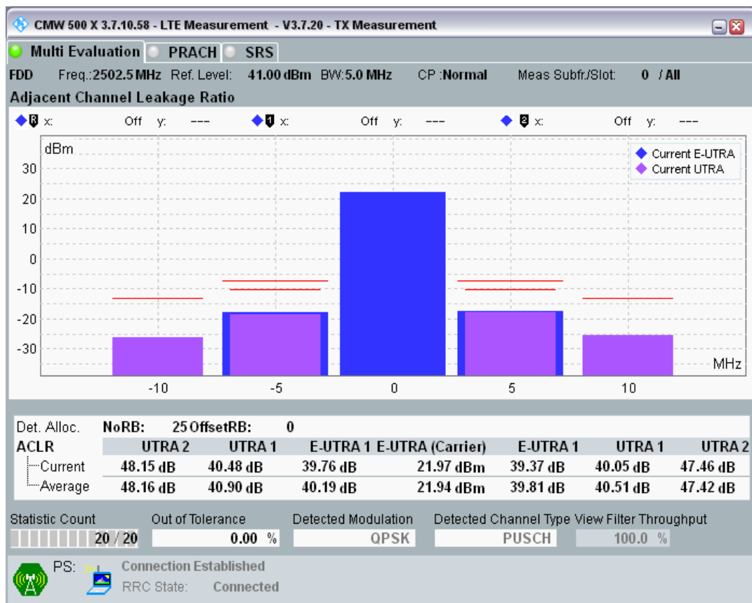
Band7 QPSK BW=5MHz Channel=20775 RB Size=8 Position=#0.png
