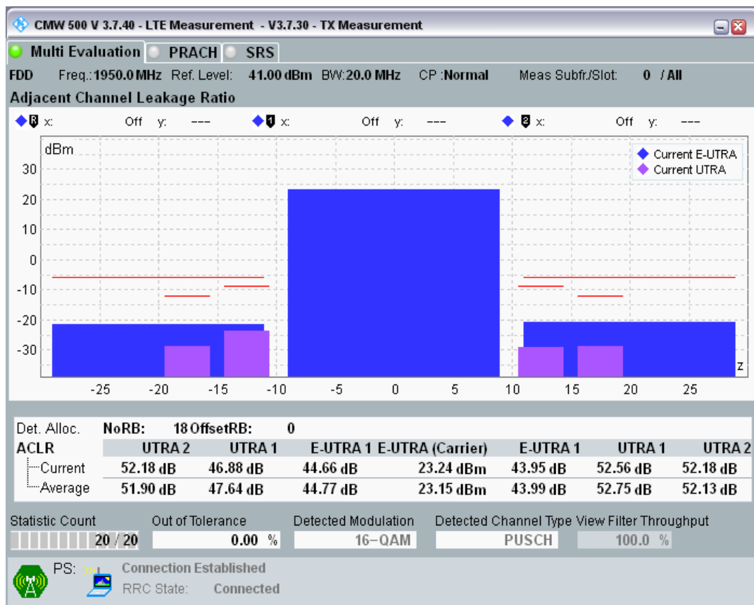
Band1 QAM16 BW=20MHz Channel=18300 RB Size=18 Position=#Max.png
