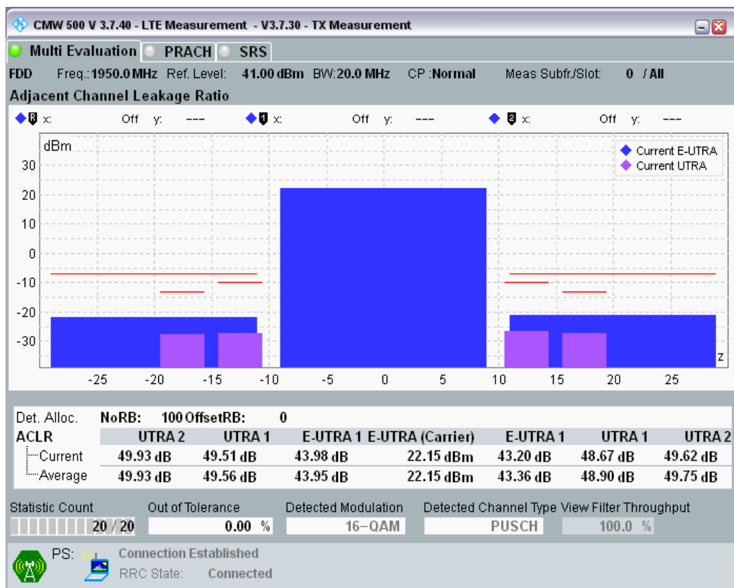
Band1 QAM16 BW=20MHz Channel=18300 RB Size=18 Position=#0.png
