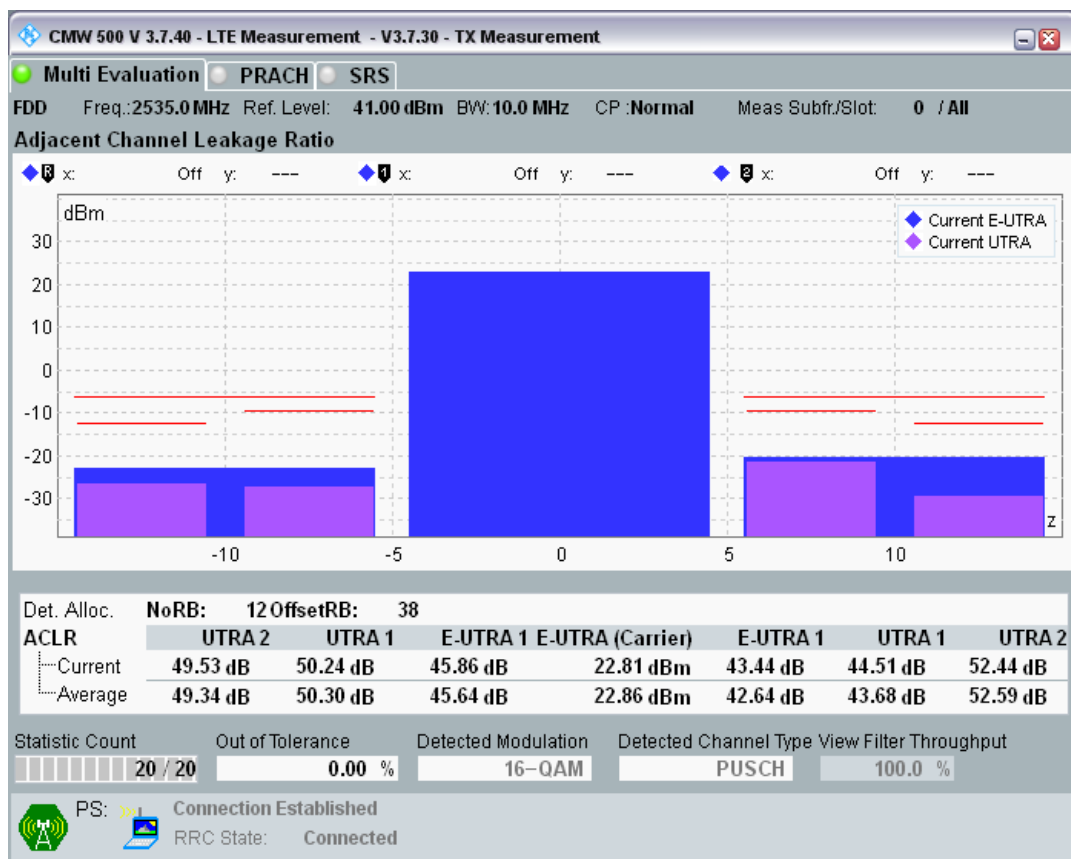
Band7 QAM16 BW=10MHz Channel=21100 RB Size=50 Position=#0.png
