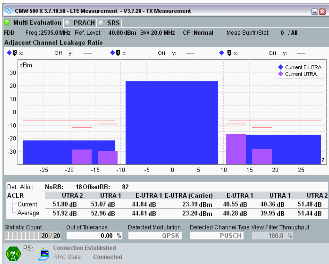
Band7 QPSK BW=20MHz Channel=21350 RB Size=100 Position=#0.png
