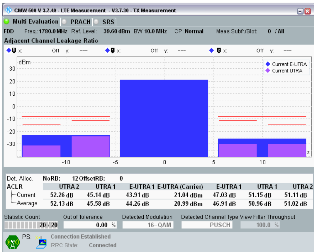
Band3 QAM16 BW=10MHz Channel=19900 RB Size=12 Position=#Max.png
