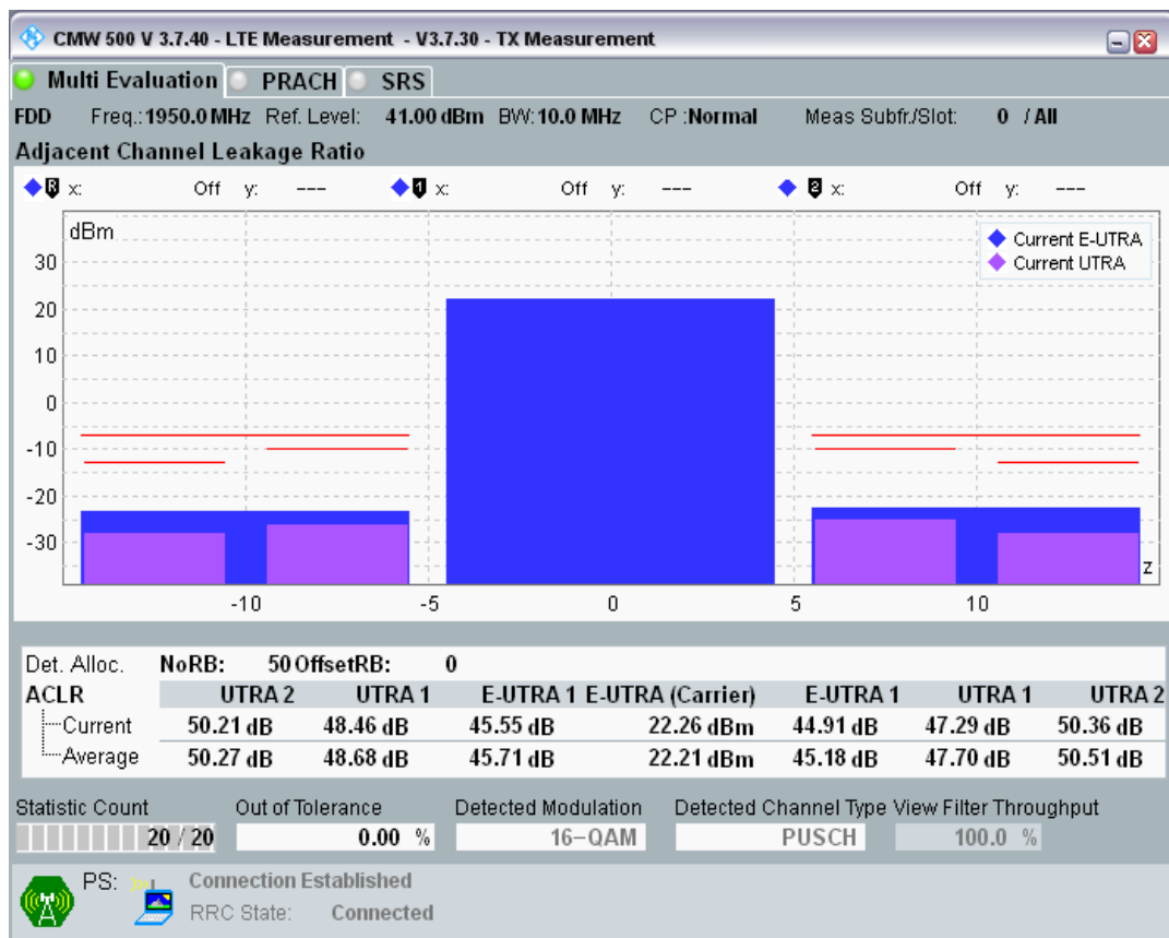
Band1 QAM16 BW=10MHz Channel=18550 RB Size=12 Position=#0.png
