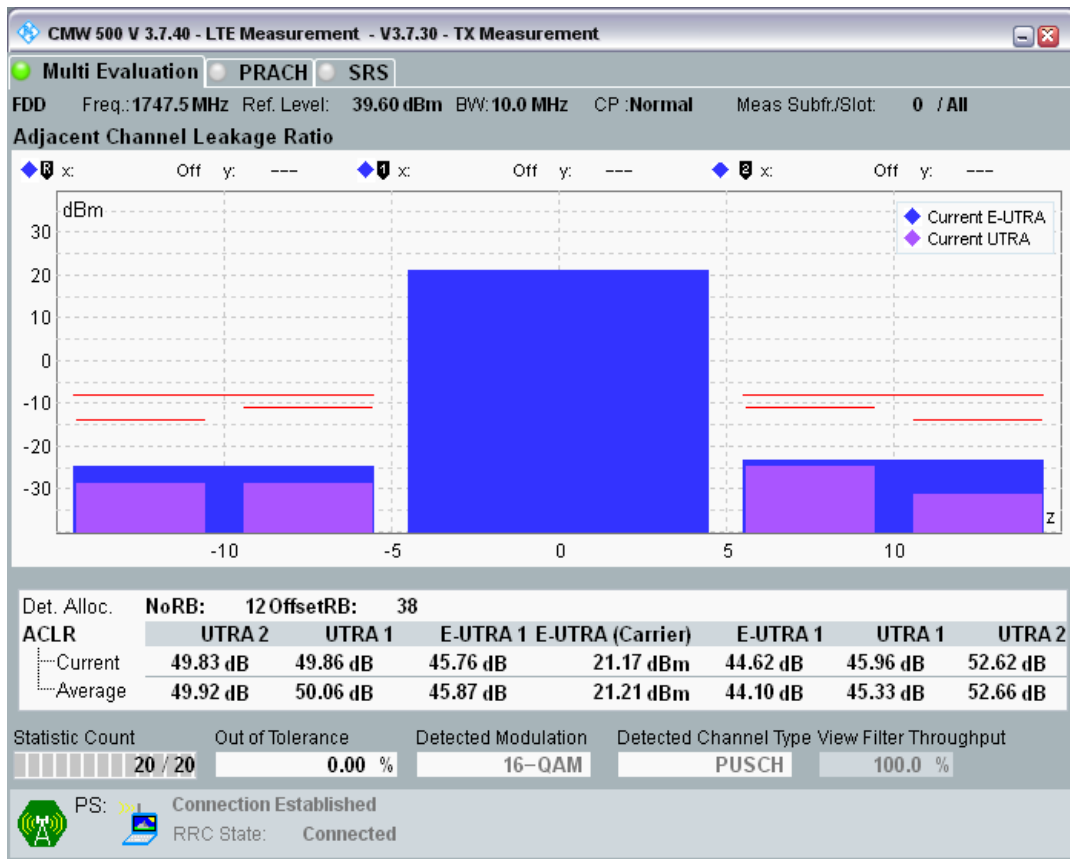
Band3 QAM16 BW=10MHz Channel=19575 RB Size=50 Position=#0.png
