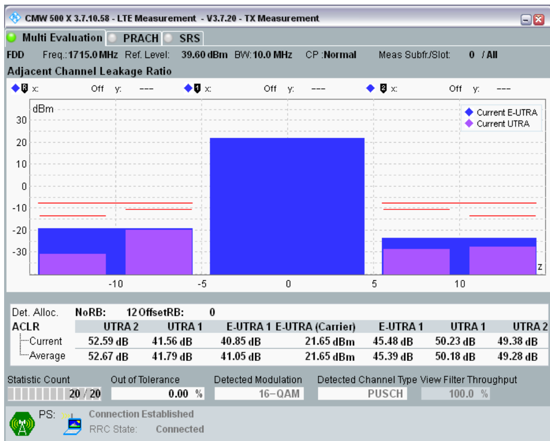
Band3 QAM16 BW=10MHz Channel=19250 RB Size=12 Position=#Max.png
