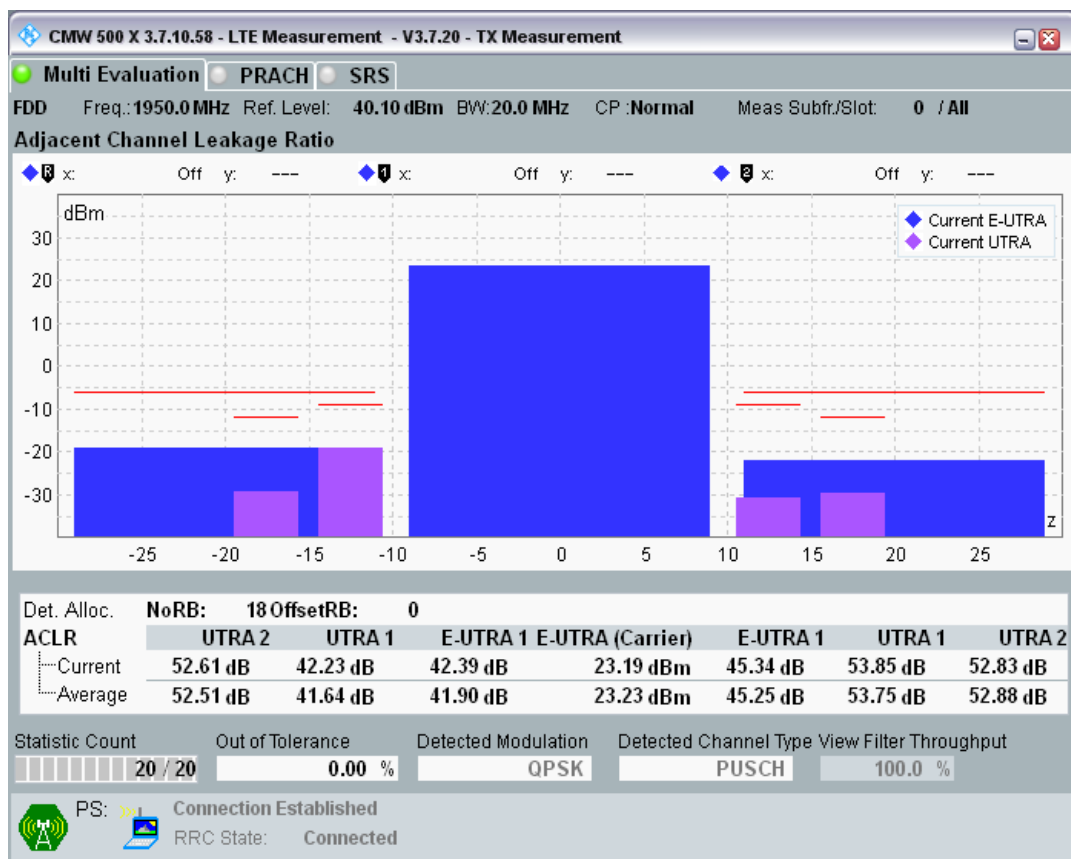
Band1 QPSK BW=20MHz Channel=18300 RB Size=18 Position=#Max.png
