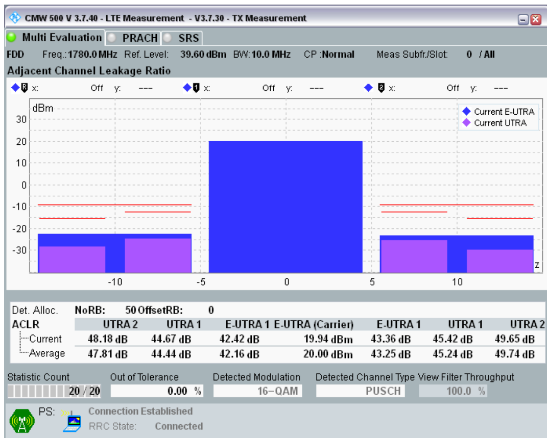
Band3 QAM16 BW=20MHz Channel=19300 RB Size=100 Position=#0.png
