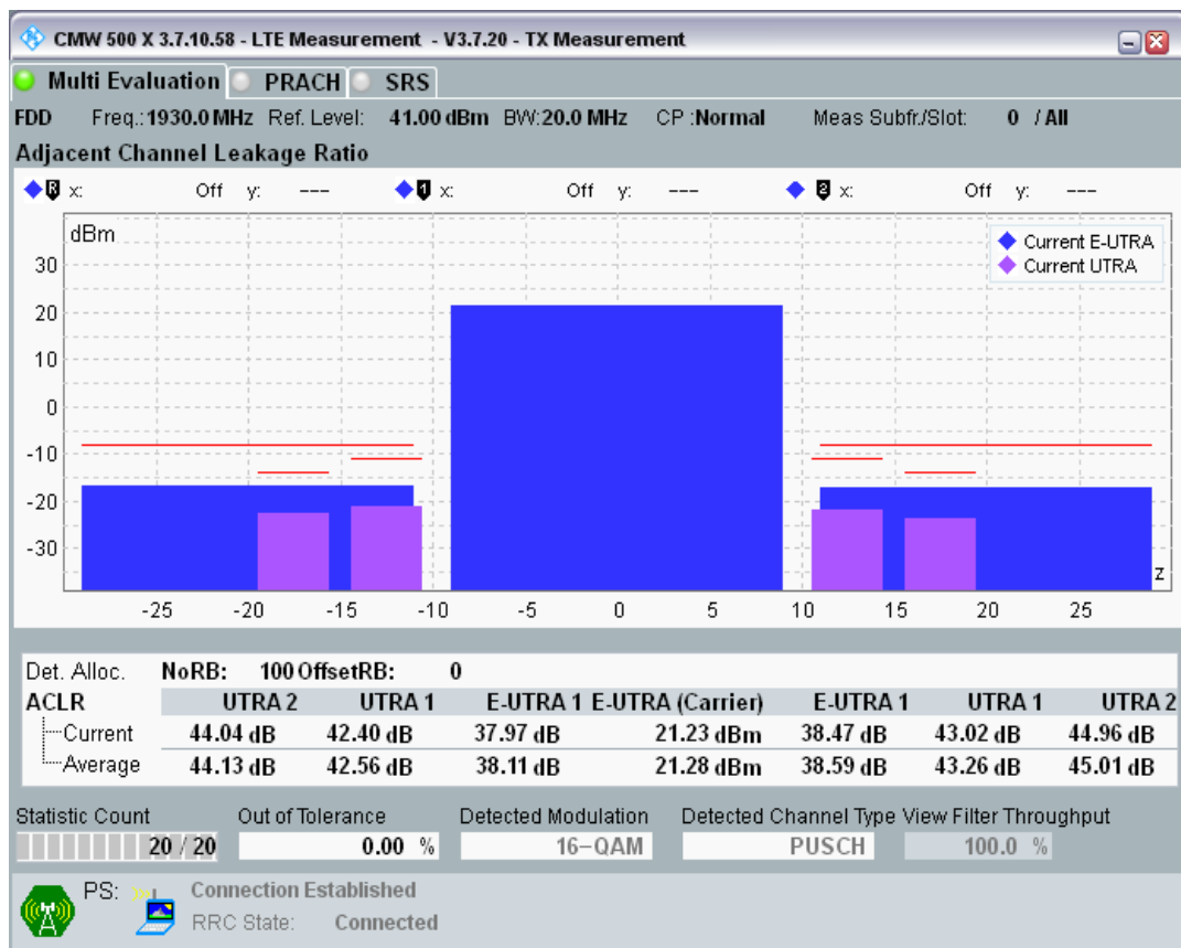
Band1 QAM16 BW=20MHz Channel=18100 RB Size=18 Position=#0.png
