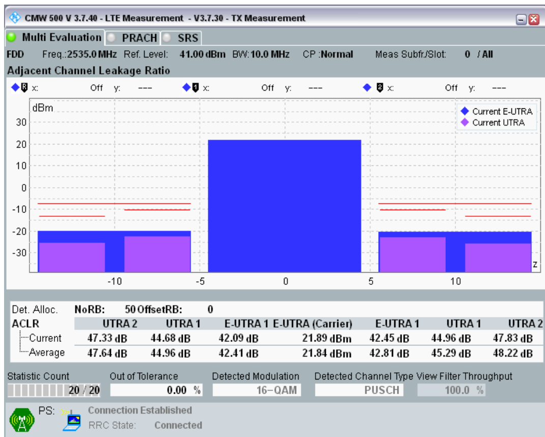
Band7 QAM16 BW=10MHz Channel=21400 RB Size=12 Position=#0.png
