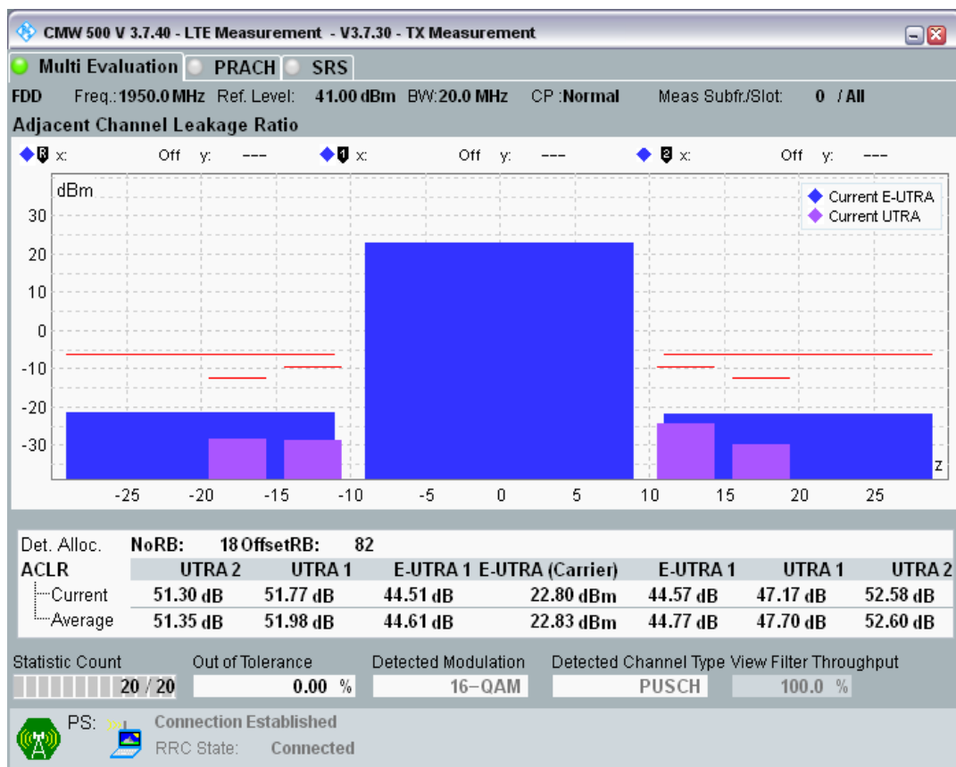
Band1 QAM16 BW=20MHz Channel=18500 RB Size=100 Position=#0.png
