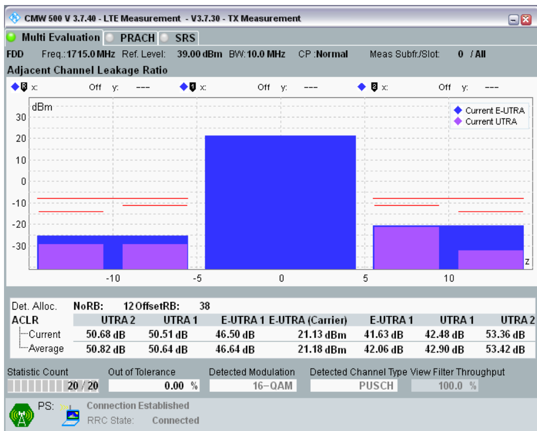
Band3 QAM16 BW=10MHz Channel=19250 RB Size=50 Position=#0.png
