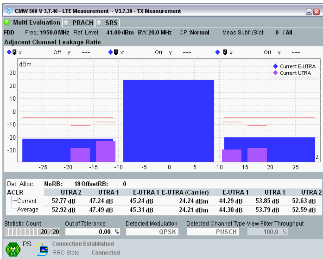
Band1 QPSK BW=20MHz Channel=18300 RB Size=18 Position=#Max.png
