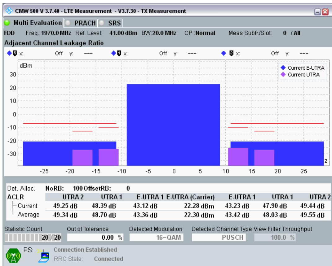
Band1 QAM16 BW=20MHz Channel=18500 RB Size=18 Position=#0.png
