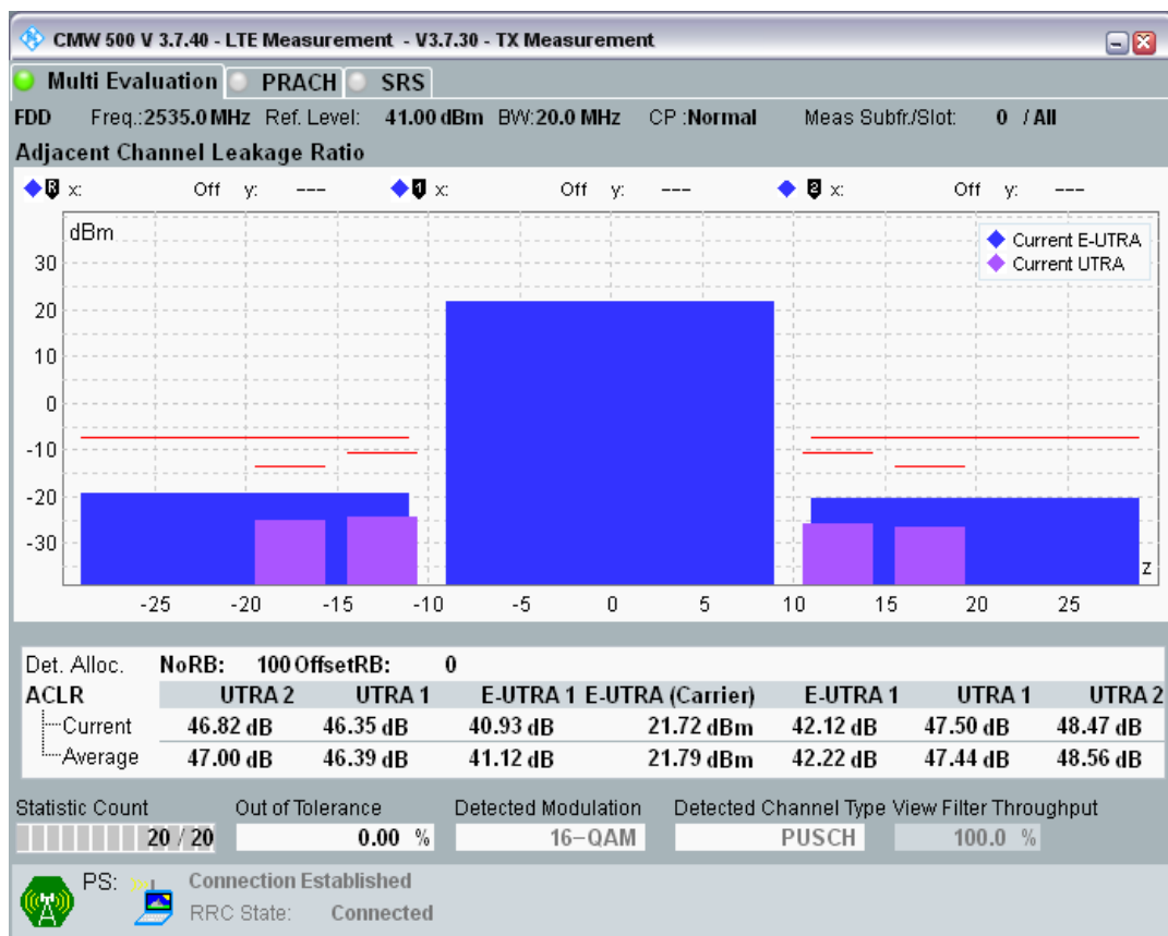
Band7 QAM16 BW=20MHz Channel=21100 RB Size=18 Position=#0.png
