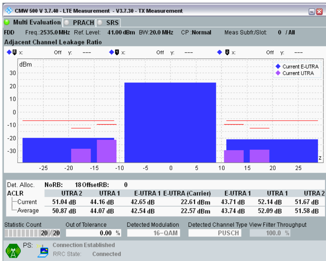
Band7 QAM16 BW=20MHz Channel=21100 RB Size=18 Position=#Max.png
