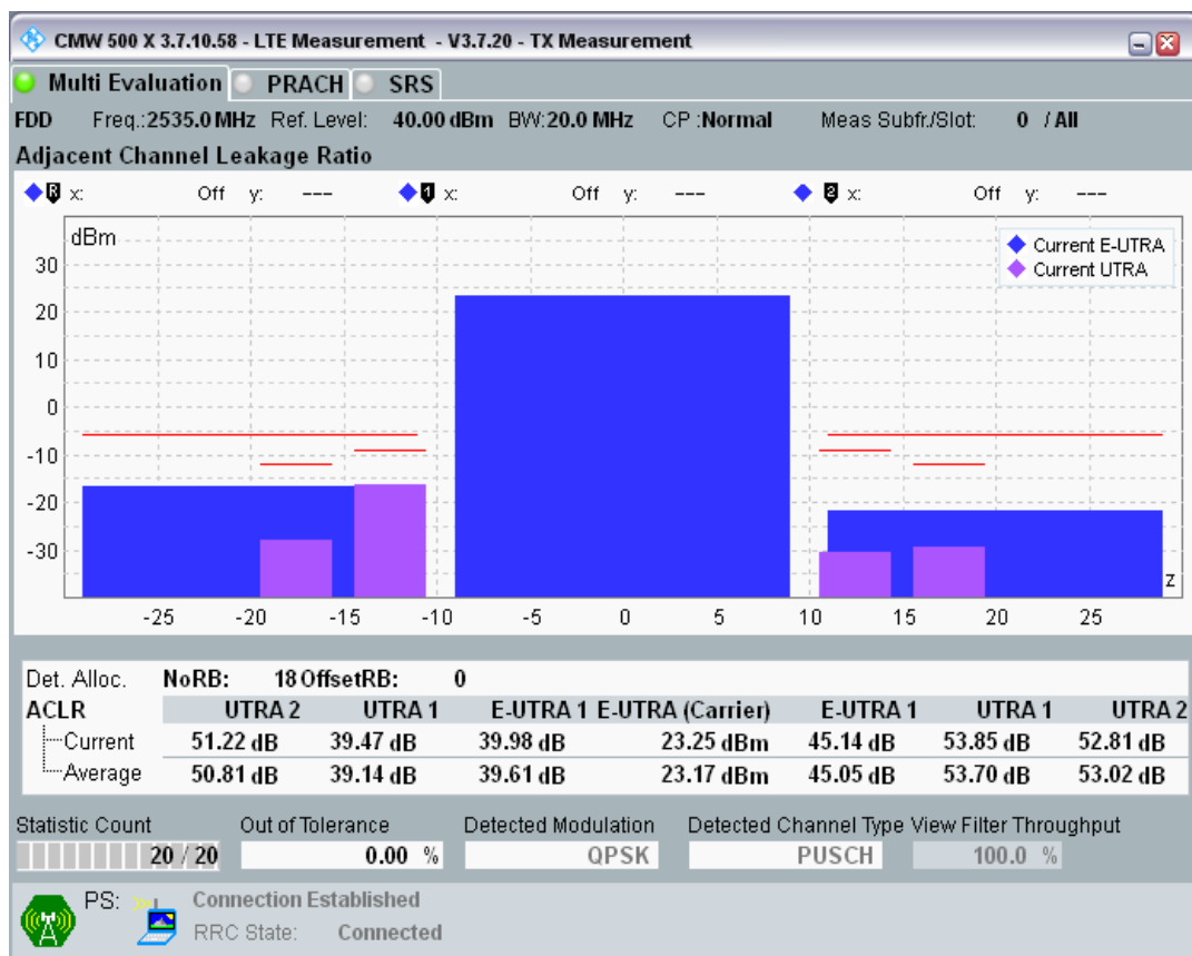
Band7 QPSK BW=20MHz Channel=21100 RB Size=18 Position=#Max.png
