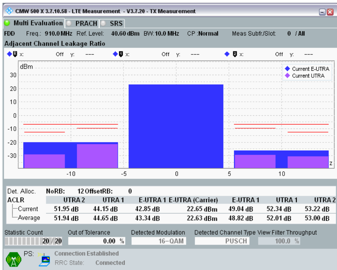
Band8 QAM16 BW=10MHz Channel=21750 RB Size=12 Position=#Max.png
