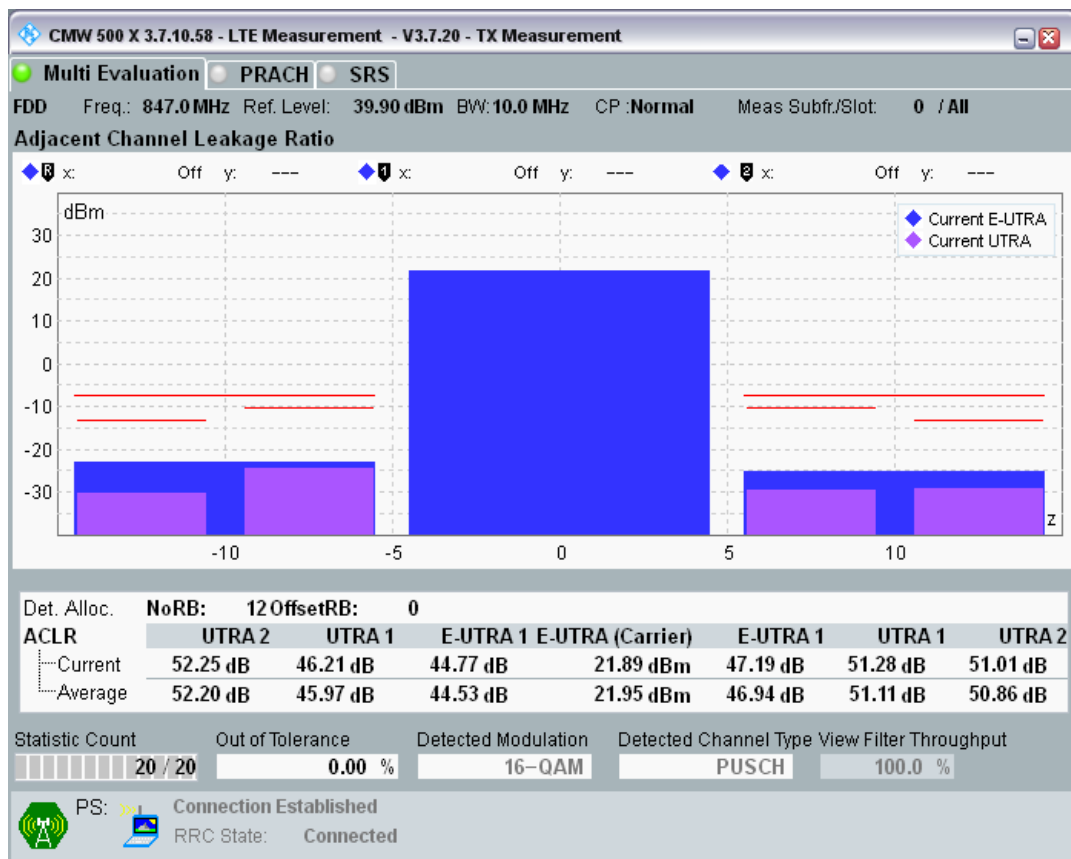
Band20 QAM16 BW=10MHz Channel=24300 RB Size=12 Position=#Max.png
