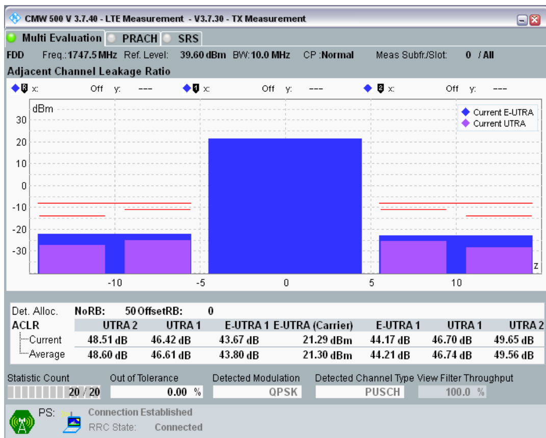
Band3 QPSK BW=10MHz Channel=19900 RB Size=12 Position=#0.png
