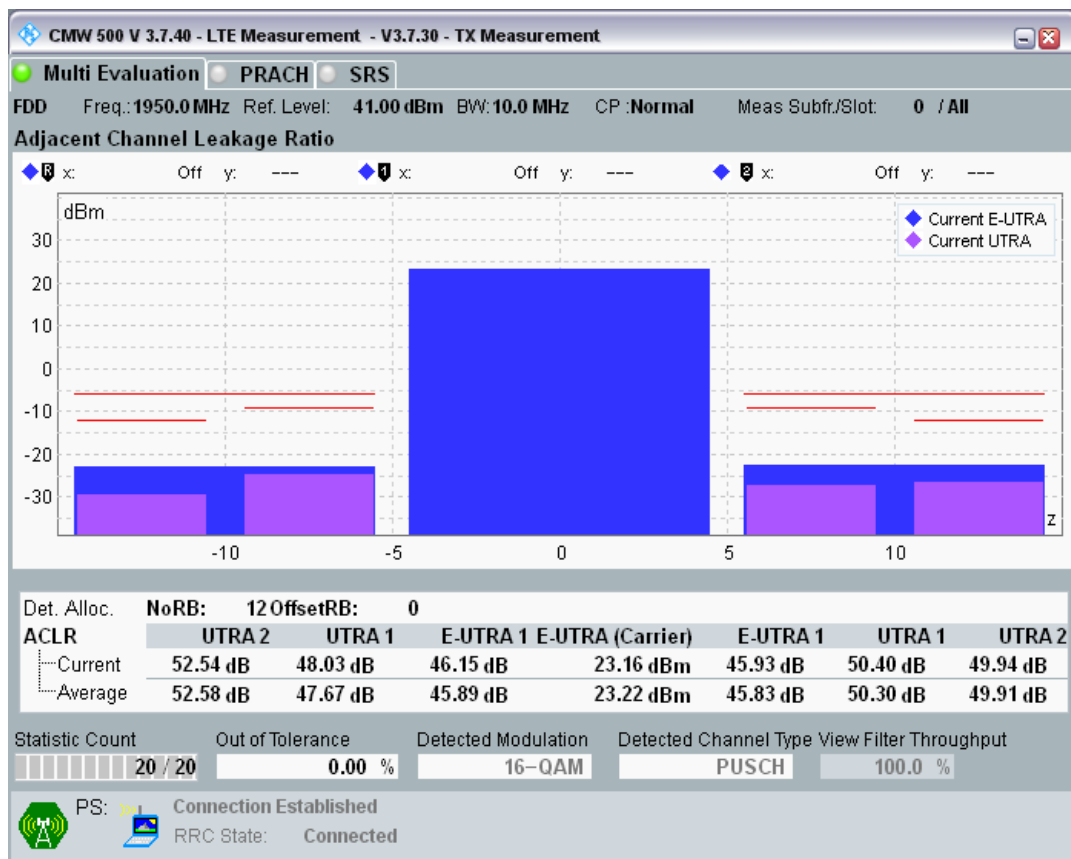
Band1 QAM16 BW=10MHz Channel=18300 RB Size=12 Position=#Max.png
