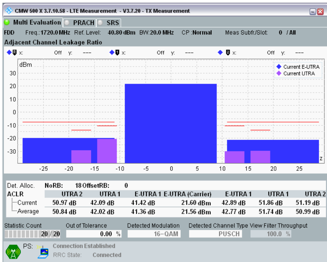
Band3 QAM16 BW=20MHz Channel=19300 RB Size=18 Position=#Max.png
