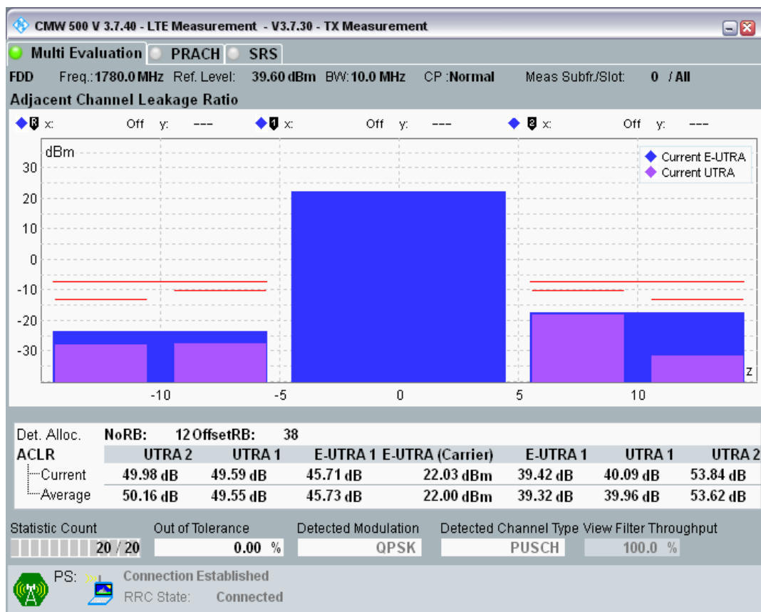
Band3 QPSK BW=10MHz Channel=19900 RB Size=50 Position=#0.png
