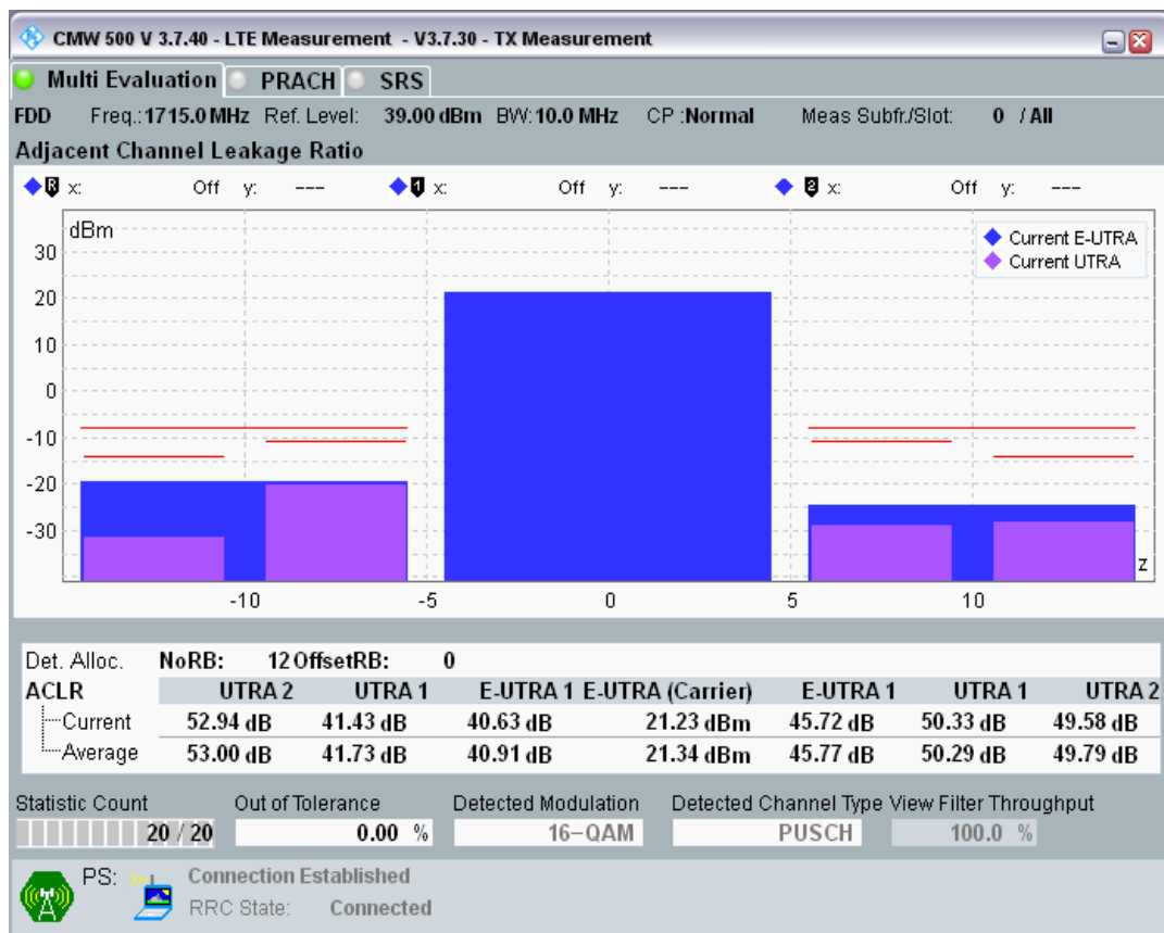
Band3 QAM16 BW=10MHz Channel=19250 RB Size=12 Position=#Max.png
