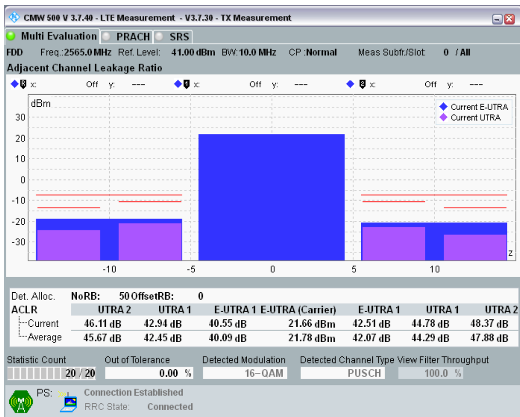
Band7 QAM16 BW=20MHz Channel=20850 RB Size=100 Position=#0.png
