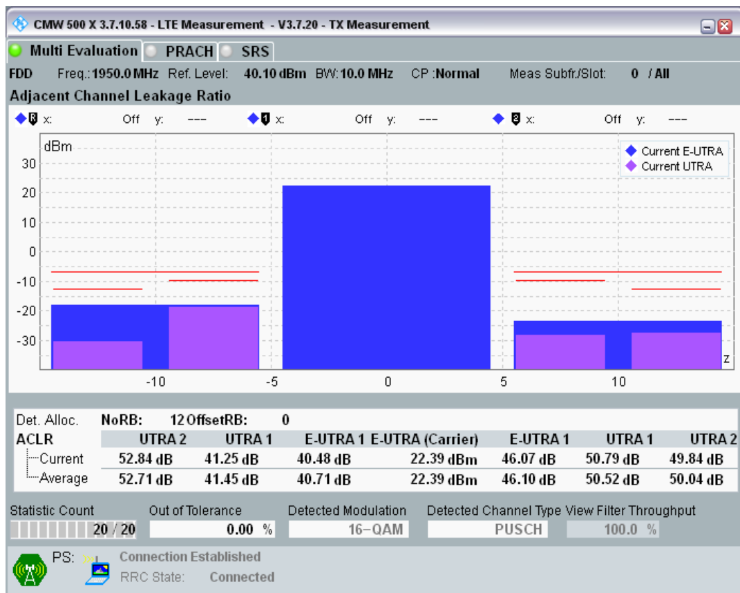
Band1 QAM16 BW=10MHz Channel=18300 RB Size=12 Position=#Max.png
