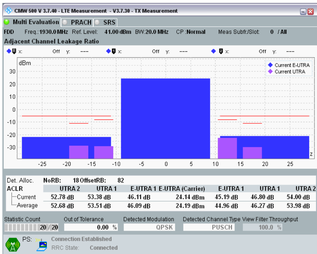
Band1 QPSK BW=20MHz Channel=18300 RB Size=100 Position=#0.png
