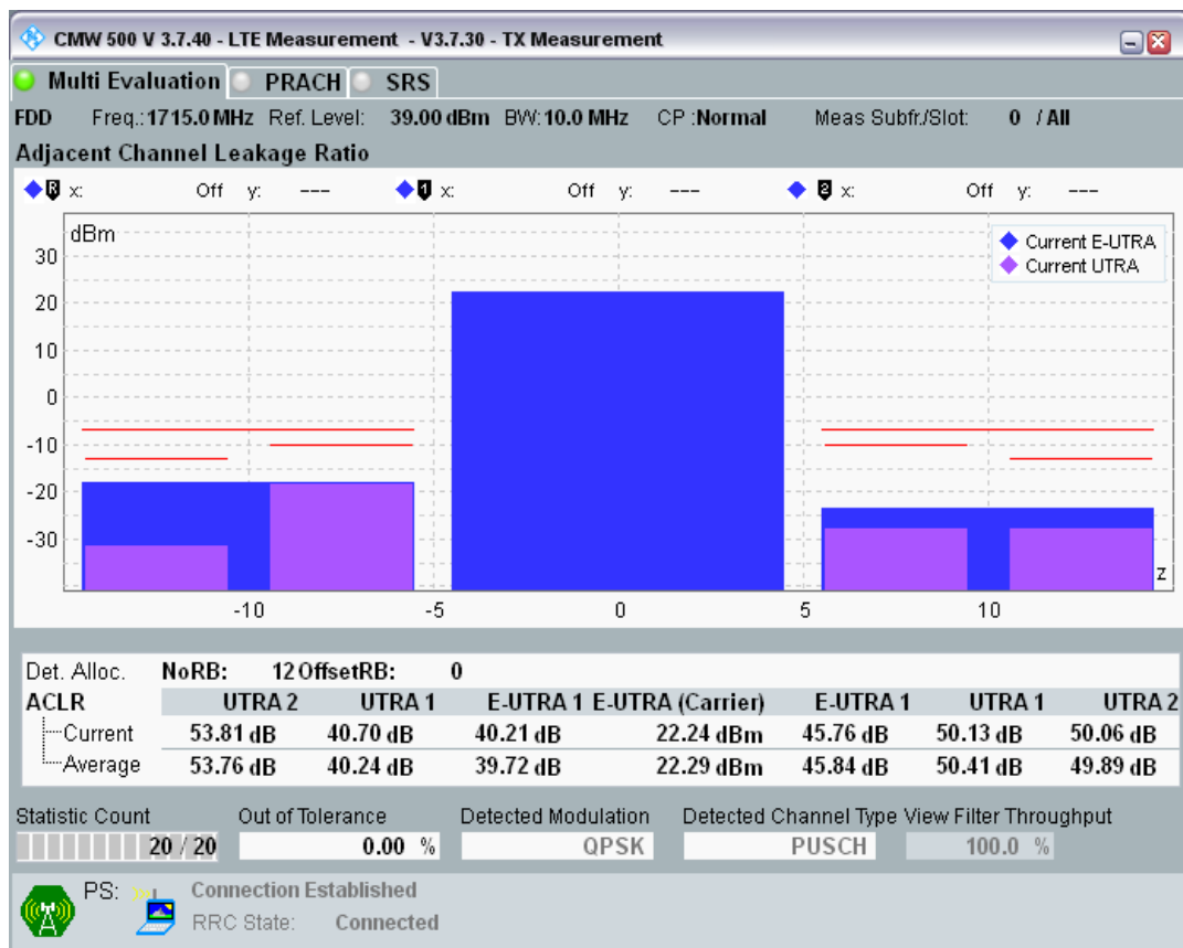
Band3 QPSK BW=10MHz Channel=19250 RB Size=12 Position=#Max.png
