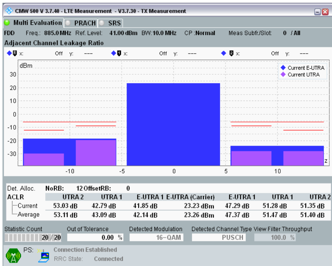
Band8 QAM16 BW=10MHz Channel=21500 RB Size=12 Position=#Max.png
