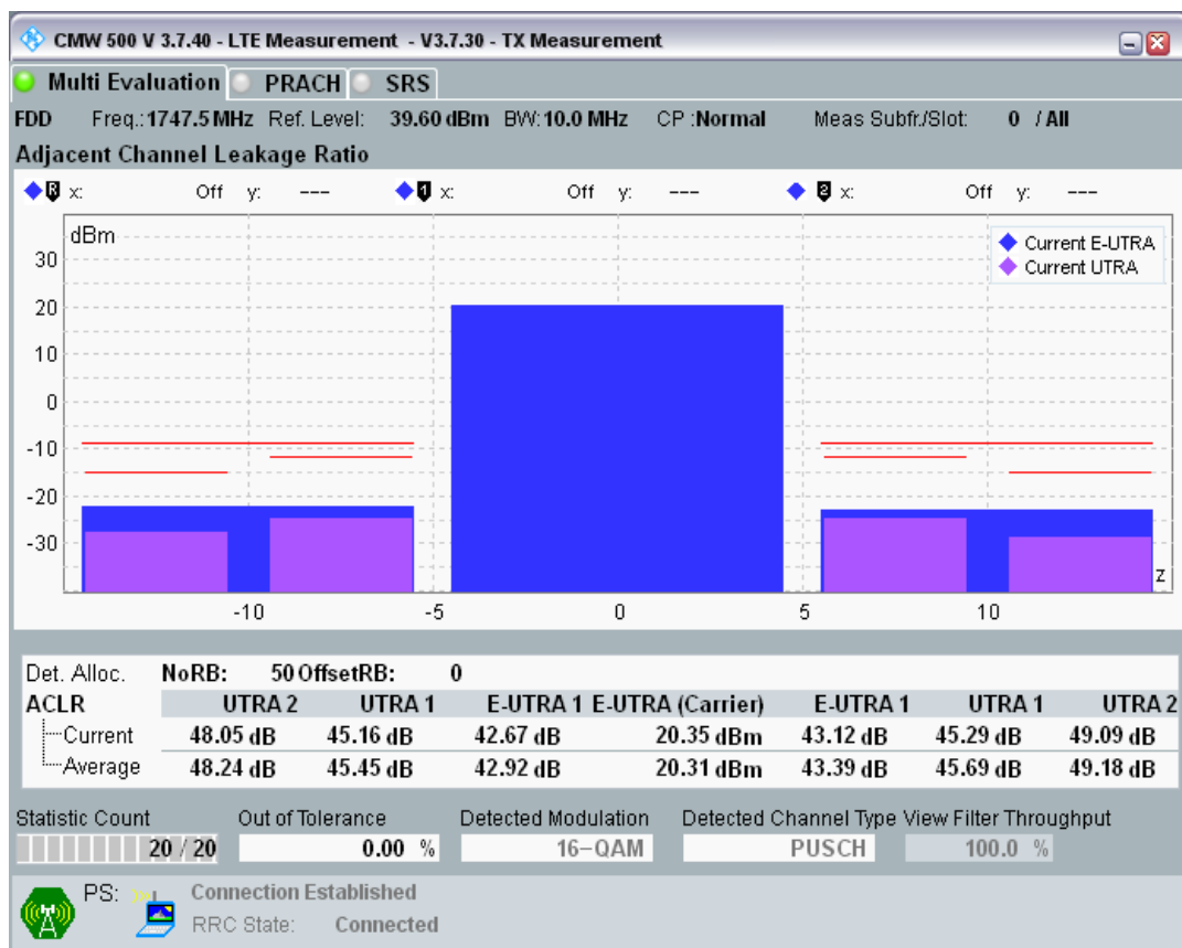
Band3 QAM16 BW=10MHz Channel=19900 RB Size=12 Position=#0.png
