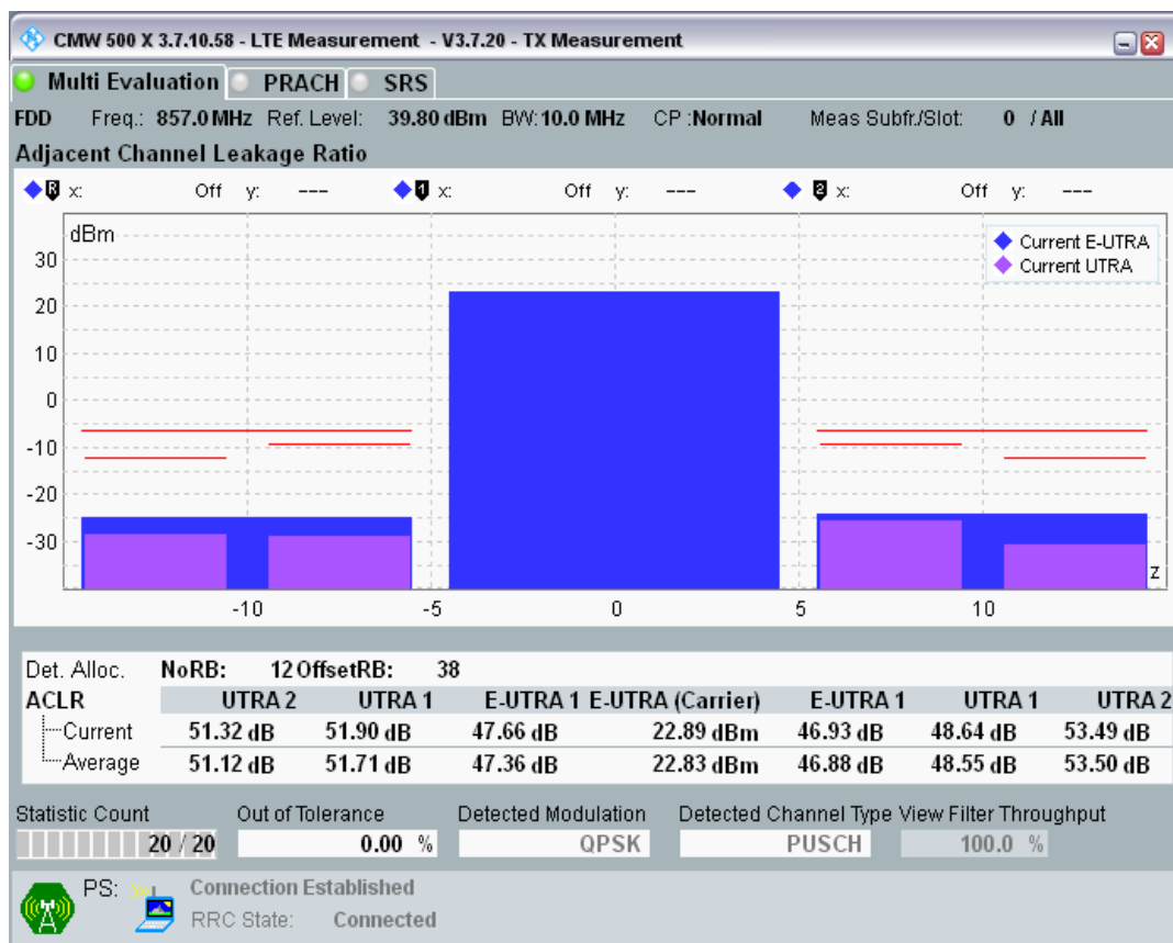
Band20 QPSK BW=10MHz Channel=24400 RB Size=50 Position=#0.png
