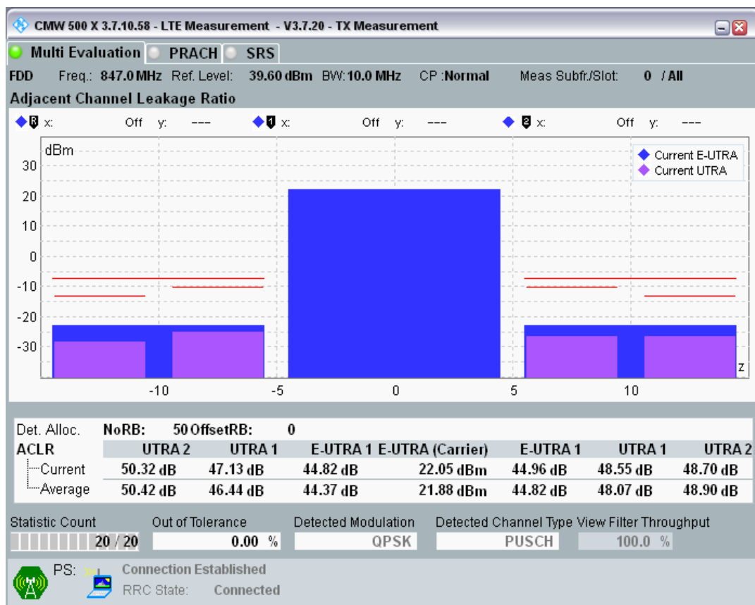
Band20 QPSK BW=10MHz Channel=24400 RB Size=12 Position=#0.png
