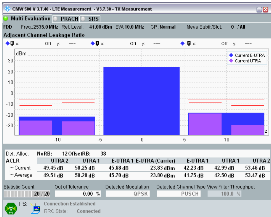
Band7 QPSK BW=10MHz Channel=21100 RB Size=50 Position=#0.png
