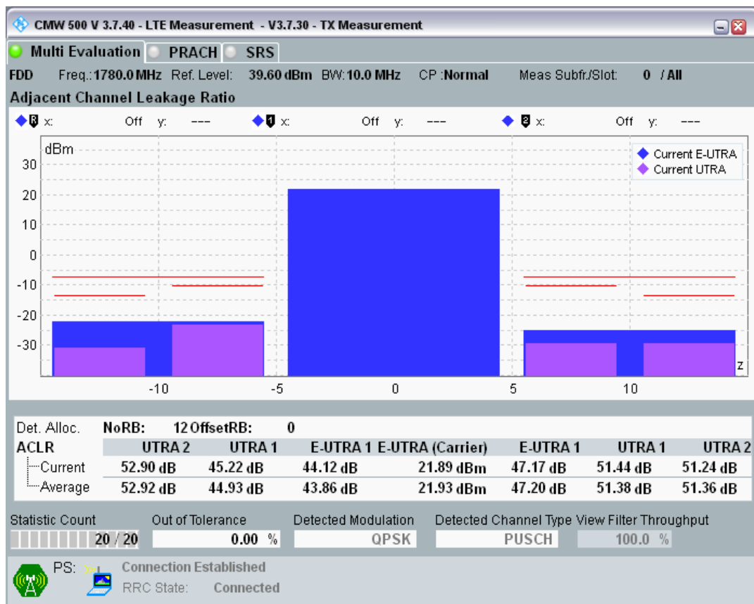
Band3 QPSK BW=10MHz Channel=19900 RB Size=12 Position=#Max.png
