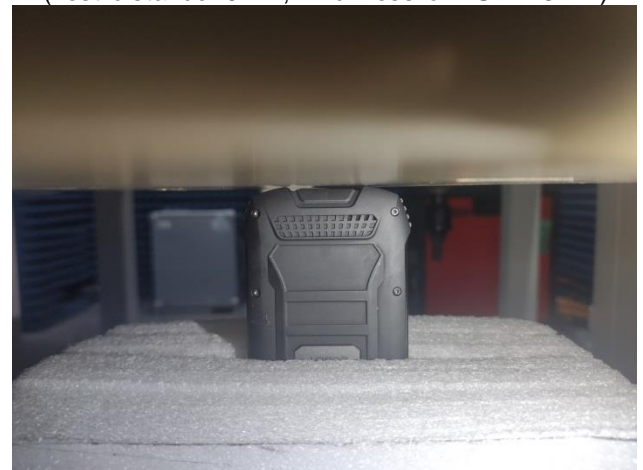
Limb – Bottom (Test distance: 0mm, Thickness of DUT: 13mm)
