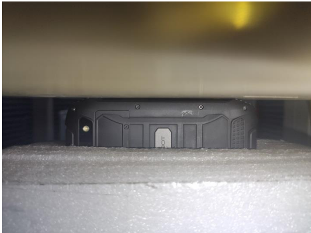
Limb – Left (Test distance: 0mm, Thickness of DUT: 13mm)
