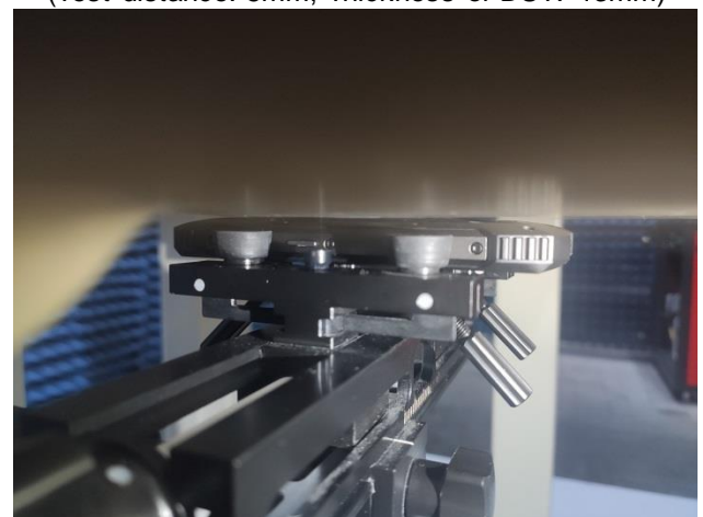
Limb – Back (Test distance: 0mm, Thickness of DUT: 13mm)
