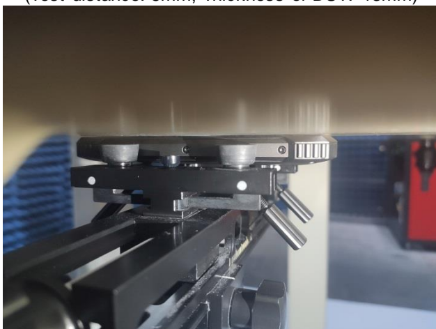
Limb – Front (Test distance: 0mm, Thickness of DUT: 13mm)
