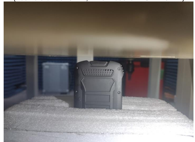
Body worn – Bottom (Test distance: 5mm, Thickness of DUT: 13mm)
