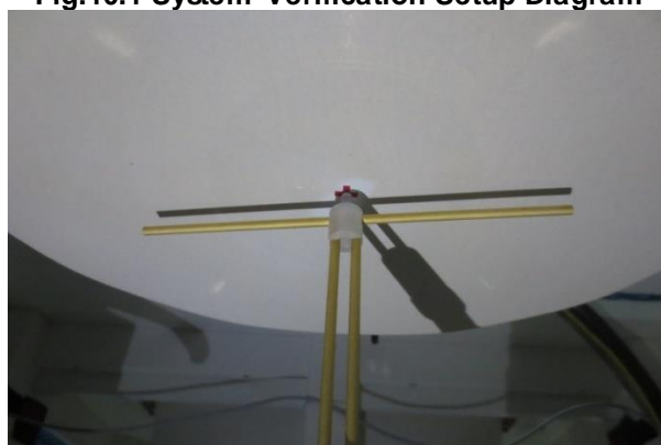
Fig.10.2 Photo of Dipole setup
