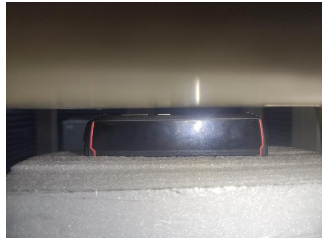
Body worn – Right (Test distance: 5mm, Thickness of DUT: 13mm)
