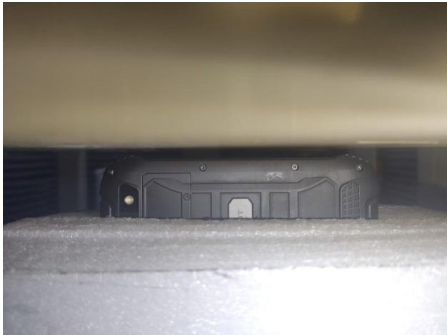
Body worn – Left (Test distance: 5mm, Thickness of DUT: 13mm)
