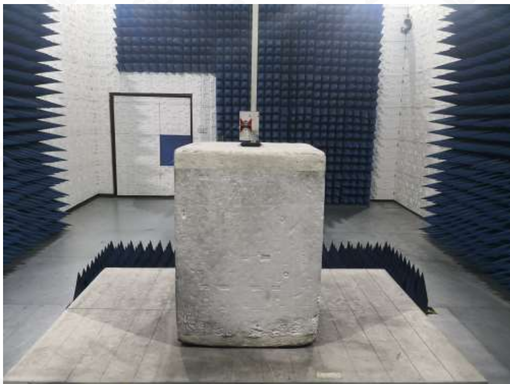
RADIATED SPURIOUS EMISSION ABOVE 1G TEST SETUP
