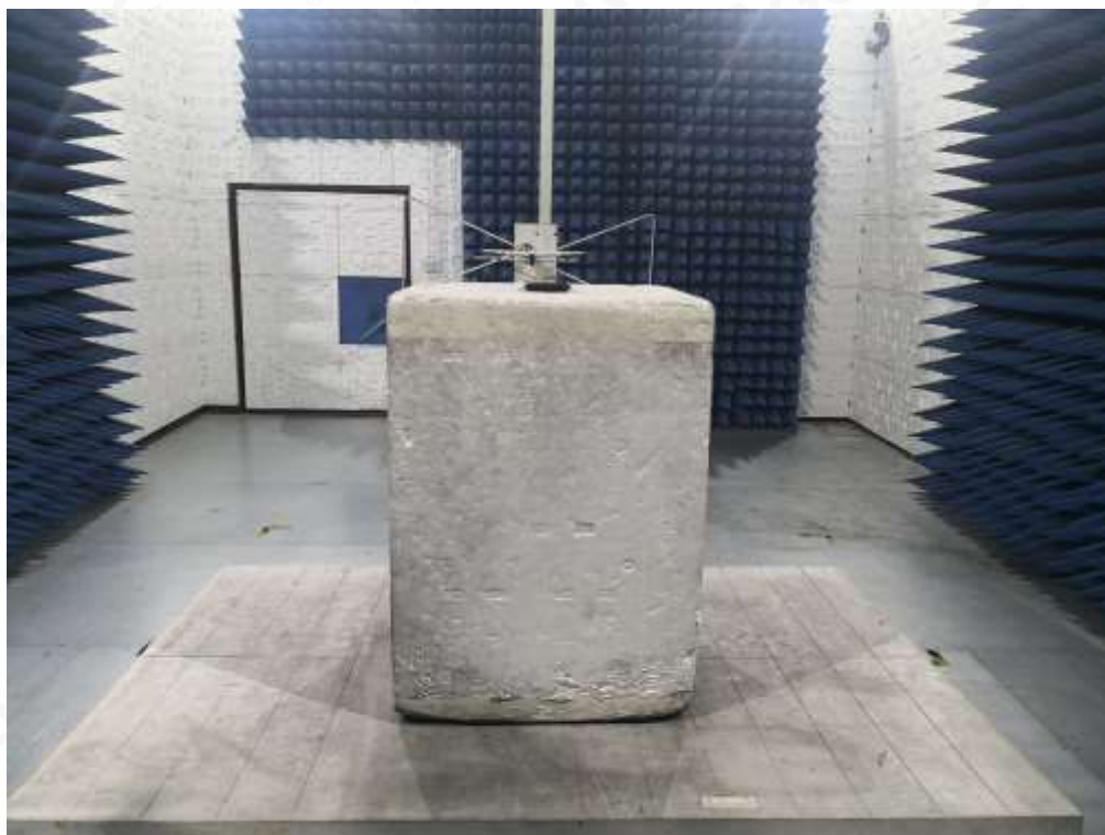
RADIATED SPURIOUS EMISSION ABOVE 1G TEST SETUP
