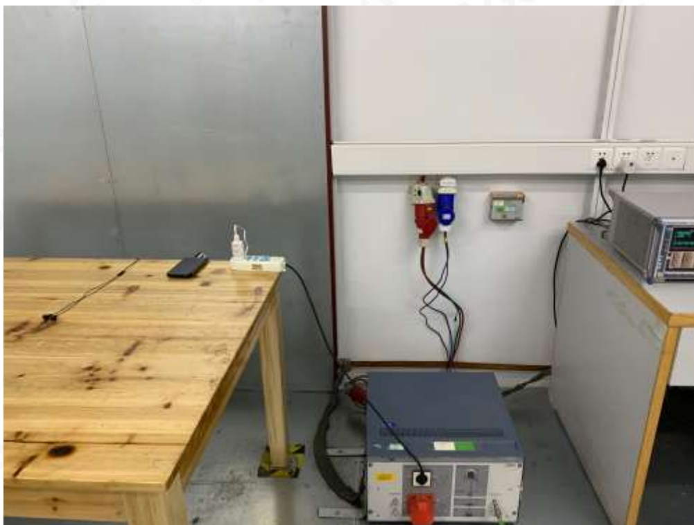
RADIATED EMISSION TEST SETUP
