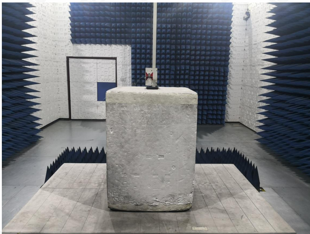
RADIATED SPURIOUS EMISSION ABOVE 1G TEST SETUP
