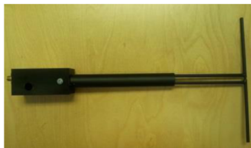
Figure 1 – MVG COMOSAR Validation Dipole
