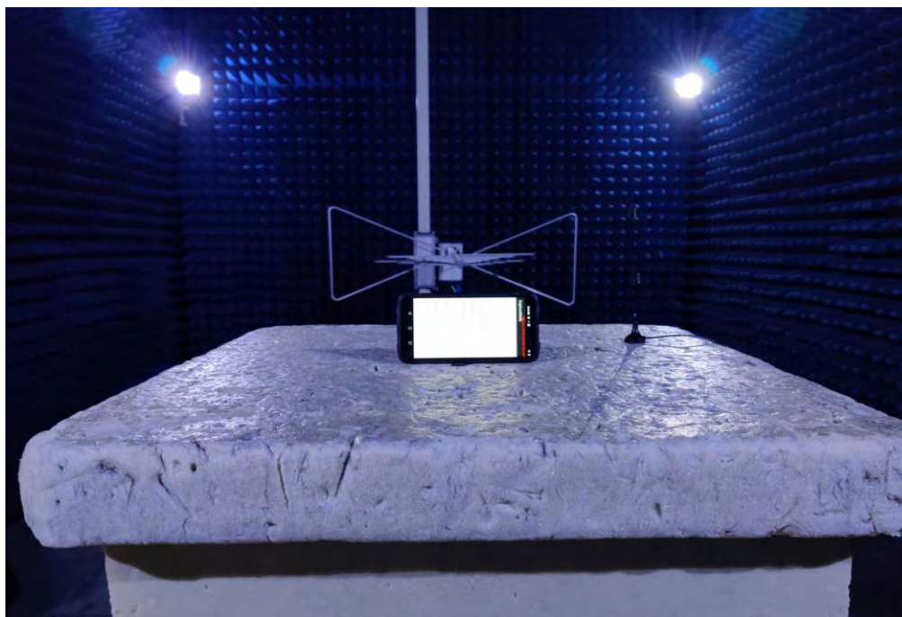
Radiated Spurious Emissions Test View (Above 1GHz)
