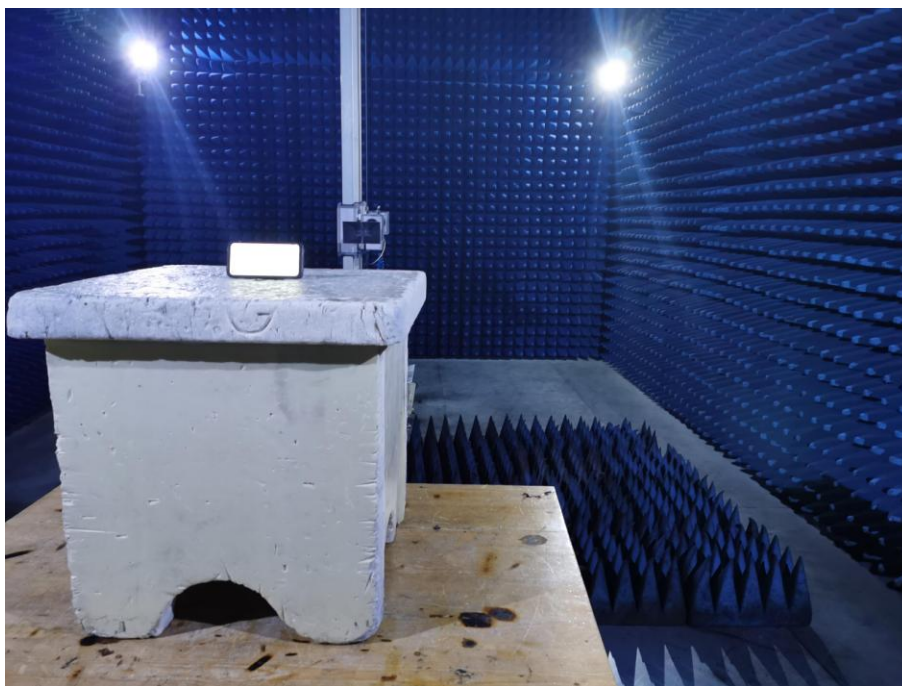
Radiated Spurious Emissions Test View (Above 1GHz)
