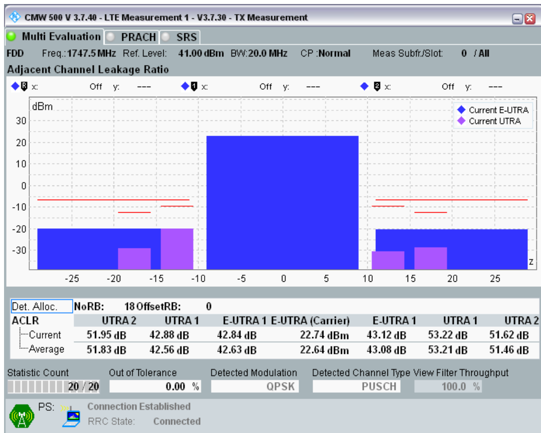
Band3 QPSK BW=20MHz Channel=19575 RB Size=18 Position=#Max
