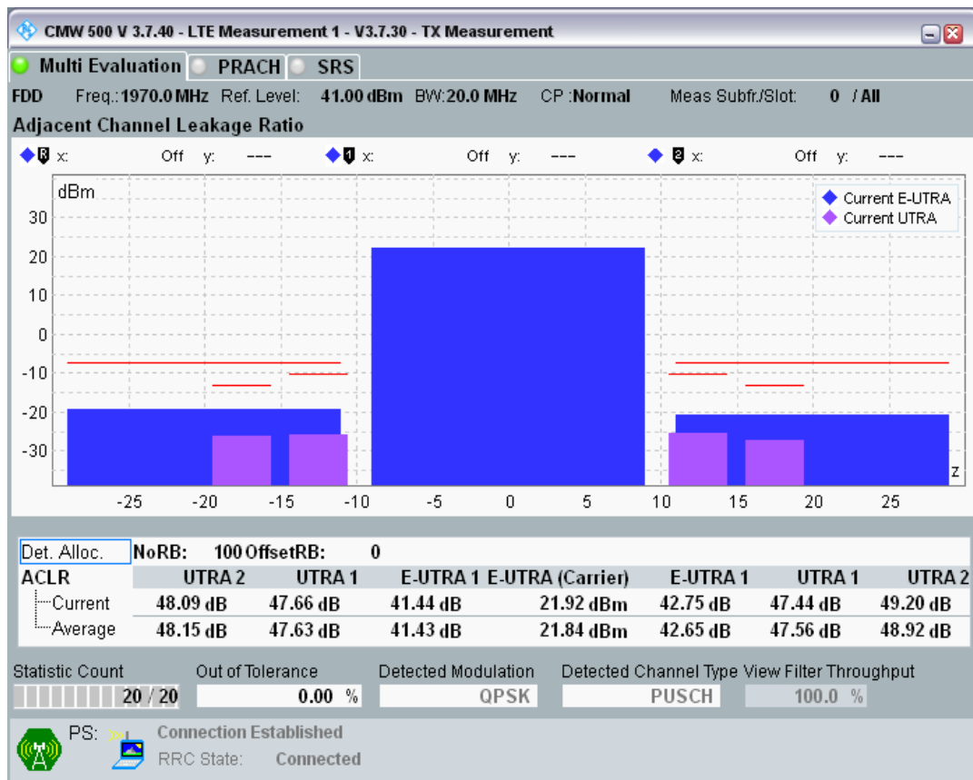
Band1 QAM16 BW=20MHz Channel=18500 RB Size=18 Position=#0
