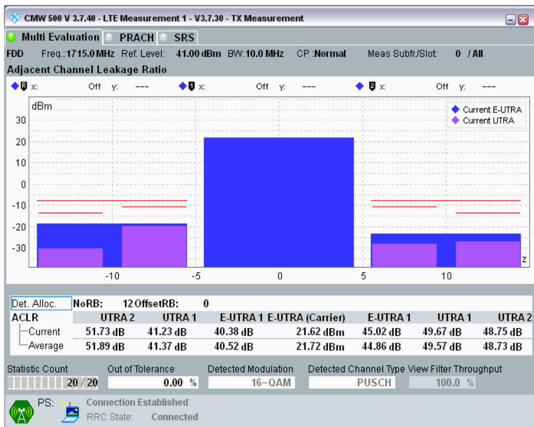
Band3 QAM16 BW=10MHz Channel=19250 RB Size=12 Position=#Max
