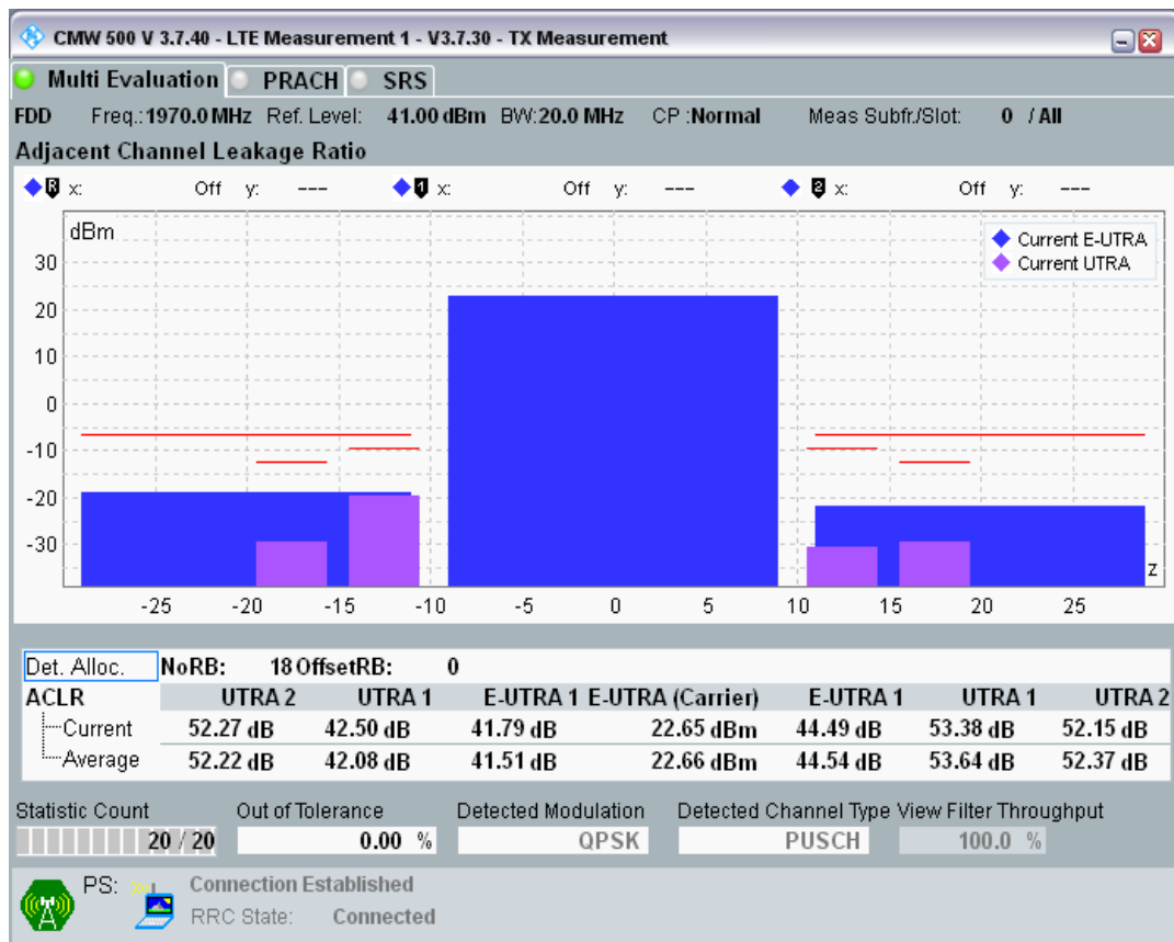
Band1 QPSK BW=20MHz Channel=18500 RB Size=18 Position=#Max
