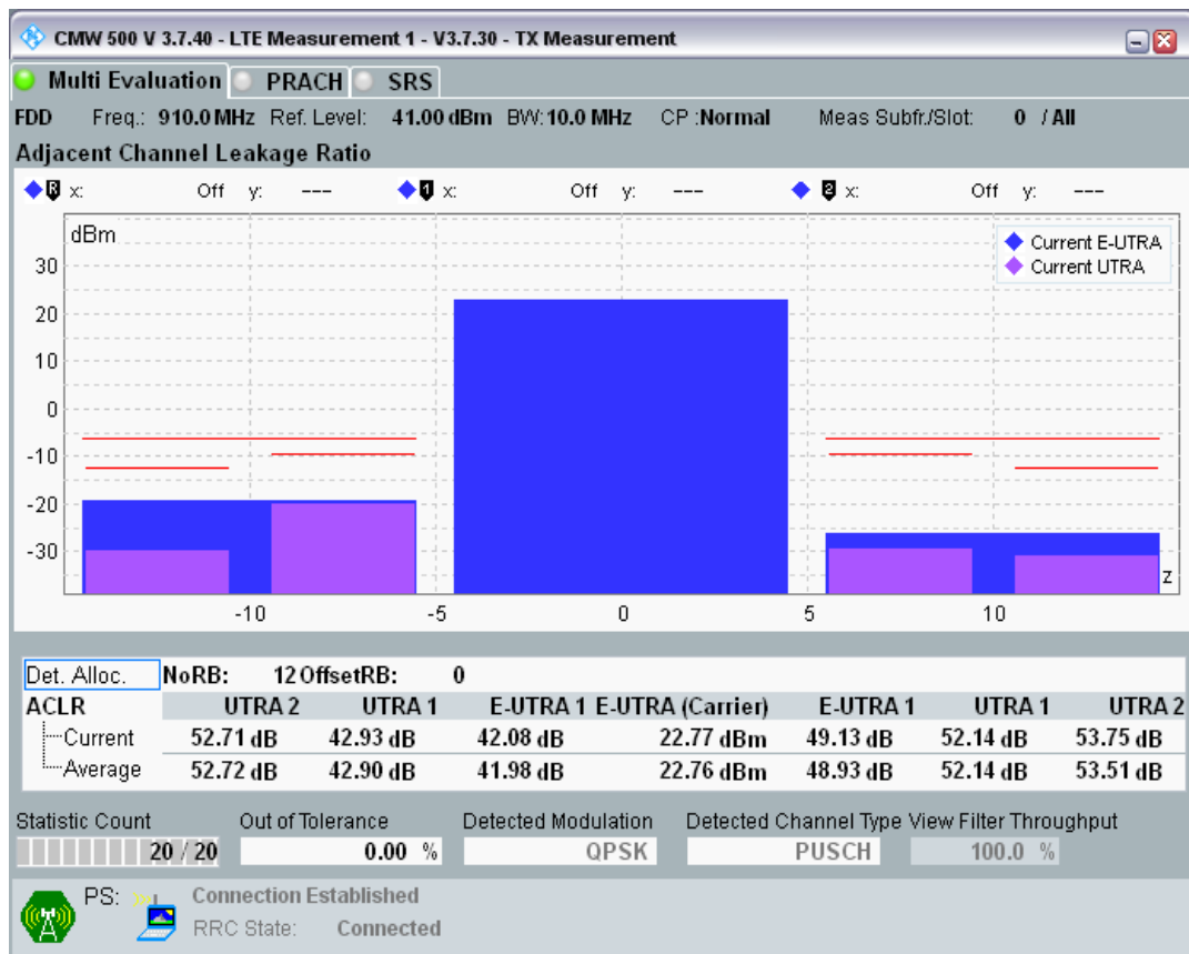
Band8 QPSK BW=10MHz Channel=21750 RB Size=12 Position=#Max
