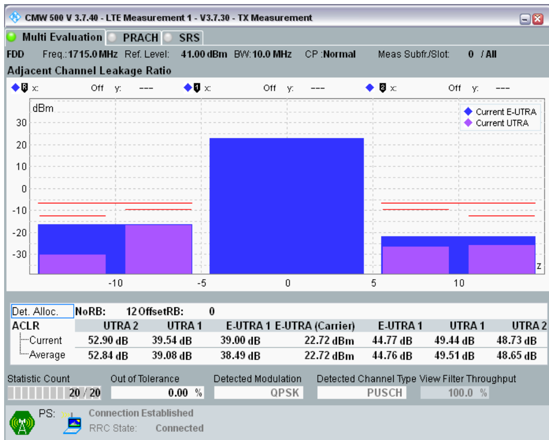
Band3 QPSK BW=10MHz Channel=19250 RB Size=12 Position=#Max
