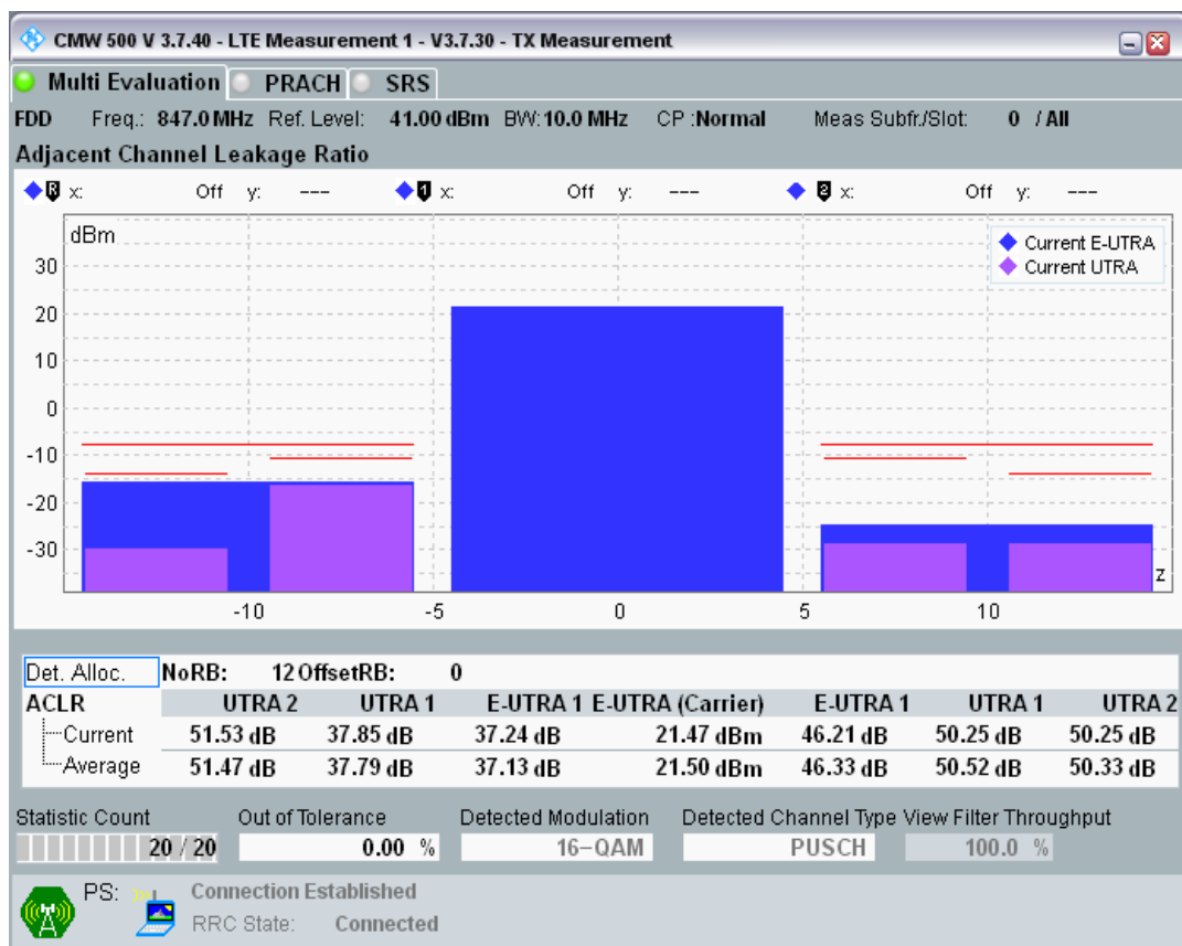
Band20 QAM16 BW=10MHz Channel=24300 RB Size=12 Position=#Max
