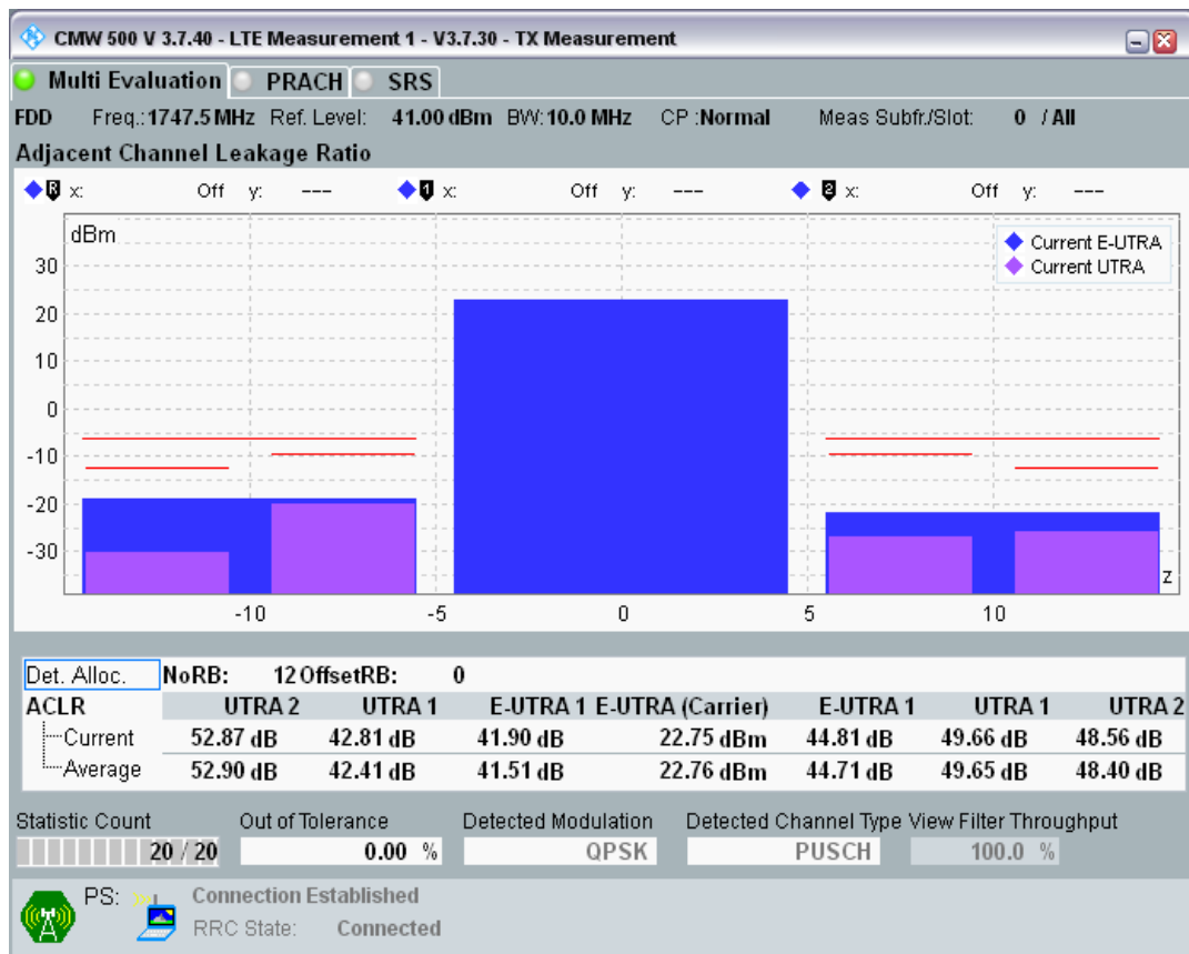
Band3 QPSK BW=10MHz Channel=19575 RB Size=12 Position=#Max
