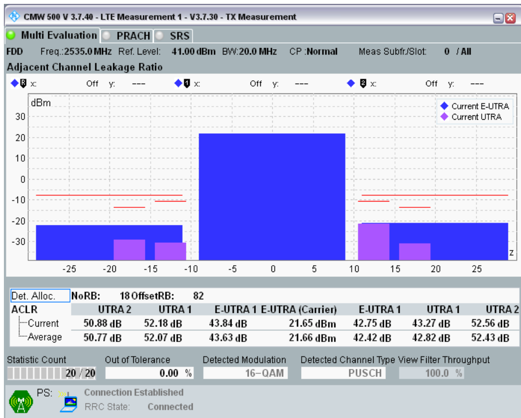
Band7 QAM16 BW=20MHz Channel=21100 RB Size=100 Position=#0
