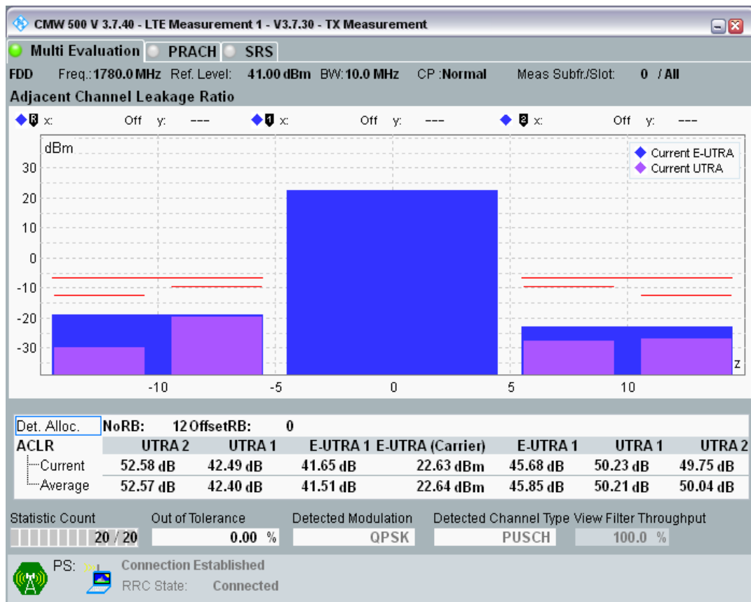
Band3 QPSK BW=10MHz Channel=19900 RB Size=12 Position=#Max
