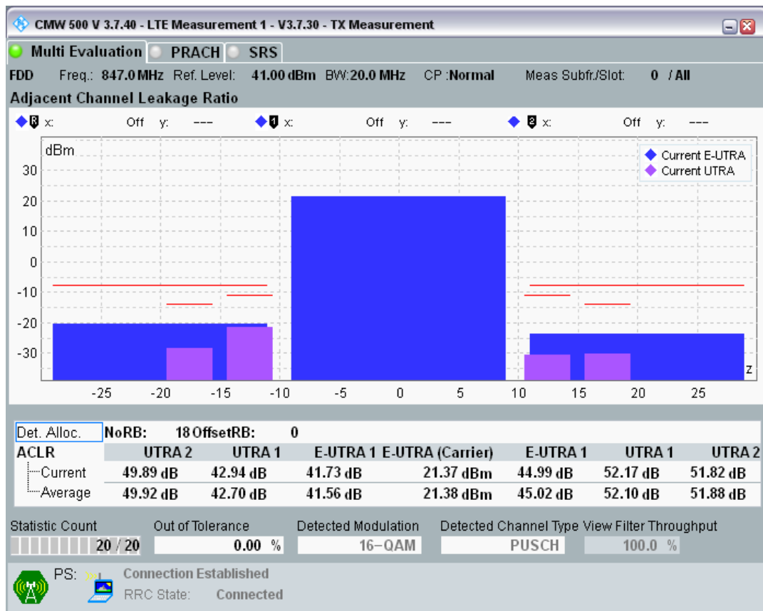
Band20 QAM16 BW=20MHz Channel=24300 RB Size=18 Position=#Max
