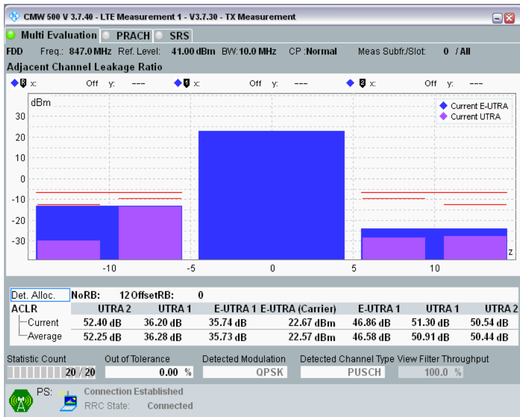
Band20 QPSK BW=10MHz Channel=24300 RB Size=12 Position=#Max
