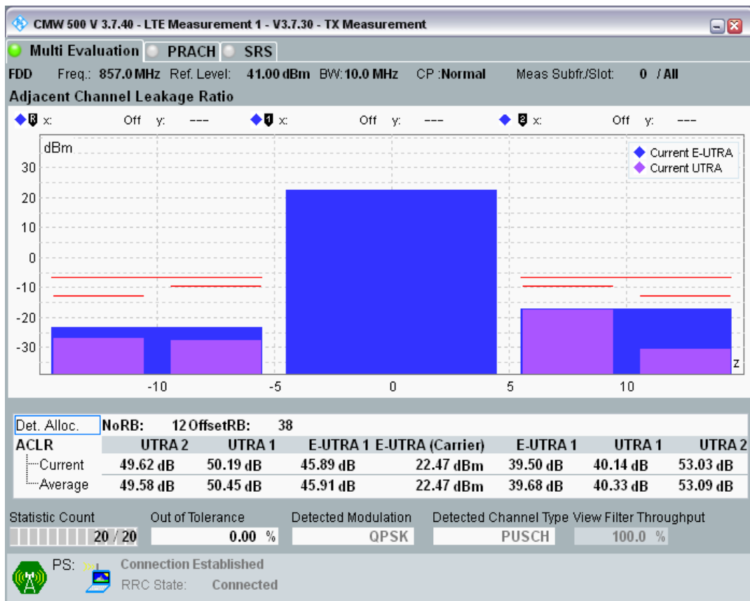
Band20 QPSK BW=10MHz Channel=24400 RB Size=50 Position=#0
