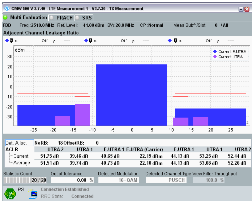
Band7 QAM16 BW=20MHz Channel=20850 RB Size=18 Position=#Max
