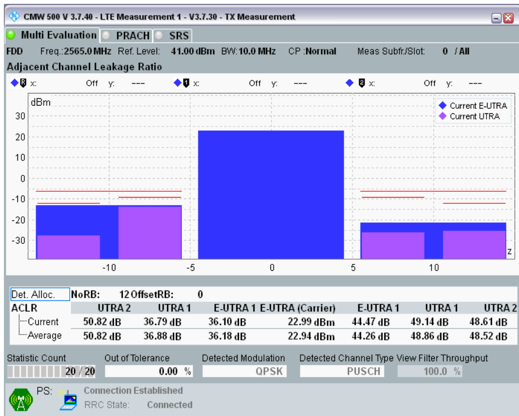
Band7 QPSK BW=10MHz Channel=21400 RB Size=12 Position=#Max
