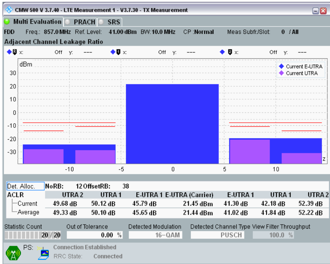
Band20 QAM16 BW=10MHz Channel=24400 RB Size=50 Position=#0
