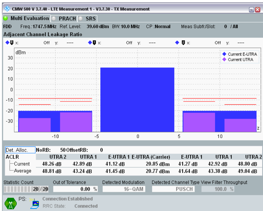
Band3 QPSK BW=10MHz Channel=19900 RB Size=12 Position=#0
