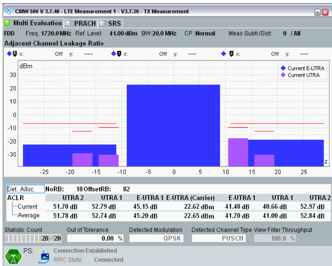
Band3 QPSK BW=20MHz Channel=19300 RB Size=100 Position=#0
