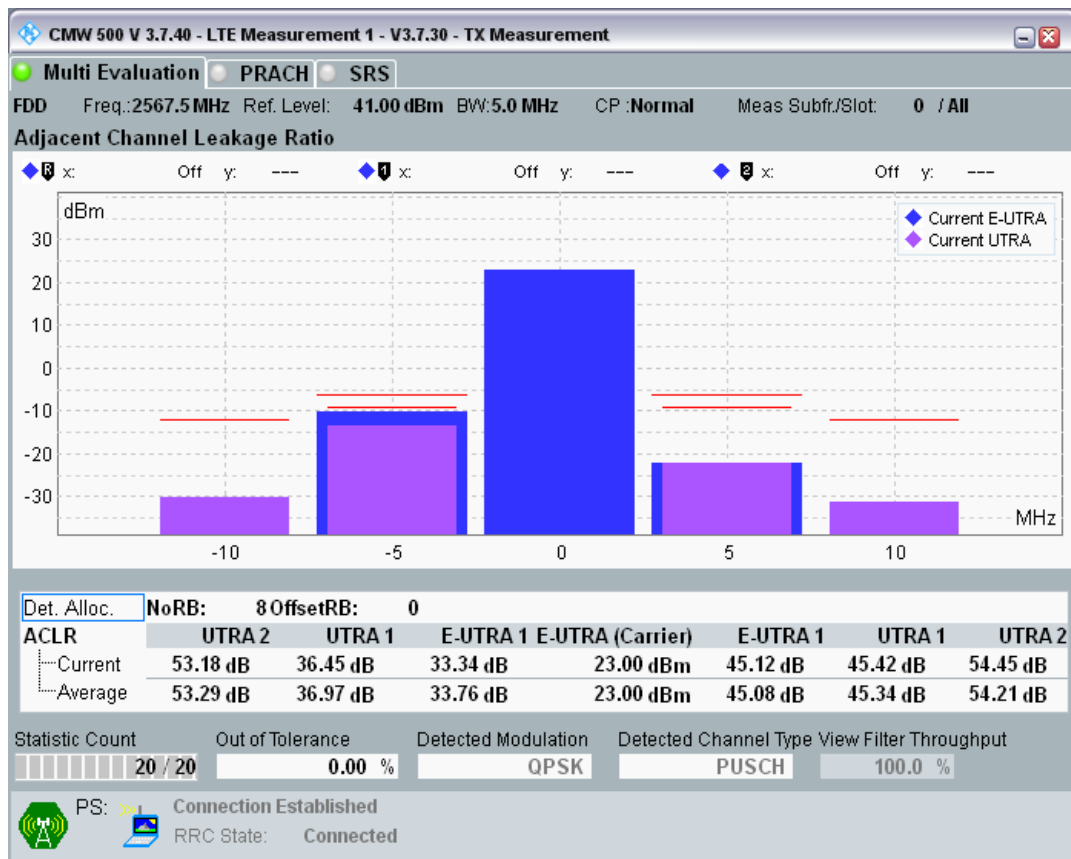
Band7 QPSK BW=5MHz Channel=21425 RB Size=8 Position=#Max
