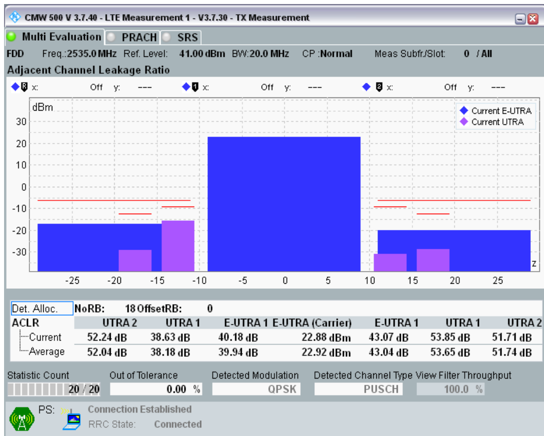
Band7 QPSK BW=20MHz Channel=21100 RB Size=18 Position=#Max
