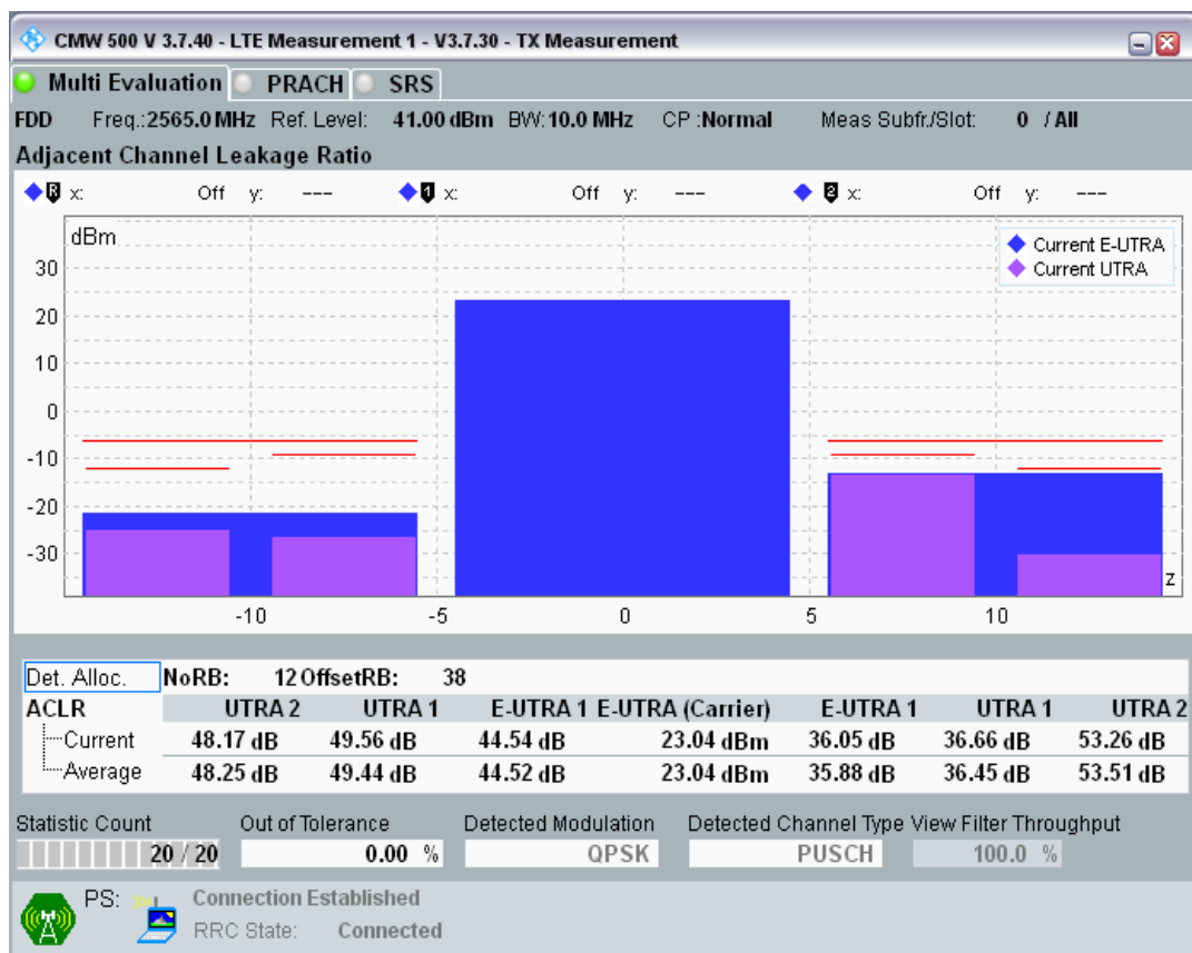
Band7 QPSK BW=10MHz Channel=21400 RB Size=50 Position=#0
