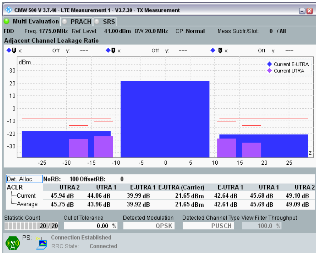
Band3 QAM16 BW=20MHz Channel=19850 RB Size=18 Position=#0
