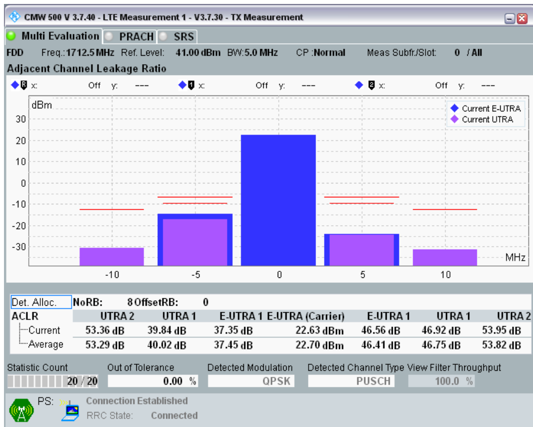
Band3 QPSK BW=5MHz Channel=19225 RB Size=8 Position=#Max
