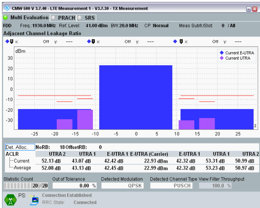
Band1 QPSK BW=20MHz Channel=18100 RB Size=18 Position=#Max
