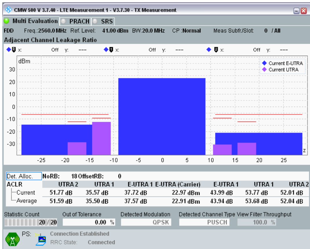
Band7 QPSK BW=20MHz Channel=21350 RB Size=18 Position=#Max
