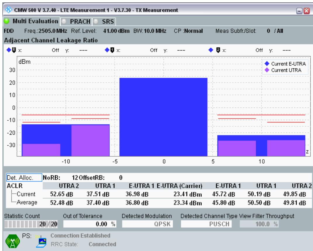
Band7 QPSK BW=10MHz Channel=20800 RB Size=12 Position=#Max
