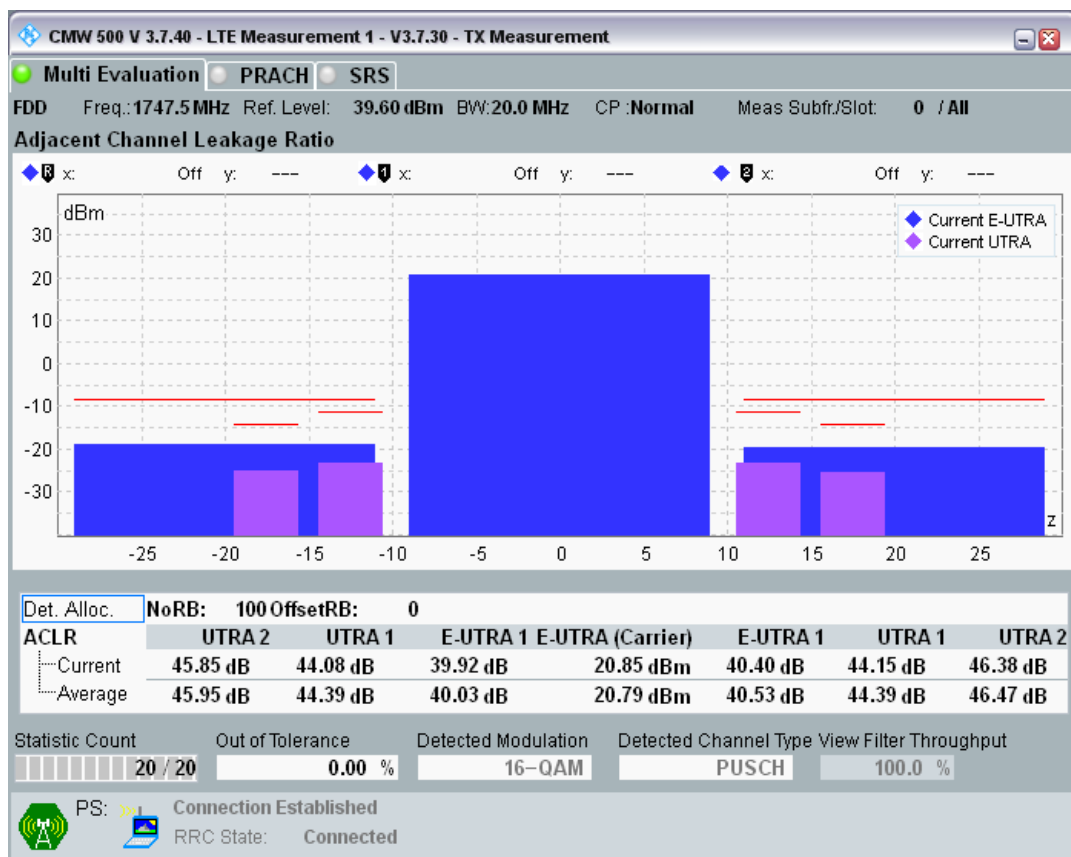
Band3 QPSK BW=20MHz Channel=19850 RB Size=18 Position=#0
