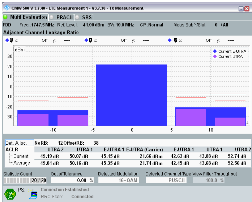
Band3 QAM16 BW=10MHz Channel=19575 RB Size=50 Position=#0
