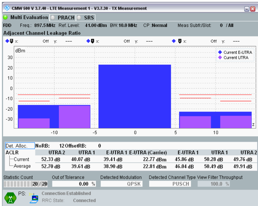
Band8 QPSK BW=10MHz Channel=21625 RB Size=12 Position=#Max
