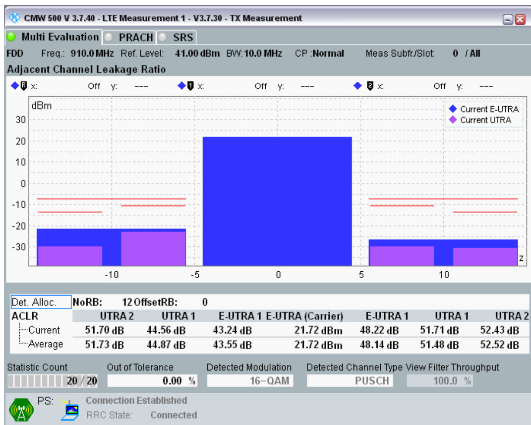
Band8 QAM16 BW=10MHz Channel=21750 RB Size=12 Position=#Max
