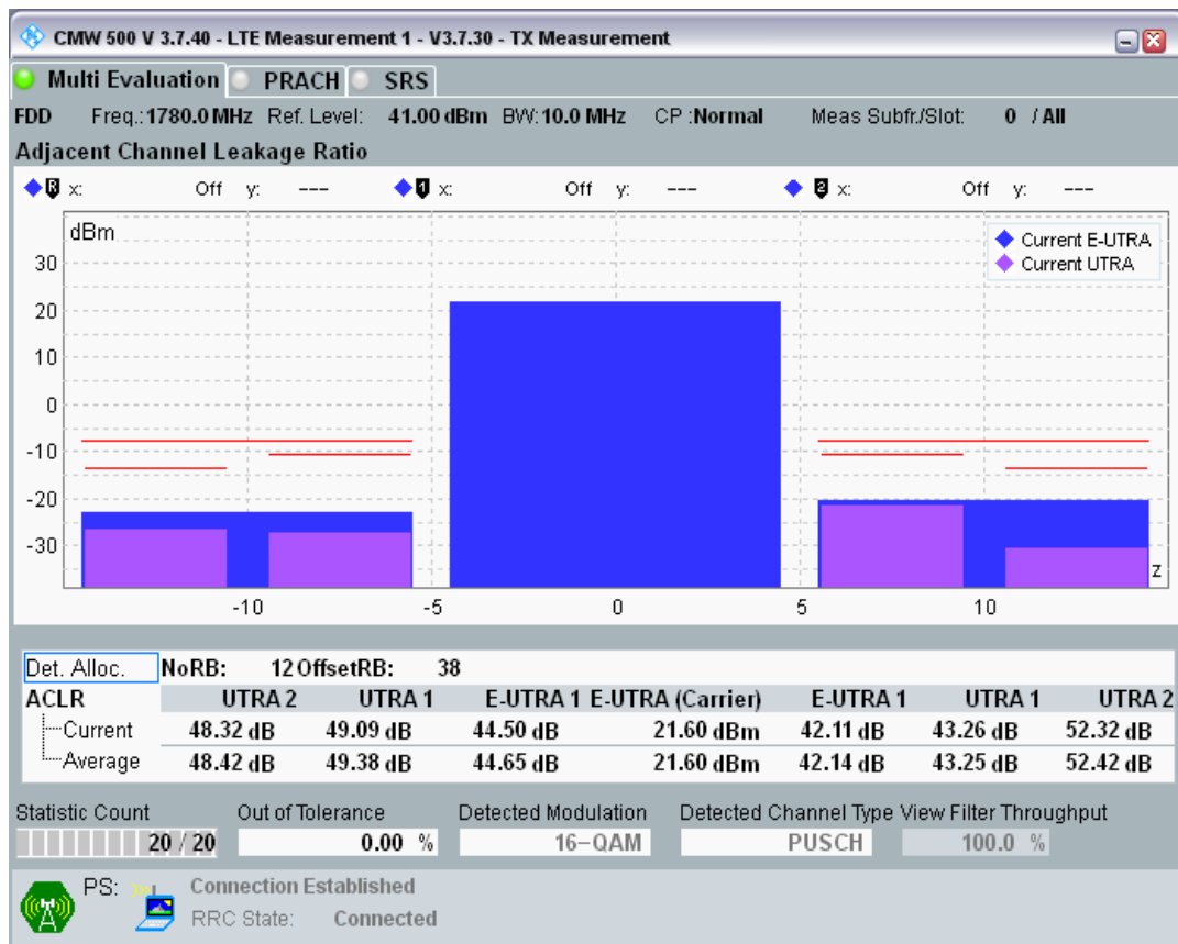
Band3 QAM16 BW=10MHz Channel=19900 RB Size=50 Position=#0
