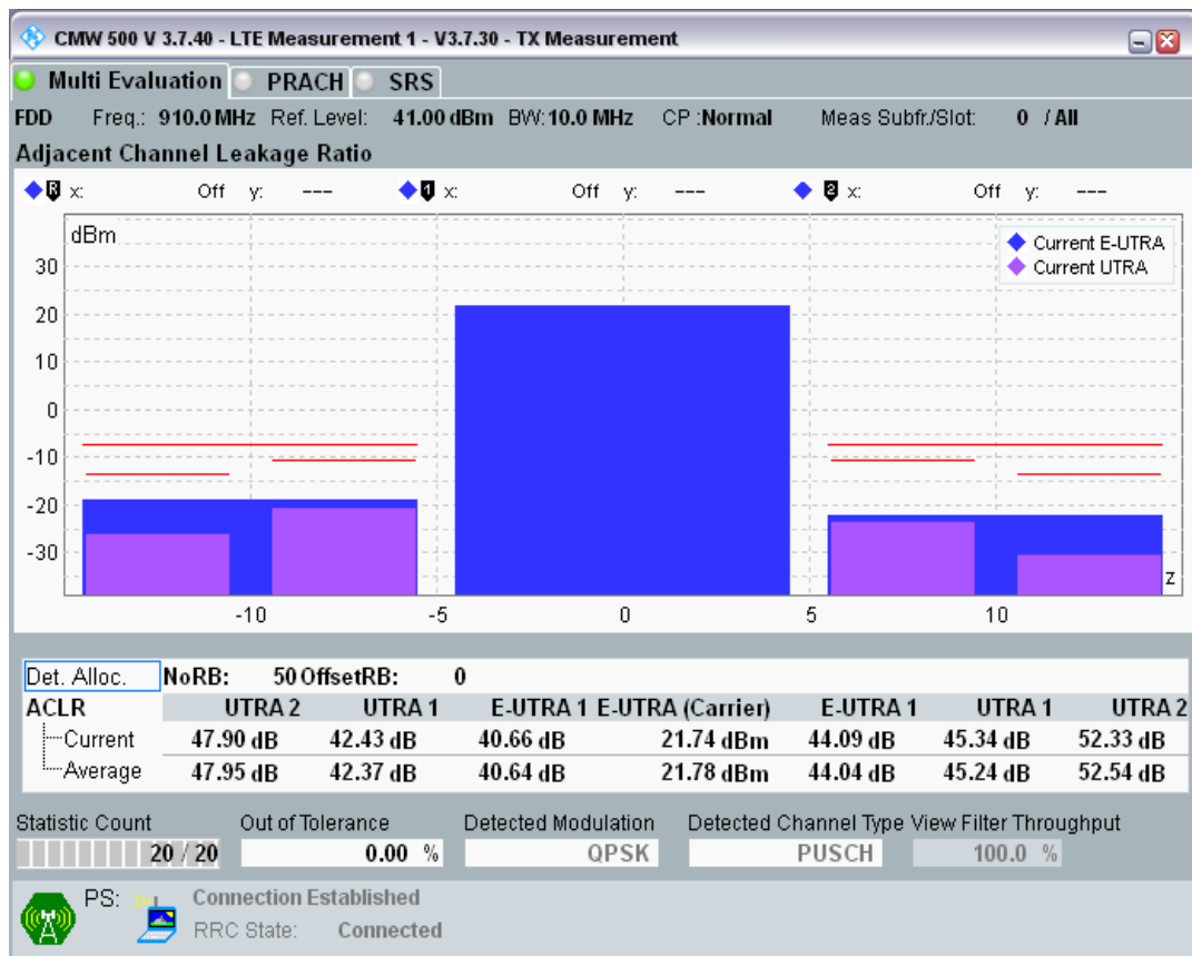
Band8 QAM16 BW=10MHz Channel=21750 RB Size=12 Position=#0
