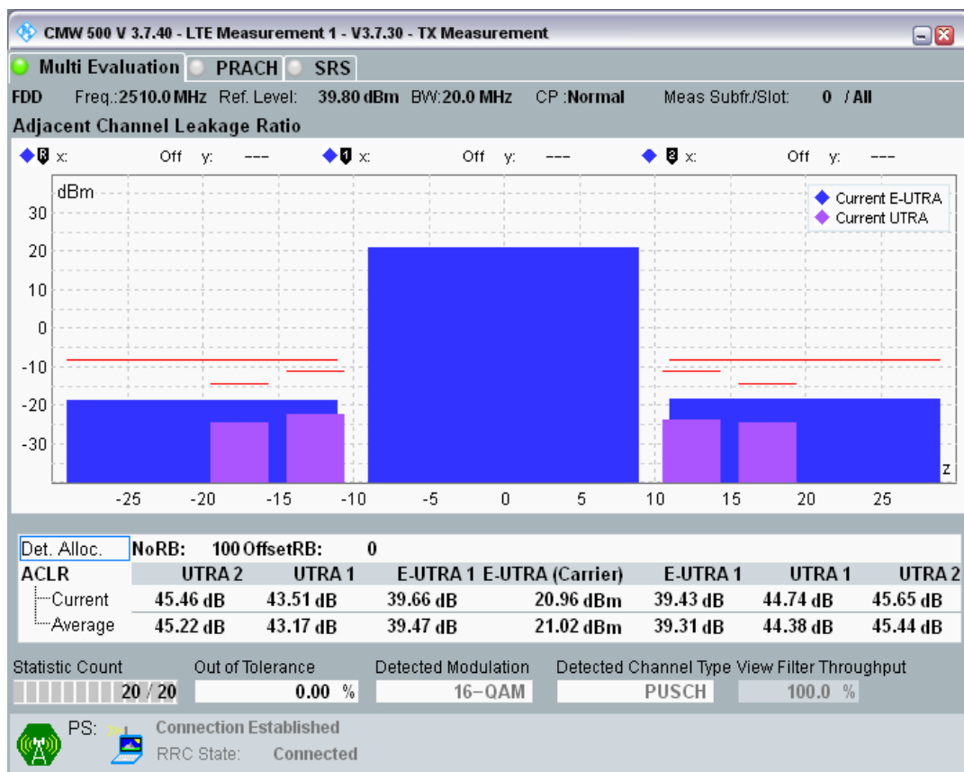
Band7 QPSK BW=20MHz Channel=21100 RB Size=18 Position=#0
