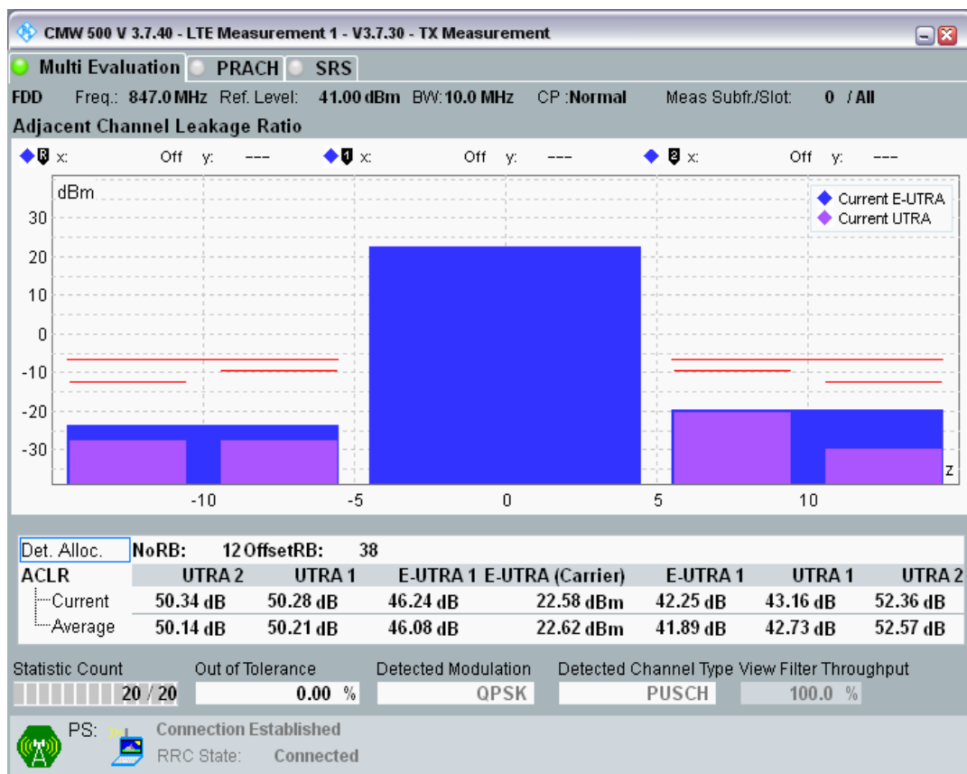
Band20 QPSK BW=10MHz Channel=24300 RB Size=50 Position=#0
