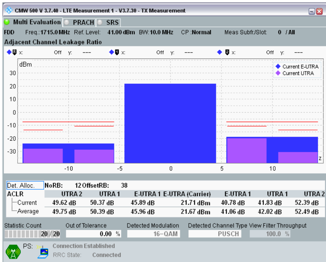
Band3 QAM16 BW=10MHz Channel=19250 RB Size=50 Position=#0
