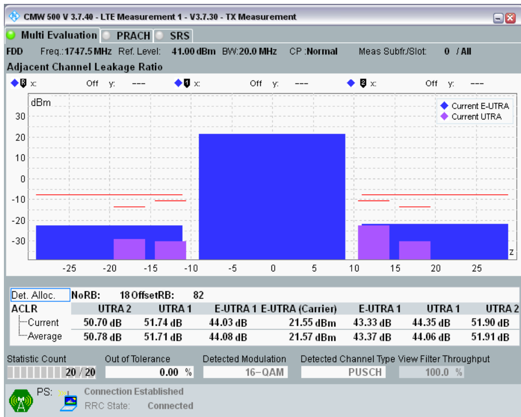
Band3 QAM16 BW=20MHz Channel=19575 RB Size=100 Position=#0
