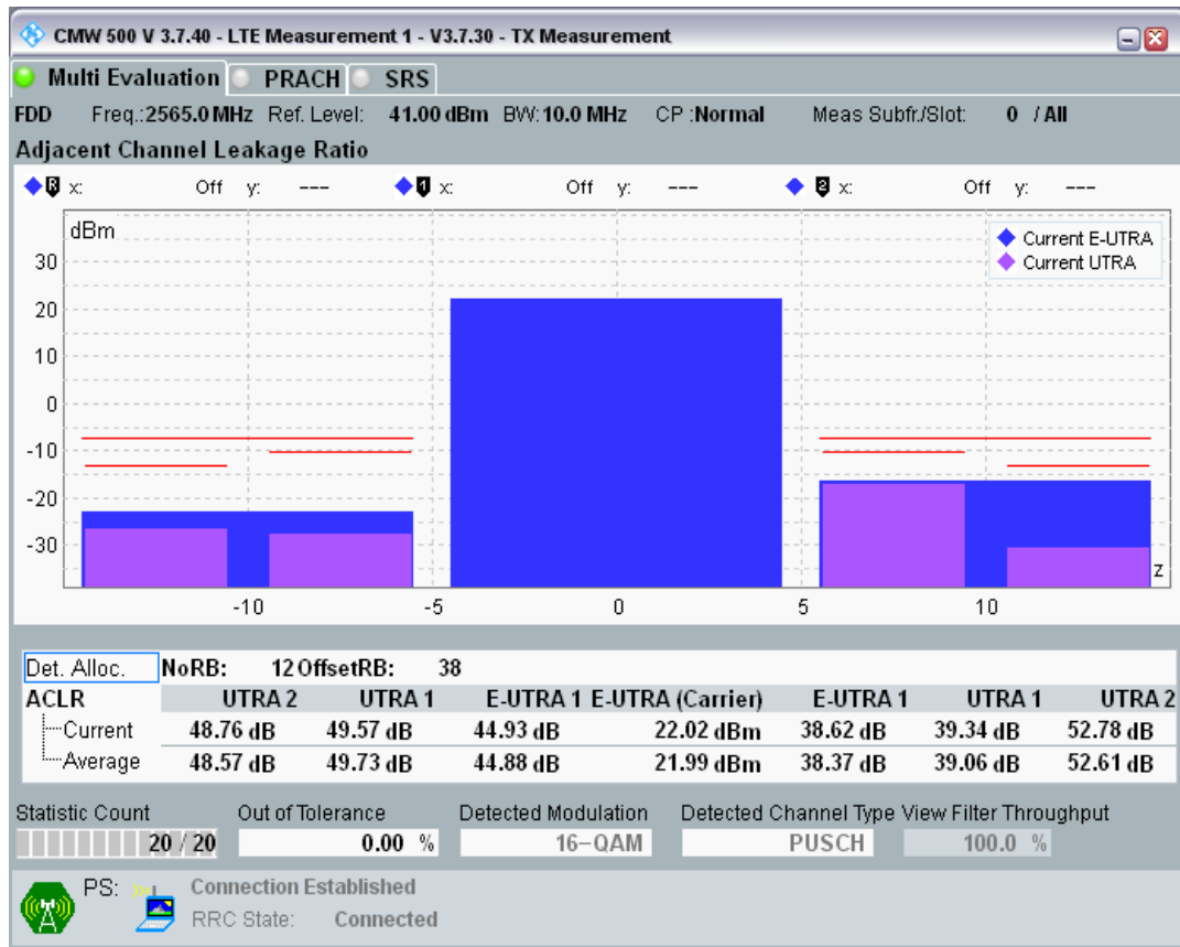
Band7 QAM16 BW=10MHz Channel=21400 RB Size=50 Position=#0
