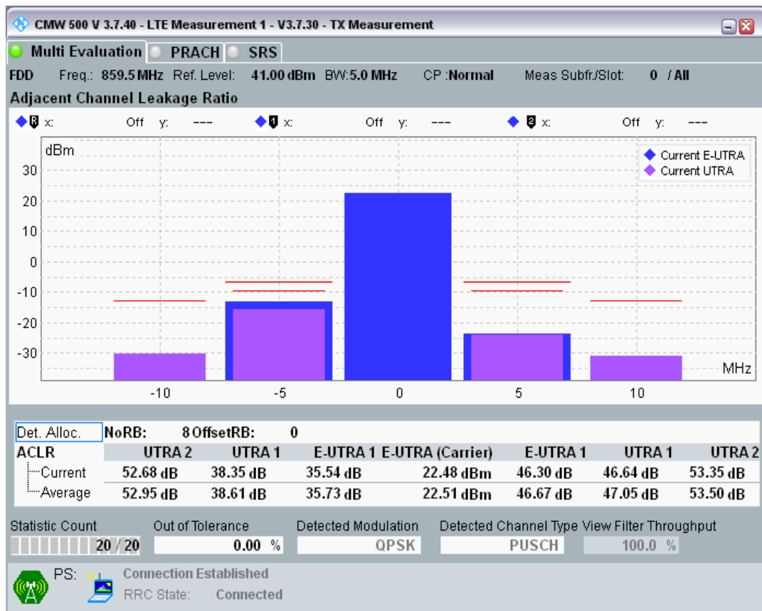
Band20 QPSK BW=5MHz Channel=24425 RB Size=8 Position=#Max
