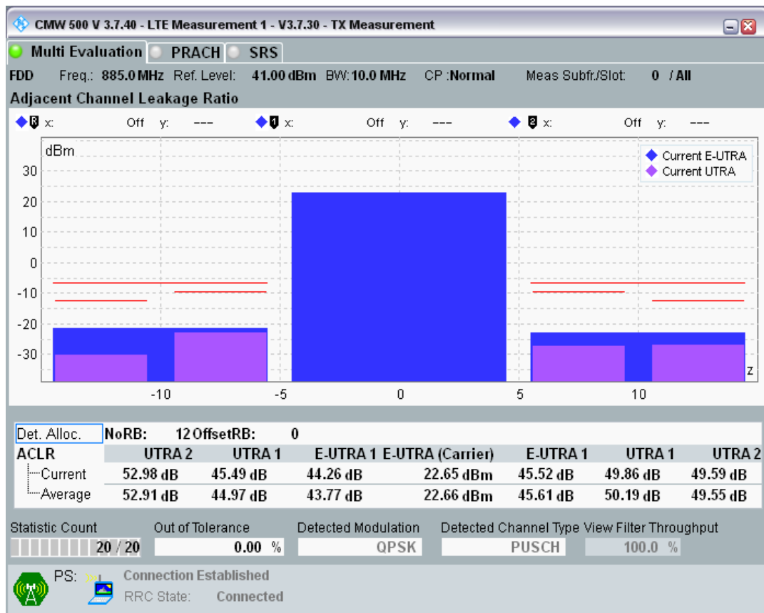
Band8 QPSK BW=10MHz Channel=21500 RB Size=12 Position=#Max
