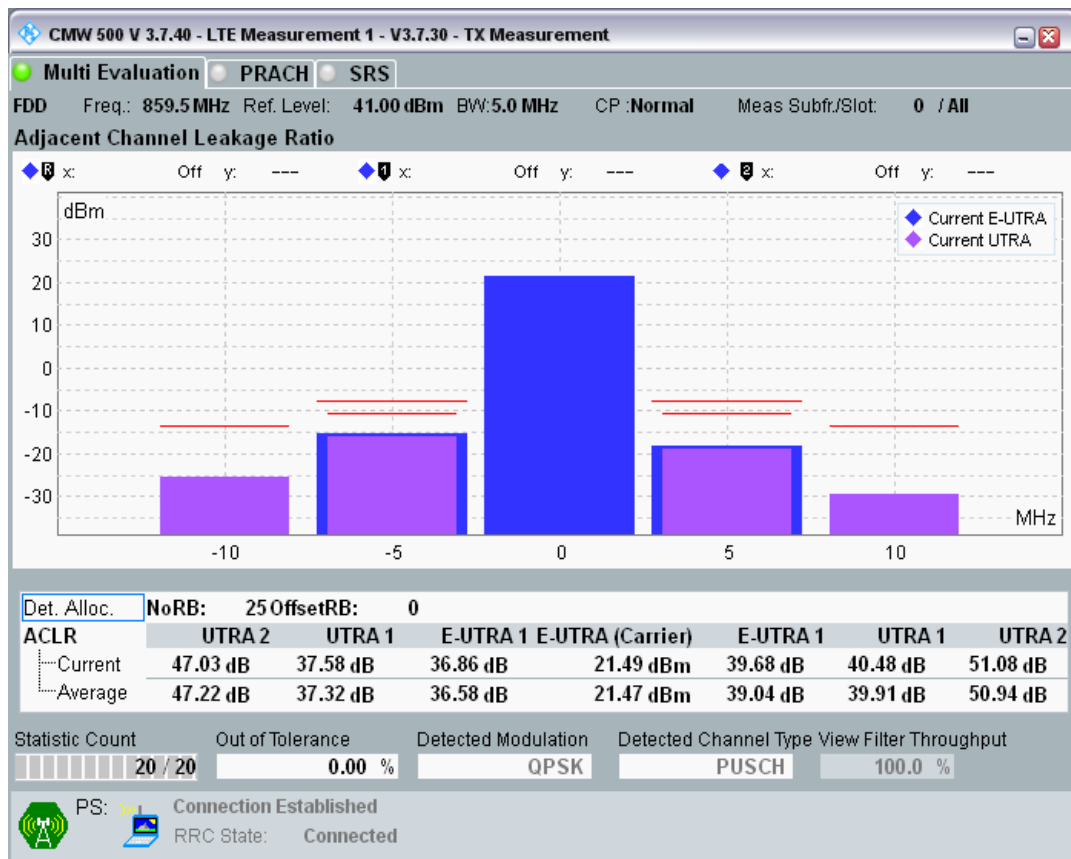
Band20 QAM16 BW=5MHz Channel=24425 RB Size=8 Position=#0
