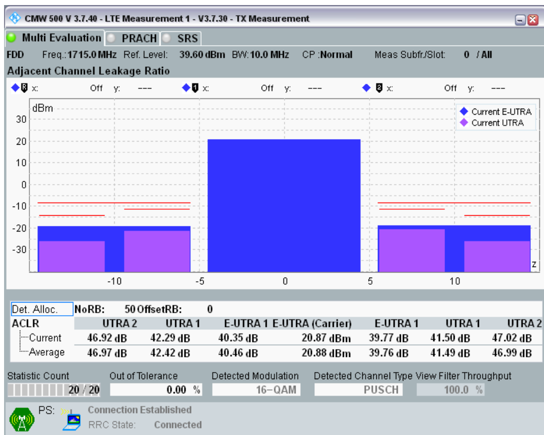
Band3 QPSK BW=10MHz Channel=19575 RB Size=12 Position=#0
