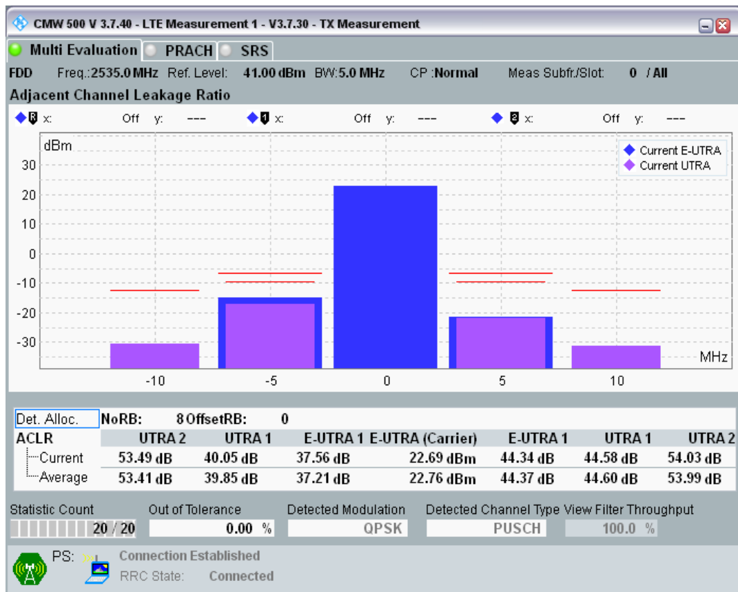
Band7 QPSK BW=5MHz Channel=21100 RB Size=8 Position=#Max
