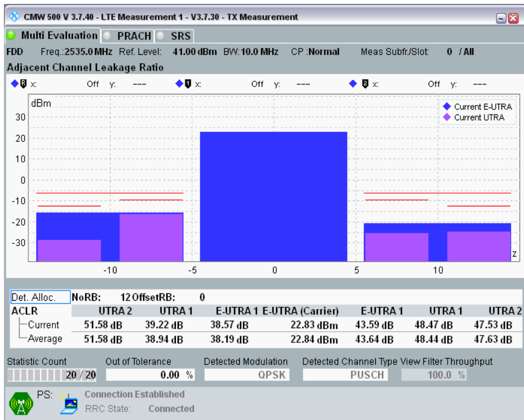
Band7 QPSK BW=10MHz Channel=21100 RB Size=12 Position=#Max
