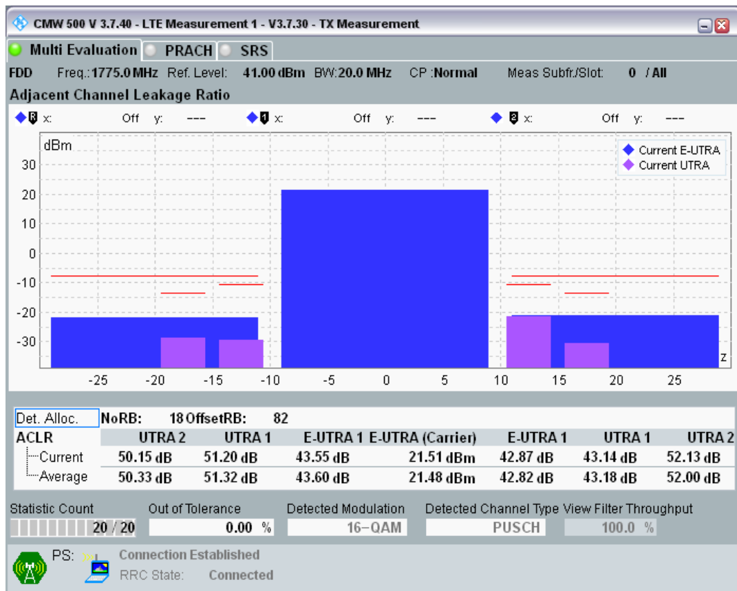
Band3 QAM16 BW=20MHz Channel=19850 RB Size=100 Position=#0
