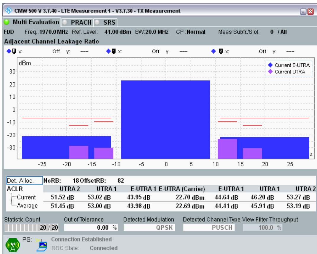
Band1 QPSK BW=20MHz Channel=18500 RB Size=100 Position=#0
