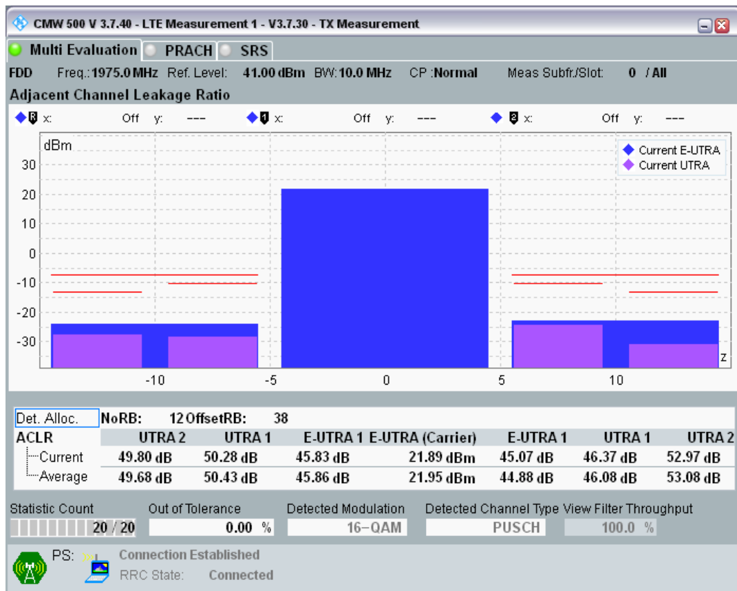
Band1 QAM16 BW=10MHz Channel=18550 RB Size=50 Position=#0
