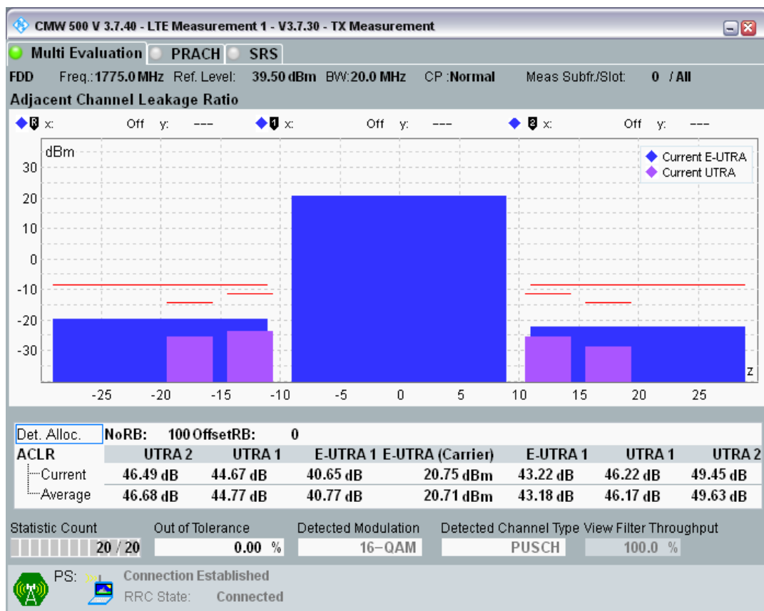
Band7 QPSK BW=5MHz Channel=20775 RB Size=8 Position=#0
