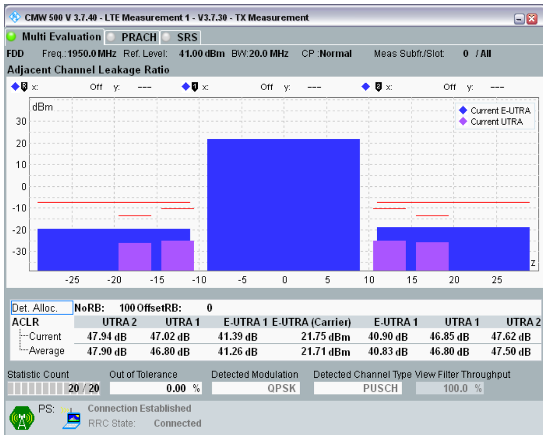
Band1 QAM16 BW=20MHz Channel=18300 RB Size=18 Position=#0
