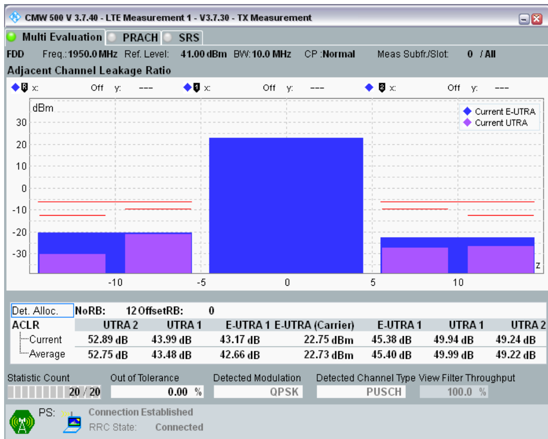
Band1 QPSK BW=10MHz Channel=18300 RB Size=12 Position=#Max
