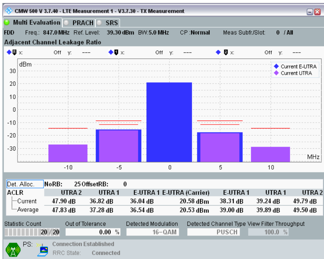
Band20 QPSK BW=5MHz Channel=24425 RB Size=8 Position=#0
