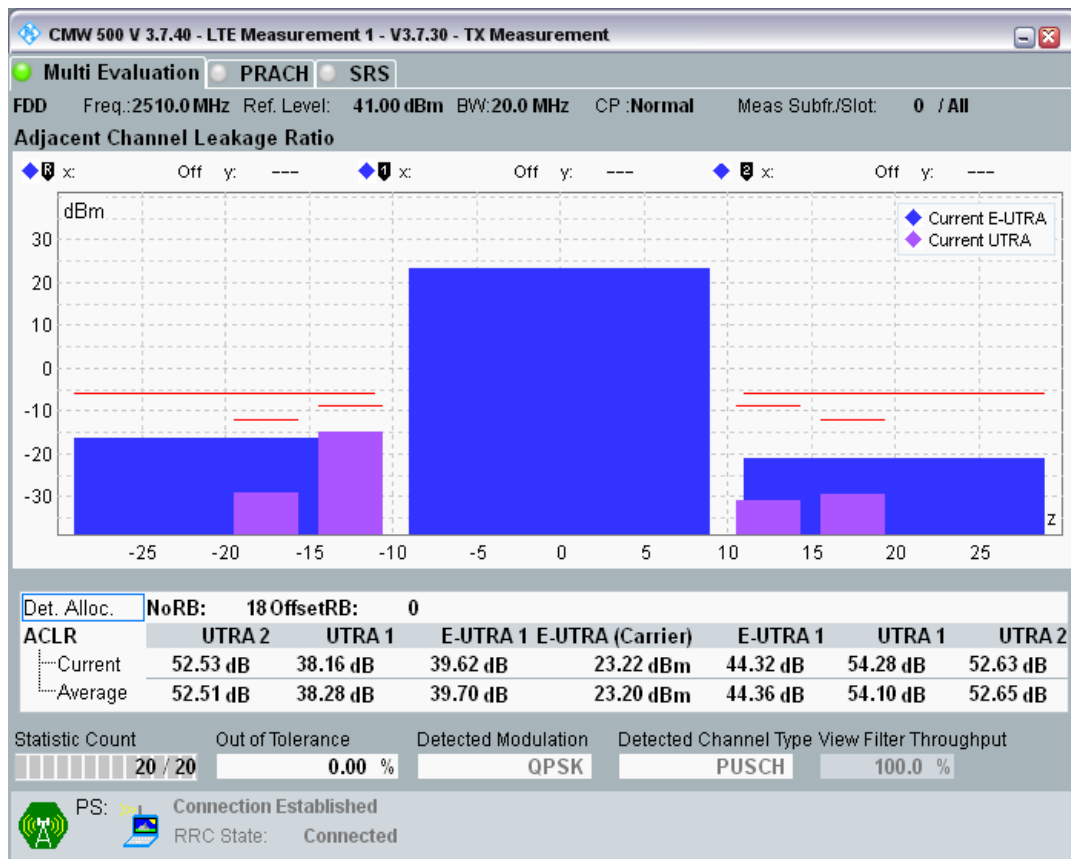
Band7 QPSK BW=20MHz Channel=20850 RB Size=18 Position=#Max
