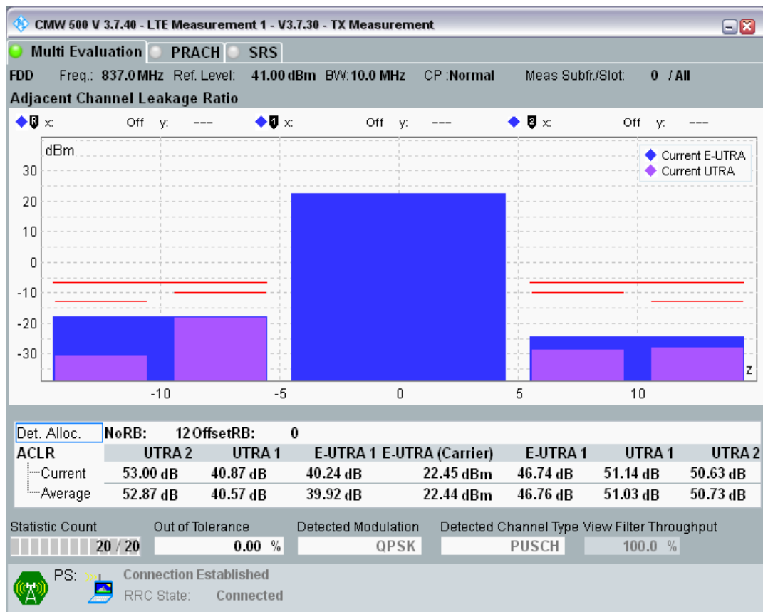
Band20 QPSK BW=10MHz Channel=24200 RB Size=12 Position=#Max
