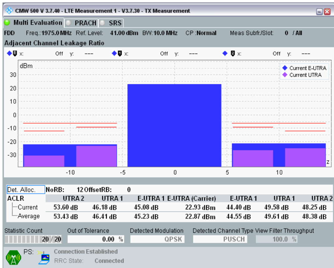
Band1 QPSK BW=10MHz Channel=18550 RB Size=12 Position=#Max
