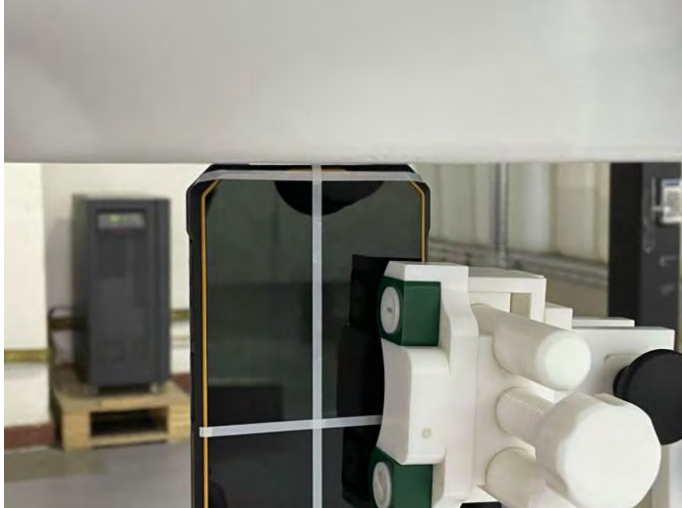
Back Side (Separation distance of 5mm)
