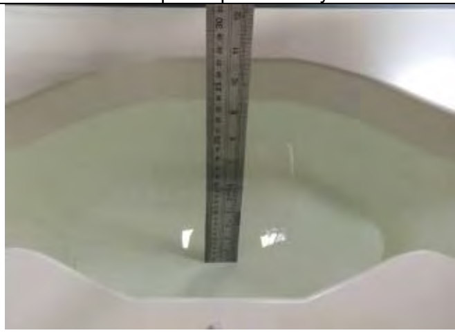
Photo of Liquid depth for Body Position
