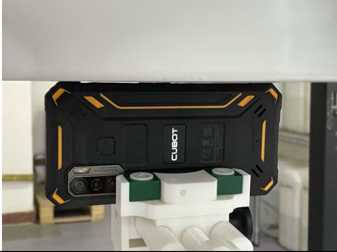
Top Side (Separation distance of 0mm)
