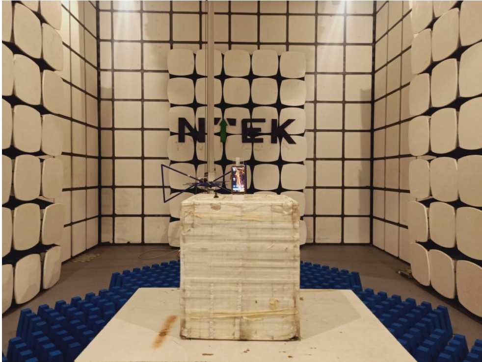
Radiated Spurious Emission Test
