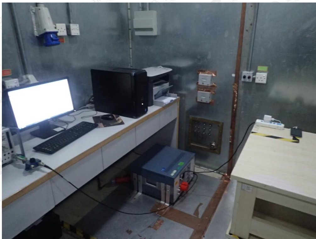
EN 55032 RADIATED EMISSION TEST SETUP
