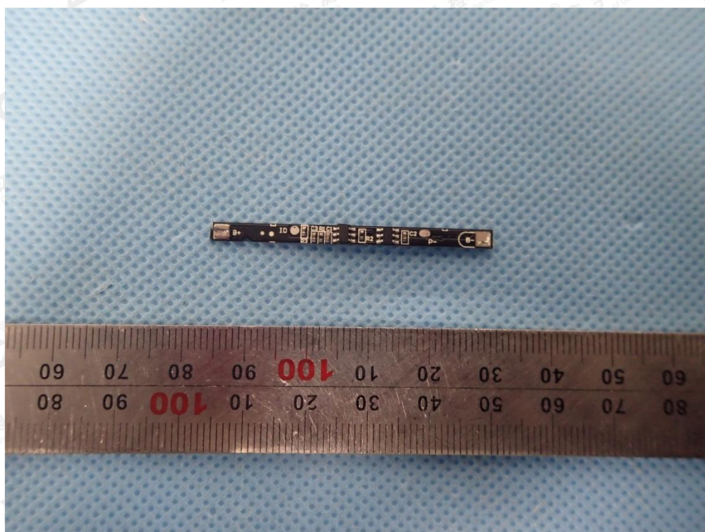
Fig.12 – top circuit of battery
