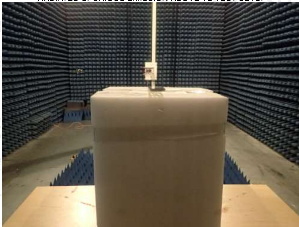
RADIATED SPURIOUS EMISSION-ABOVE 1G TEST SETUP
