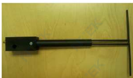
Figure 1 – MVG COMOSAR Validation Dipole
