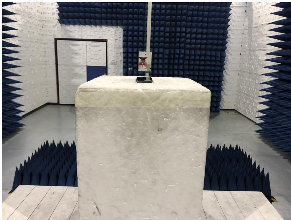
RADIATED EMISSION TEST SETUP ABOVE 1GHZ
