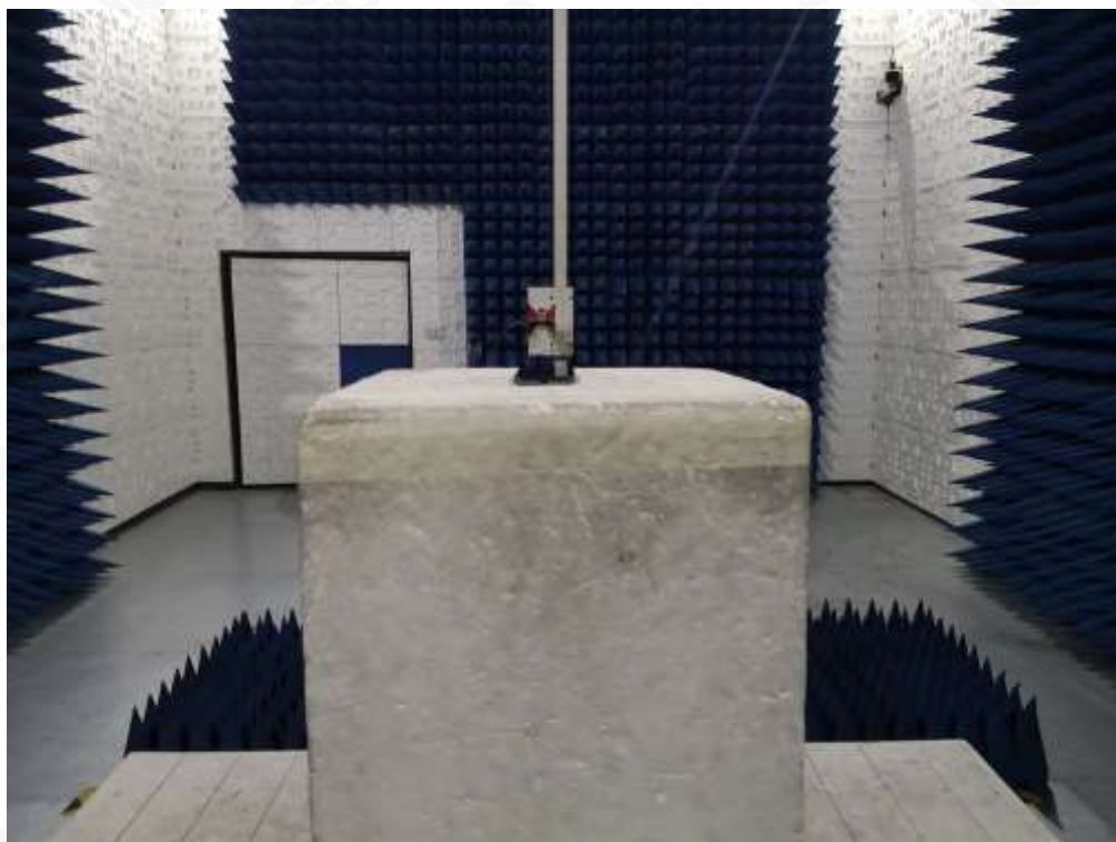
RADIATED SPURIOUS EMISSION-ABOVE 1G TEST SETUP
