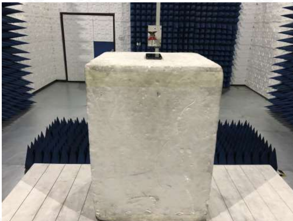
RADIATED SPURIOUS EMISSION-ABOVE 1G TEST SETUP
