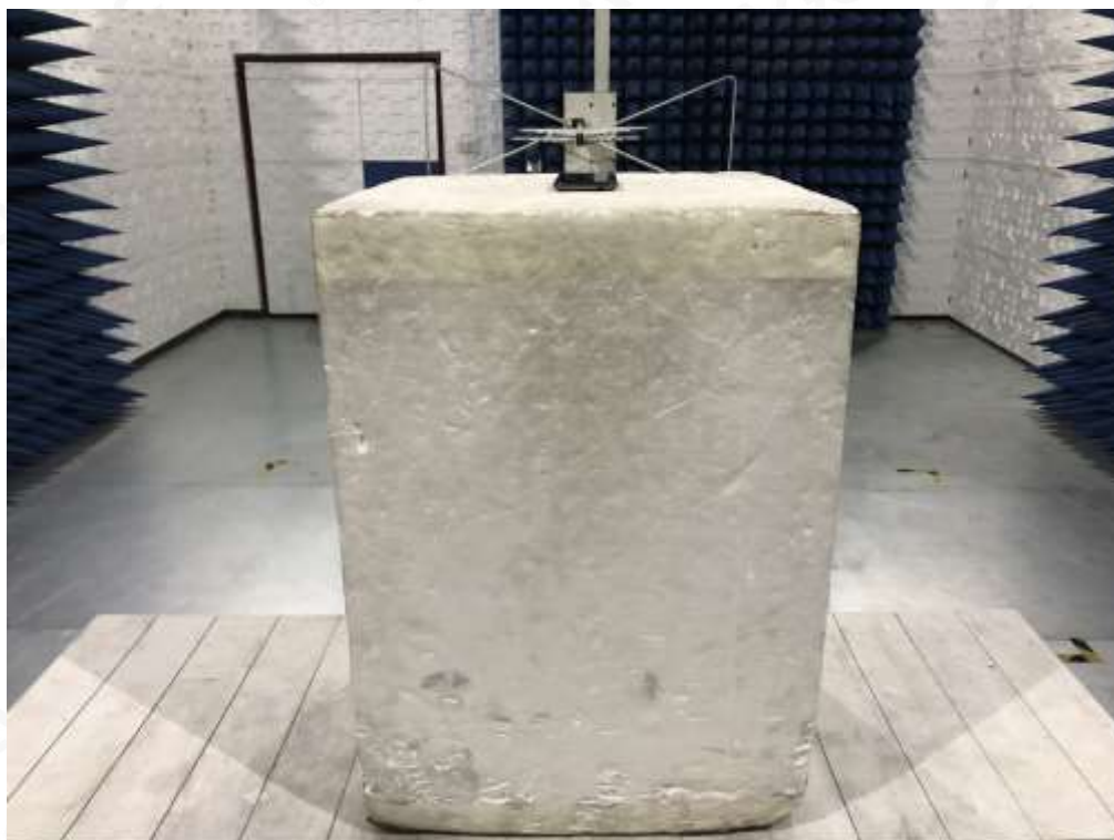
RADIATED SPURIOUS EMISSION-ABOVE 1G TEST SETUP
