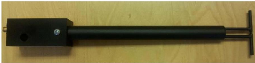
Figure 1 – MVG COMOSAR Validation Dipole
