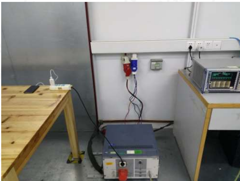
RADIATED EMISSION TEST SETUP
