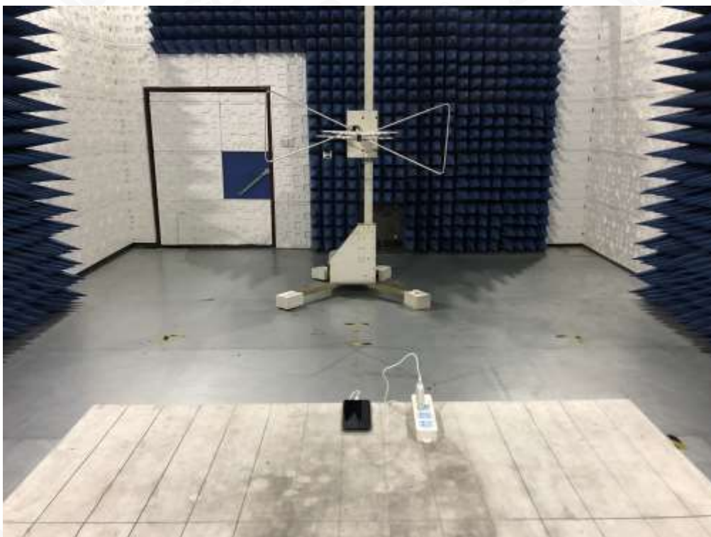
RADIATED EMISSION TEST SETUP
