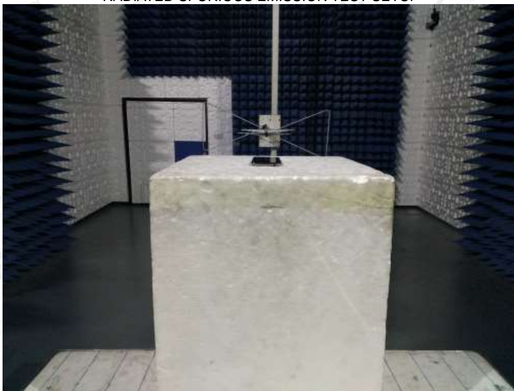
RADIATED SPURIOUS EMISSION-ABOVE 1G TEST SETUP
