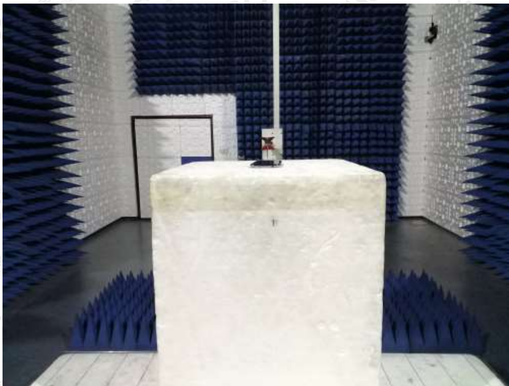
RADIATED SPURIOUS EMISSION-ABOVE 1G TEST SETUP
