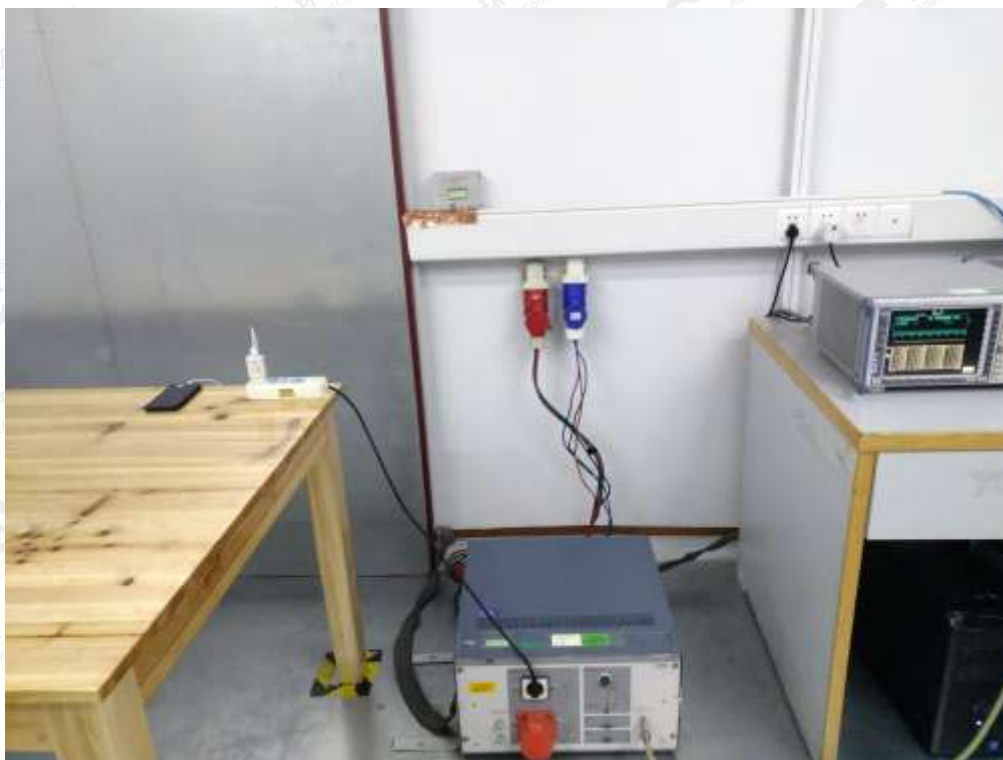
EN 55032 RADIATED EMISSION TEST SETUP
