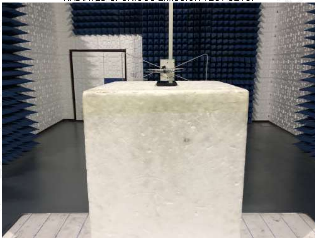
RADIATED SPURIOUS EMISSION-ABOVE 1G TEST SETUP
