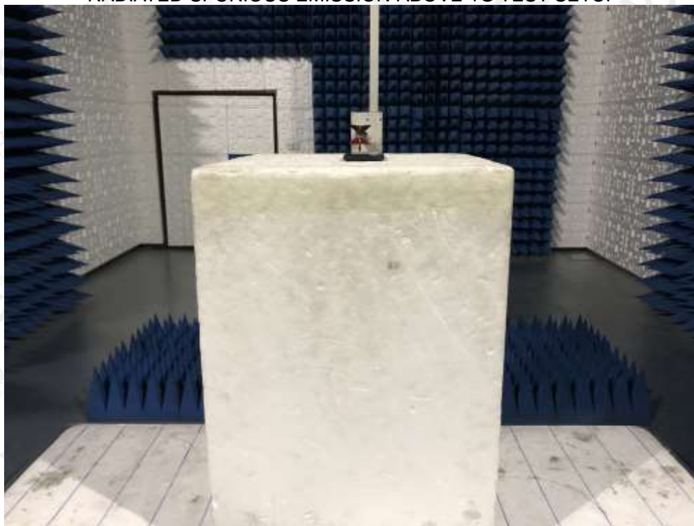
RADIATED SPURIOUS EMISSION-ABOVE 1G TEST SETUP
