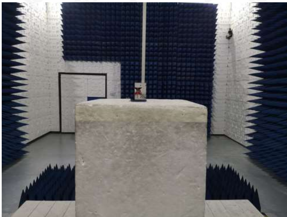
RADIATED SPURIOUS EMISSION-ABOVE 1G TEST SETUP
