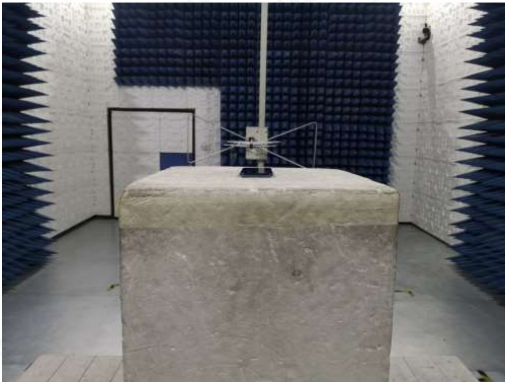
RADIATED SPURIOUS ABOVE 1G EMISSION TEST
