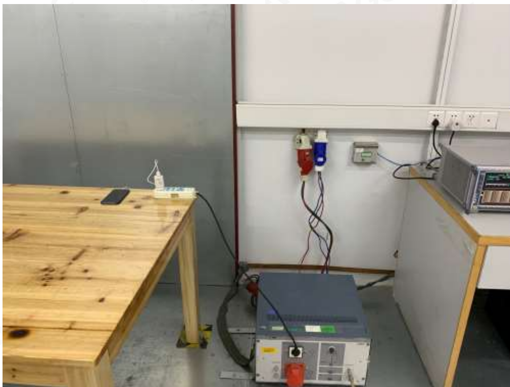
RADIATED EMISSION TEST SETUP
