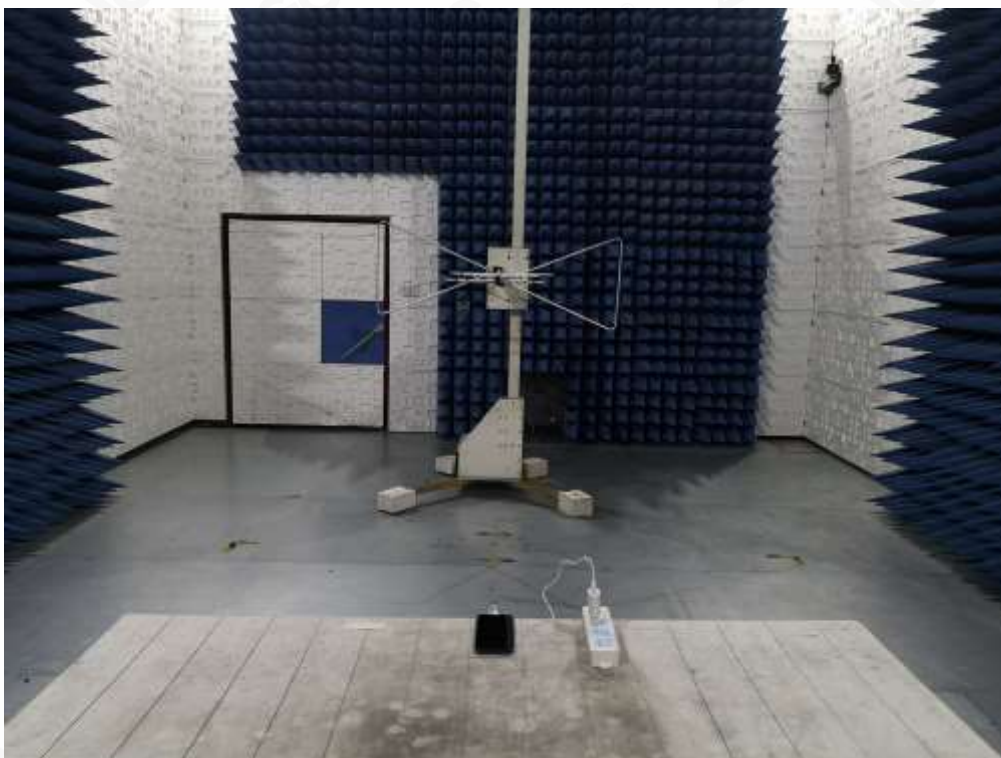
EN 55032 RADIATED EMISSION TEST SETUP
