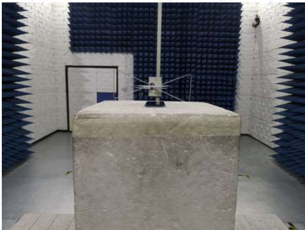
RADIATED SPURIOUS EMISSION ABOVE 1G TEST SETUP
