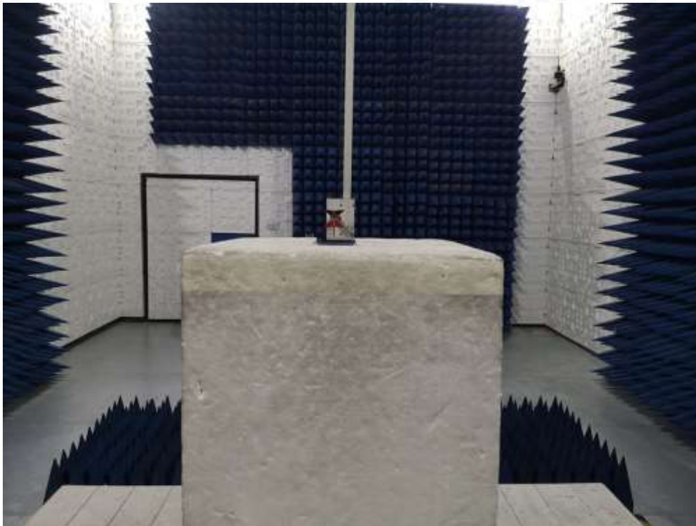
RADIATED SPURIOUS ABOVE 1G EMISSION TEST
