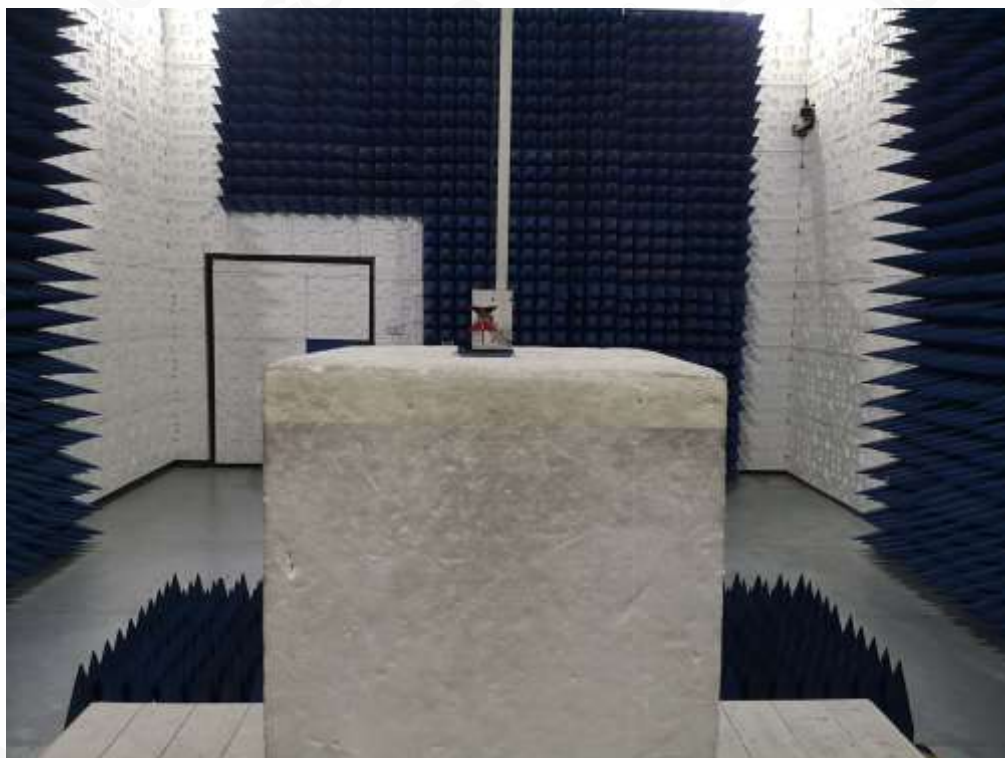
RADIATED SPURIOUS EMISSION ABOVE 1G TEST SETUP
