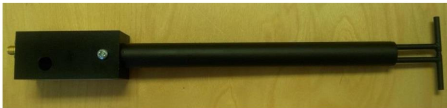
Figure 1 – MVG COMOSAR Validation Dipole
