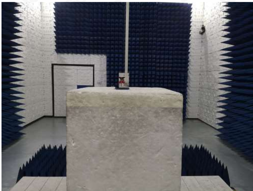
RADIATED SPURIOUS EMISSION ABOVE 1G TEST SETUP
