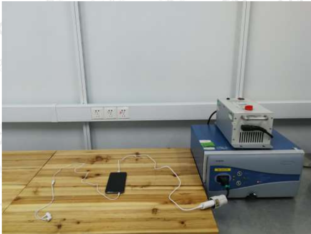
EFT SURGE and DIPS IMMUNITY TEST SETUP
