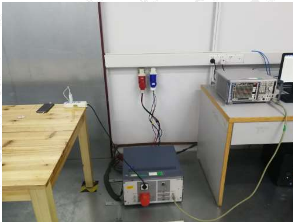
EN 55032 RADIATED EMISSION TEST SETUP
