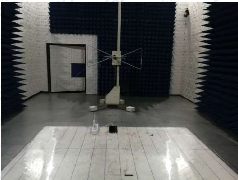
EN 55032 RADIATED EMISSION TEST SETUP
