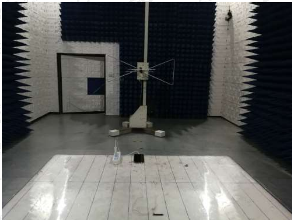
RADIATED EMISSION TEST SETUP
