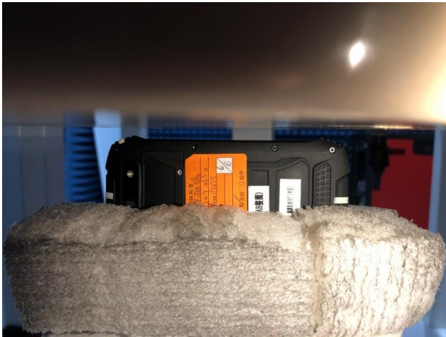
Body worn –Left (Test distance: 5mm, Thickness of DUT: 12mm)
