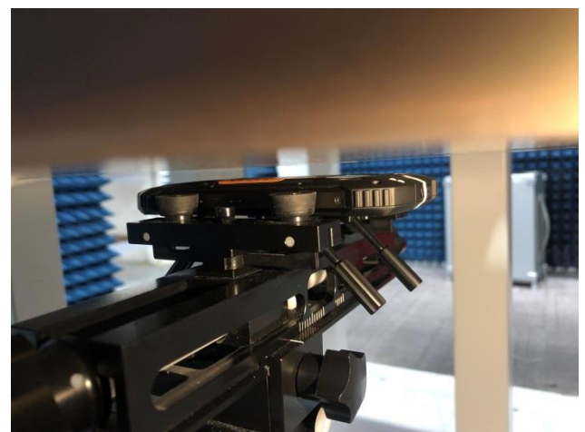
Body worn – Back (Test distance: 5mm, Thickness of DUT: 12mm)
