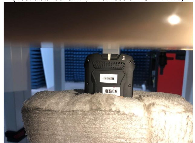
Body worn –Bottom (Test distance: 5mm, Thickness of DUT: 12mm)
