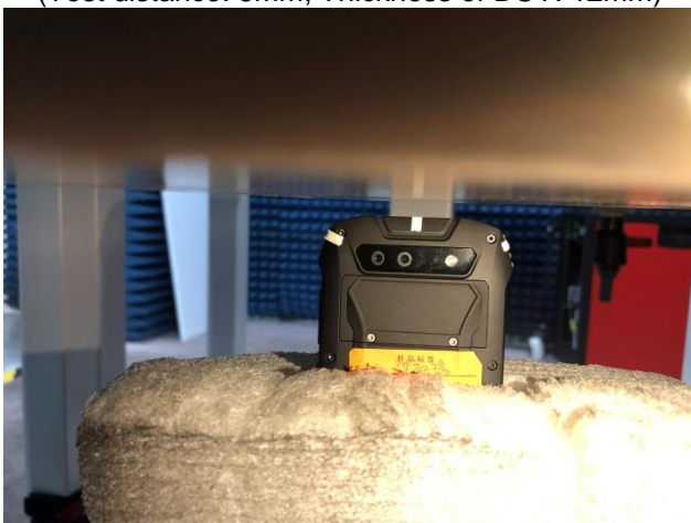
Body worn –Top (Test distance: 5mm, Thickness of DUT: 12mm)
