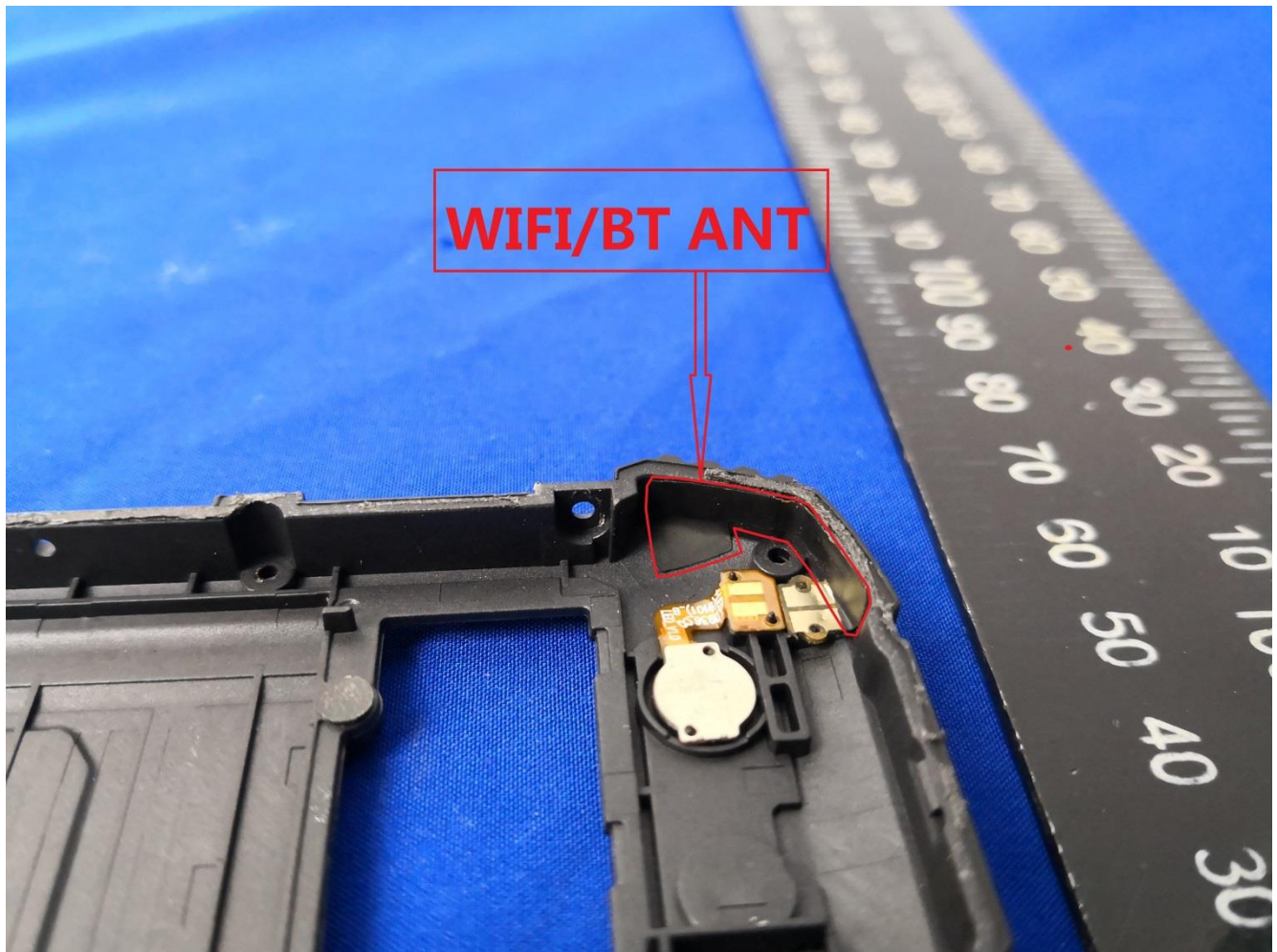
Fig.14.1 EUT Antenna Locations
