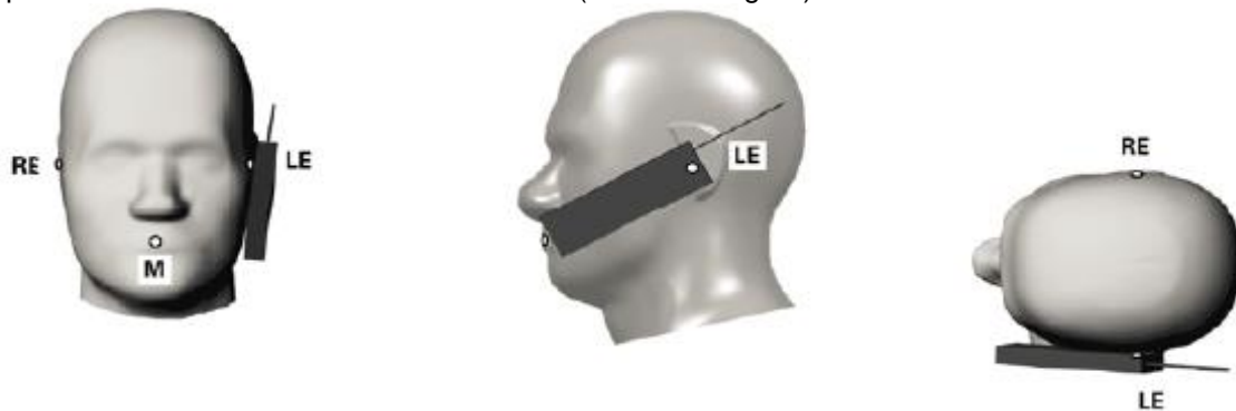
Fig. 11.3 Illustration for Cheek Position
