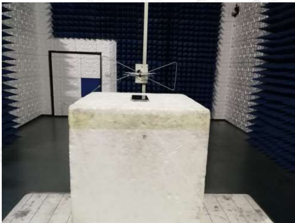
RADIATED SPURIOUS EMISSION-ABOVE 1G TEST SETUP
