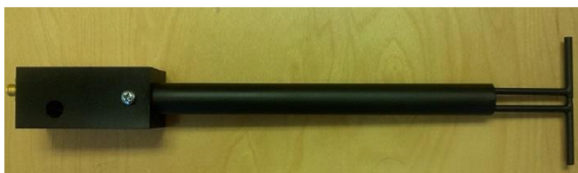
Figure 1 – MVG COMOSAR Validation Dipole
