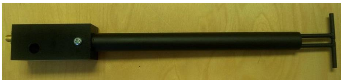
Figure 1 – MVG COMOSAR Validation Dipole
